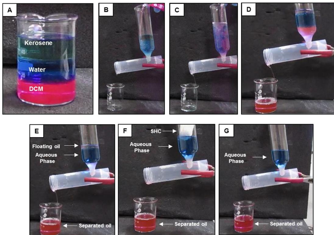
**Figure S11.** A) Digital image of three phases oil/water mixture that is consisted of kerosene (at top), aqueous phase (at middle) and DCM (model heavy oil, at bottom). B-E) Digital images illustrating the oil/water separation by the gravity driven filtration process, and small fraction of floating oil was finally removed based on absorption process. Pieces of SHC were strategically exploited during complimentary use of both the filtration and absorption processes.
