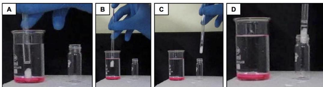
**Figure S8.** A-D) Digital images illustrating the inability of native cotton in collecting the sediment oil under DI water.
