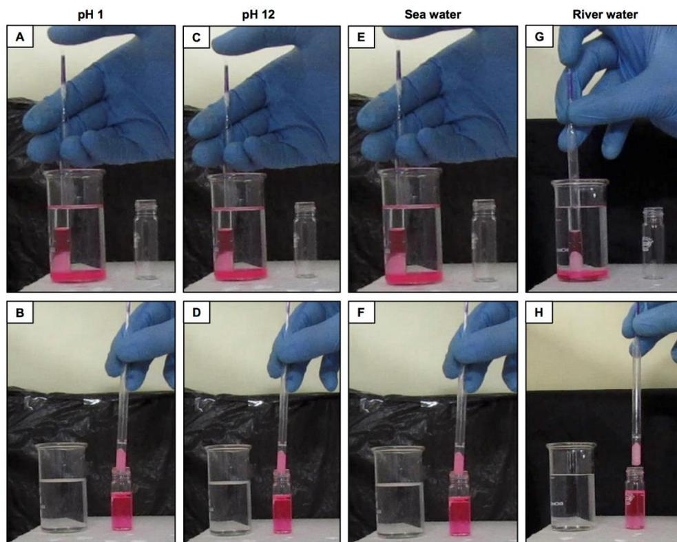
**Figure S7.** (A-H) Digital images illustrating the collection of sediment oil by filtration through SHC—but against the gravity under various complex aqueous phases including highly acidic medium of pH 1 (A, B), highly alkaline medium of pH 12 (C, D), artificial sea water (E, F) and river (Brahmaputra Assam India) water (G, H).
