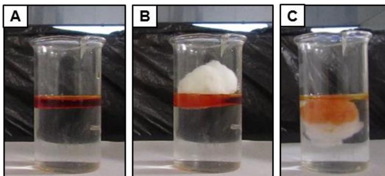
Figure S5. A-C) Digital images illustrating the performance of native cotton in removing the layered motor oils that were floating on aqueous phases.
