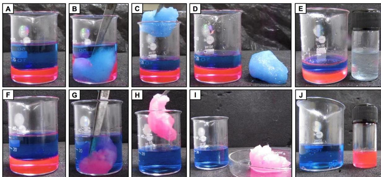
**Figure S6.** (A-J) Digital images comparing the interaction of native cotton (A-E) and SHC (F-J) with heavy oil (DCM, red color) under water; SHC was noticed to be extremely efficient in separating oil under water and native cotton was completely incapable of removing oil that was settled under water.
