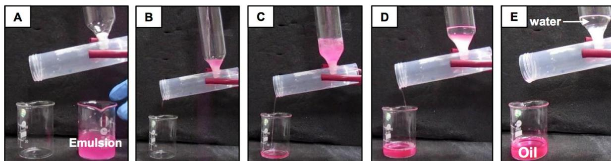
**Figure S12.** A-E) Digital images are revealing the ability of SHC in gravity driven filtration based emulsion (5 mL of water in 20 mL of DCM) separation.
