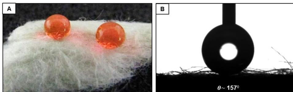
**Figure S10.** A-B) Digital image (A) and contact angle image (B) of beaded water droplet on SHC after successive (100 times) use in oil/water separation.
