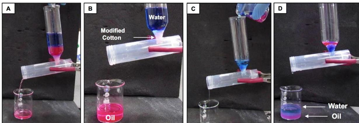
**Figure S9.** A-D) Digital images are illustrating the ability of both SHC (A-B) and the native cotton (C-D) in the gravity driven separation of oil/water mixture (20 mL DCM and 20 mL of water).
