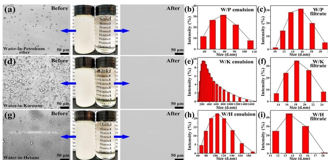
**Fig. S2** Microscope images, digital photos and droplet size distribution of the separation results for (a-c) Span 80 stabilized water-in-petroleum ether (W/P), (d-f) water-in-kerosene (W/K) and (g-i) water-in-hexane (W/H) emulsion.
