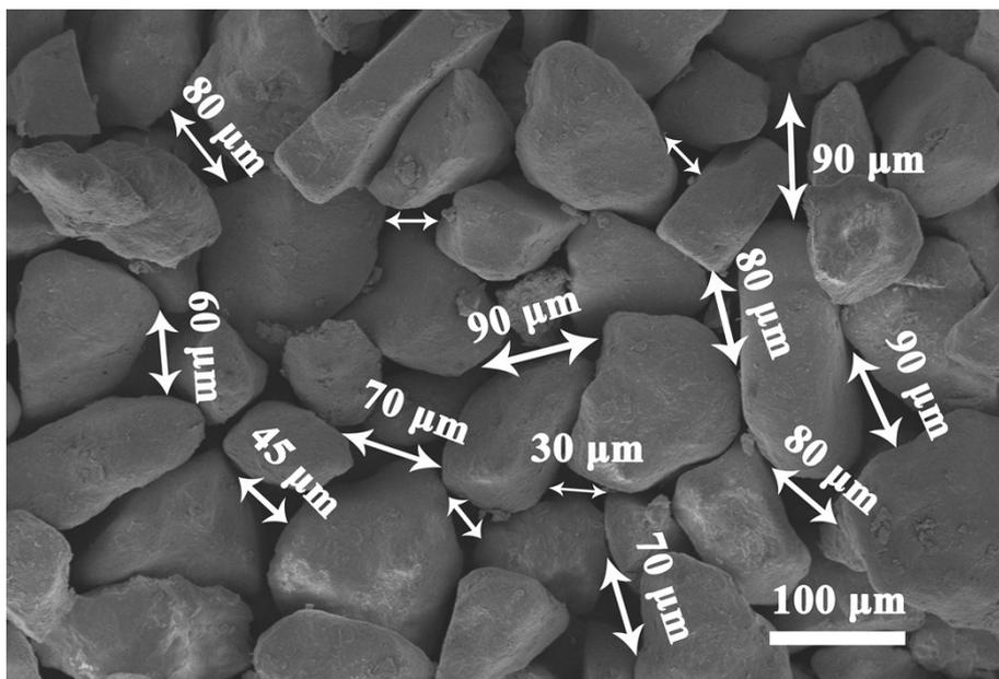
**Fig. S1** FE-SEM images of the sand layer for observation of pore size between sand particles.
