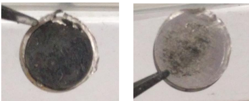
Figure S21. Photographs of Li anodes of S cath ( left ) and S-PAQ cath ( right ) cells showing the side of Li facing the separator.
