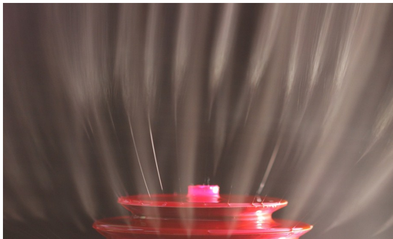
Fig. S1 Mass production of PAN nanofiber through Free-surface electrospinning
