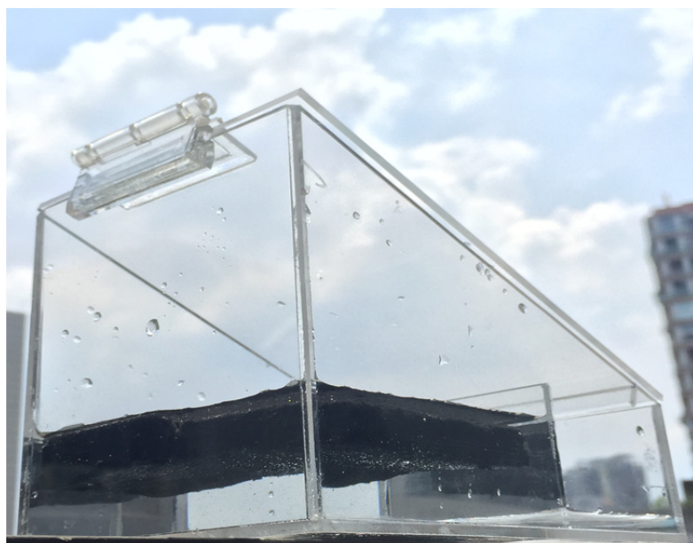
Fig. S20 The photograph of the homemade device for desalination under the natural sunlight.
