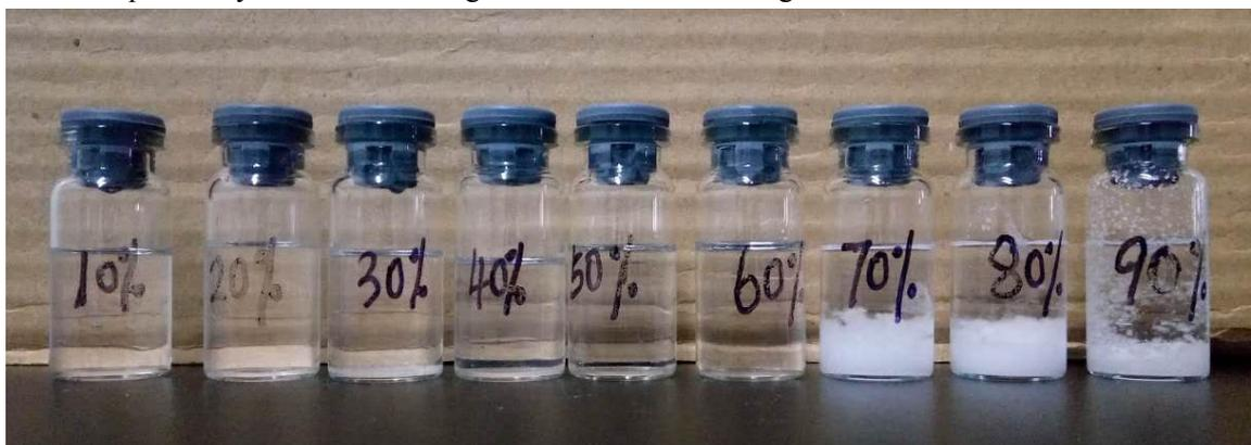
Fig. S7 Photograph of different pseudo concentrated electrolytes standing for 12 hours. Some lithium salt will be precipitated when the content of HFME is too high. Owing to the anti-solvent
