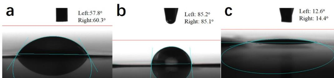
Fig. S5 Contact angle measurements of the electrolyte on the Celgard 2320 separator. (a) DE-LiFSI, (b) CE-LiFSI and (c) PCE-LiFSI.
