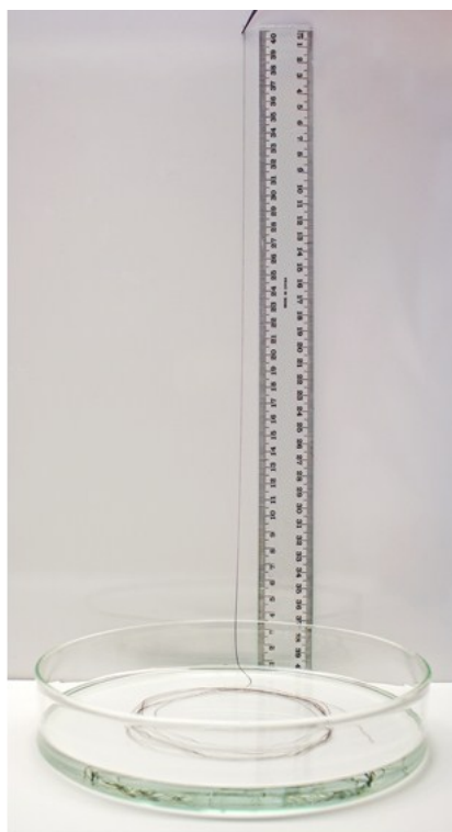
Fig. S2 Digital photograph of a wet-spun MXene/GO fiber (MXene ~88 wt.%). The hybrid fiber could be easily taken out of the coagulation bath without breaking.
