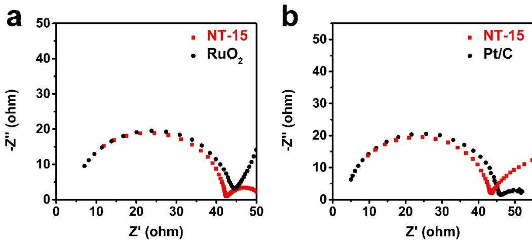
**Figure S3.** (a) Nyquist plots of NT-15 and RuO<sub>2</sub>; (b) Nyquist plots of NT-15 and Pt/C.
