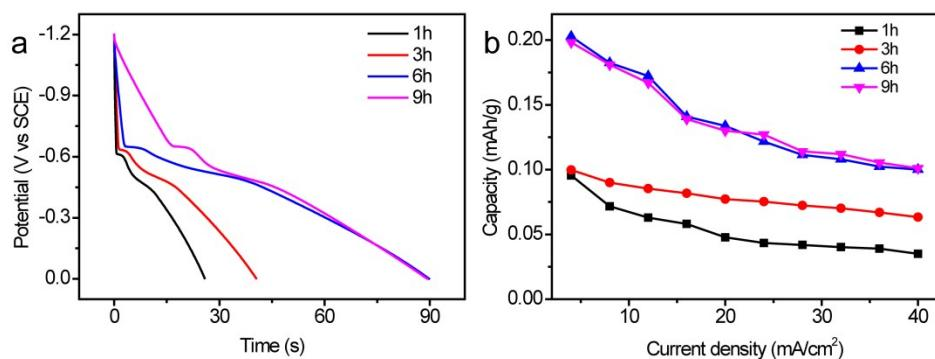
**Figure S8.** (a) Galvanostatic discharge curves at 16 mA/cm<sup>2</sup>, and (b) Capacity as a function of the H- $\text{Bi}_2\text{O}_3$  electrodes obtained at different annealing times.
