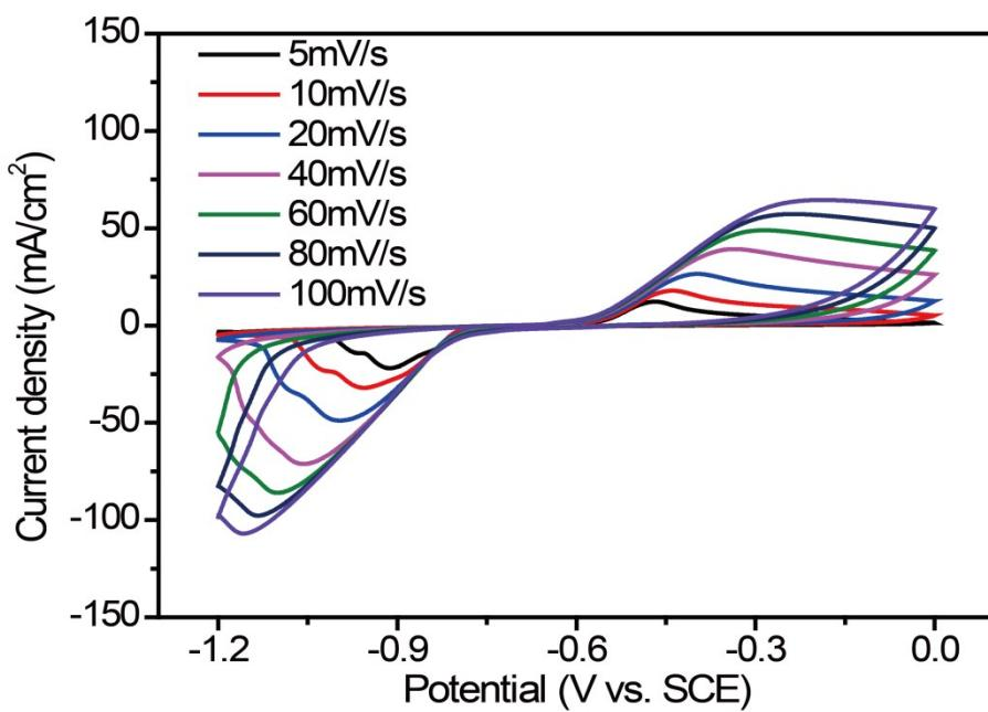
**Figure S4.** CV curves at various scan rates of H-Bi<sub>2</sub>O<sub>3</sub> samples
