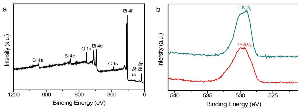
**Figure S3.** (a) Survey XPS spectrum of  $\text{Bi}_2\text{O}_3$  samples. (b) O 1s XPS spectra of the L- $\text{Bi}_2\text{O}_3$  and H- $\text{Bi}_2\text{O}_3$  samples.
