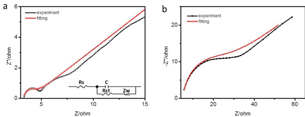
**Figure S6.** (a) EIS plots for H- $\text{Bi}_2\text{O}_3$  (black), and their corresponding simulation results (red). (b) for L- $\text{Bi}_2\text{O}_3$  and their simulation result.
