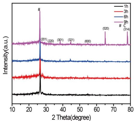
**Figure S7.** XRD spectra of the  $\text{Bi}_2\text{O}_3$  after different annealing time.
