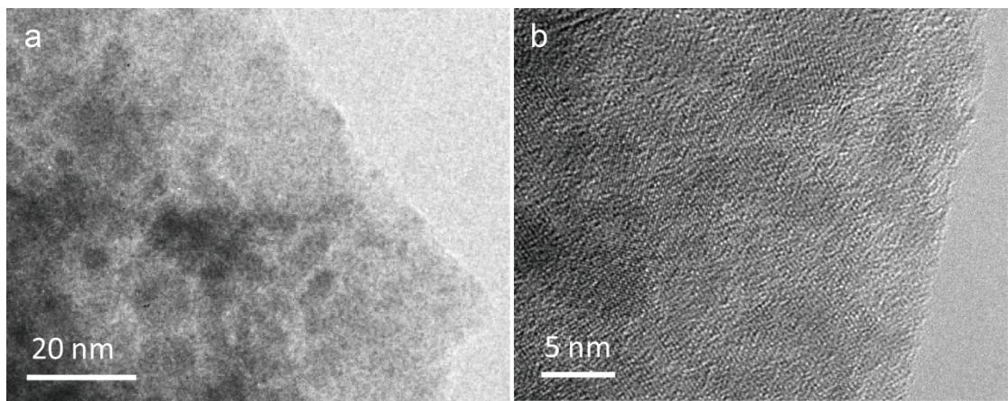
**Figure S2.** (a) TEM images of the L- $\text{Bi}_2\text{O}_3$ . (b) High-magnification TEM image of the L- $\text{Bi}_2\text{O}_3$ .
