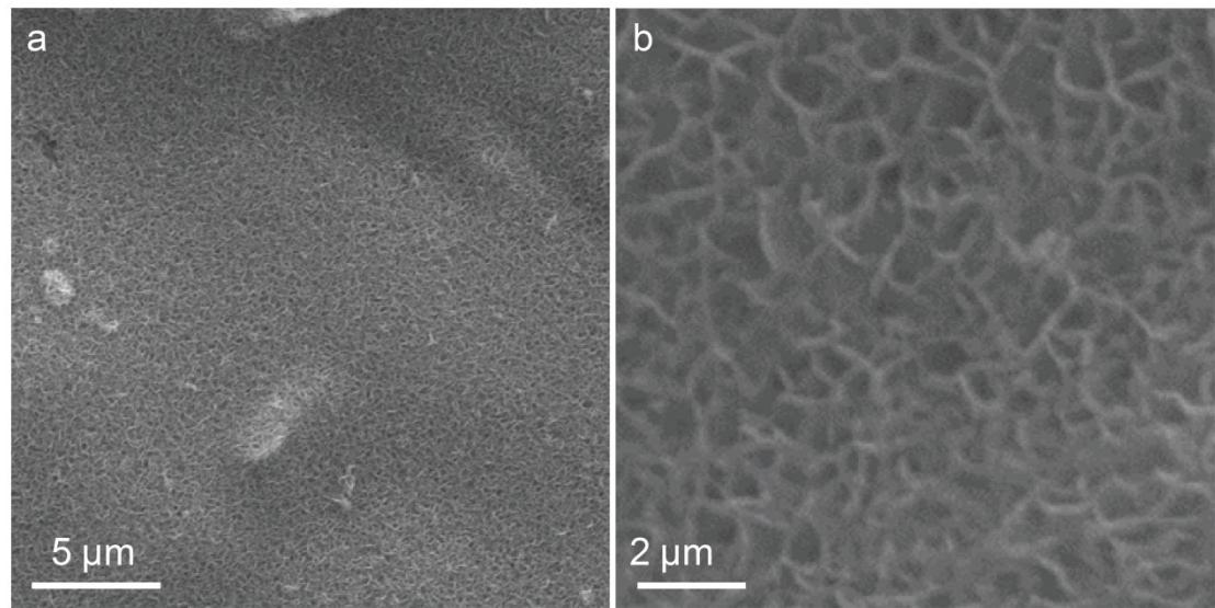
**Figure S1.** (a) SEM images of the L- $\text{Bi}_2\text{O}_3$ . (b) High-magnification SEM image of the L- $\text{Bi}_2\text{O}_3$ .
