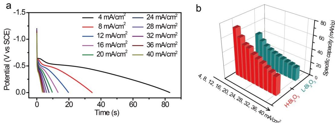
**Figure S5.** (a) Galvanostatic discharge curves of the L-Bi<sub>2</sub>O<sub>3</sub> electrodes at a different current densities. (b) Mass capacity of the L-Bi<sub>2</sub>O<sub>3</sub> and H-Bi<sub>2</sub>O<sub>3</sub> electrodes obtained from galvanostatic discharge curves.
