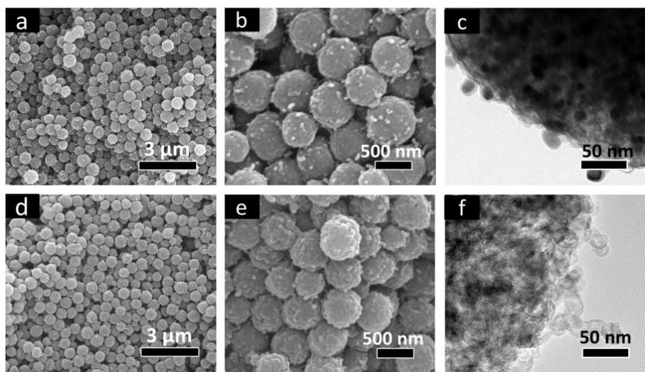
**Figure S2.** SEM and TEM images of metal carbide/carbon hybrid microspheres before (a-c) and after (d-f) acid etching.
