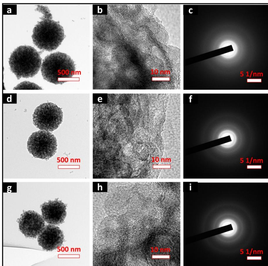
**Figure S5.** TEM, HRTEM and SAED patterns of PNC-600 (a-c), PNC-700 (d-f), and PNC-900 (g-i).
