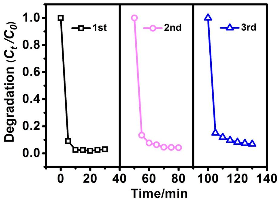
**Figure S10.** Stability and regeneration tests of PNC-800. Reaction conditions: [MB]=100 mg L<sup>-1</sup>, [Oxone]=1.0 g/L, catalyst=0.1 g L<sup>-1</sup>, T=25 °C, pH=6.30.
