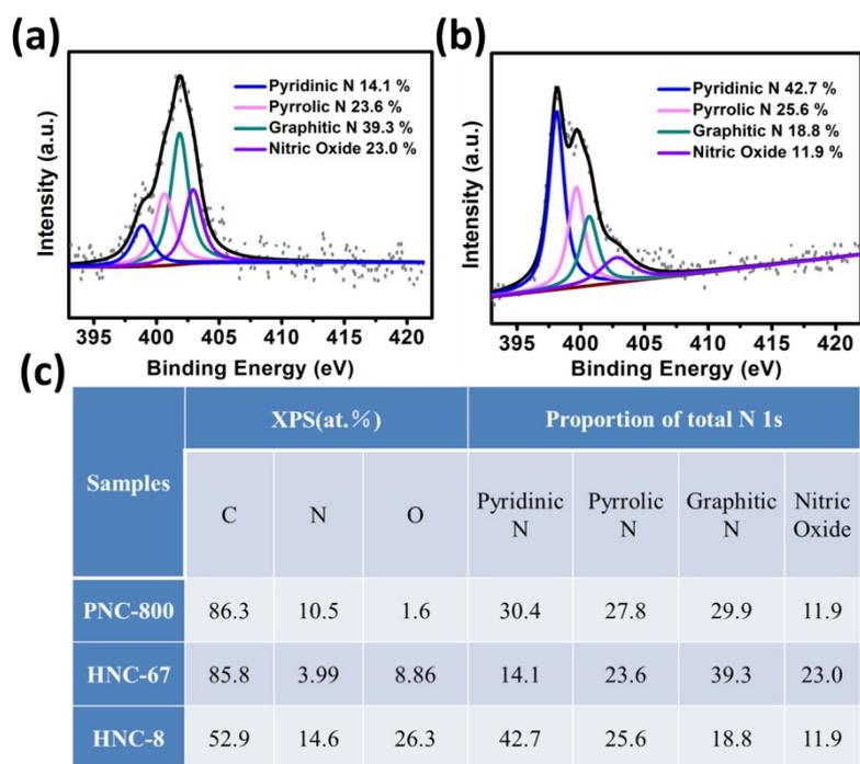
**Figure S7.** High-resolution N 1s XPS spectra of HNC-67 (a) and HNC-8 (b), and the parameters of XPS spectra and the fitting results of N 1s peaks of PNC-800, HNC-67 and HNC-8 (c).
