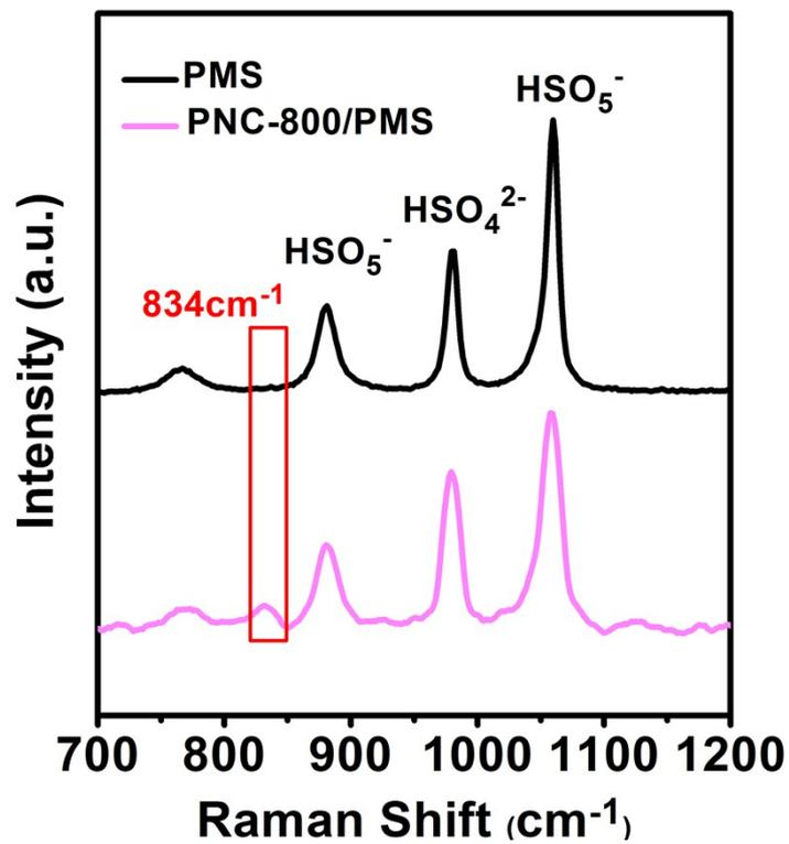
Figure S9. Raman spectra of PMS solution and PNC-800 in PMS solution.
