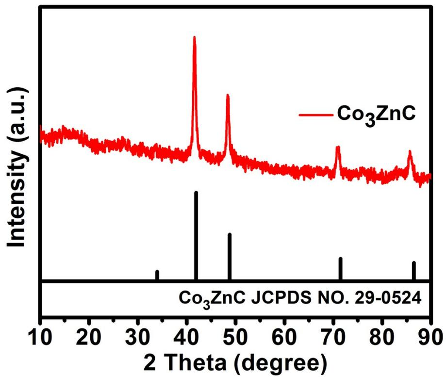
Figure S3. XRD pattern of metal carbide/carbon hybrid nanocomposite.
