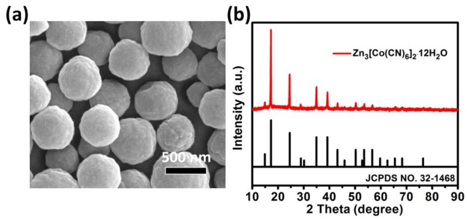
**Figure S1.** SEM and XRD pattern of  $\text{Zn}_3[\text{Co}(\text{CN})_6]_2 \cdot 12\text{H}_2\text{O}$  microspheres.
