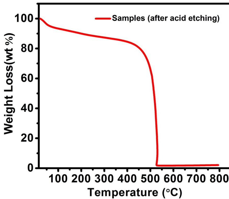
**Figure S4.** TG curve of metal carbide/carbon hybrid microspheres after acid etching under air atmosphere.
