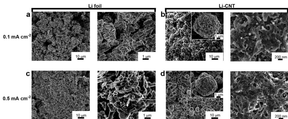
**Figure S8.** SEM images of (a) the Li foil electrodes and (b) the Li-CNT electrodes after 400 h cycling at  $0.1 \text{ mA cm}^{-2}$ . SEM images of (c) the Li foil electrodes and (d) the Li-CNT electrodes after 400 h cycling at  $0.5 \text{ mA cm}^{-2}$ .
