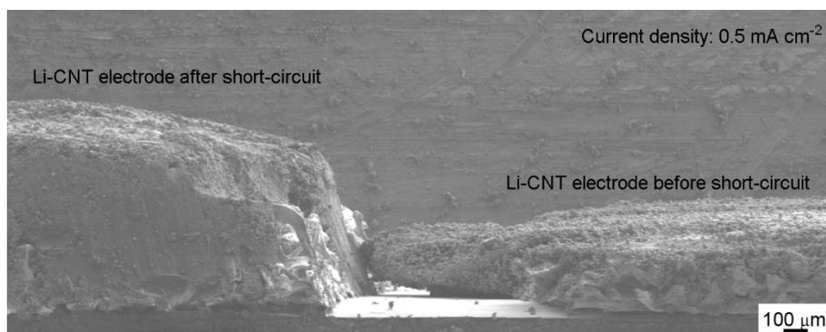
**Figure S5.** The cross section SEM images of the Li-CNT electrode before and after the short-circuit testing at a current density of  $0.5 \text{ mA cm}^{-2}$ .
