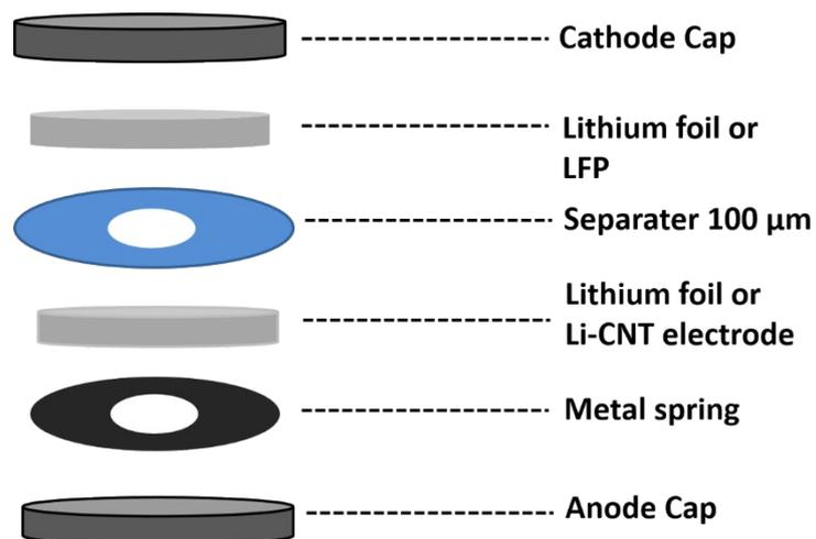
**Figure S4.** The configuration of the coin battery used for short-circuit time testing.
