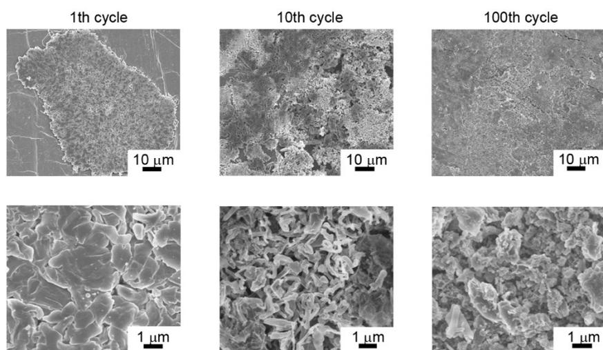
**Figure S6.** SEM images of the Li foil electrodes after different cycles at  $0.5 \text{ mA cm}^{-2}$ . The Li foil surface morphology evolution indicates that more and more dendrites grow on the electrode surface.
