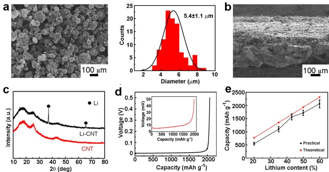
**Figure S3.** Characterization of the Li-CNT composite particles. (a) SEM micrographs and the diameter distribution histogram of the Li-CNT composite particles. (b) The cross-section SEM image of the Li-CNT electrode. (c) XRD patterns of the CNT particles (red line) and the Li-CNT composites particles (black line). (d) Galvanostatic discharge curve of the Li-CNT electrode. (e) The Li-CNT capacity vs. the lithium content in Li-CNT.
