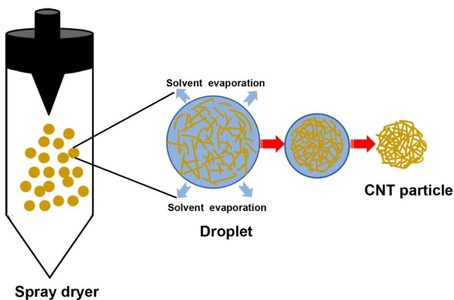
**Figure S1.** Schematic illustration of the spray dry preparation process of CNT particles.
