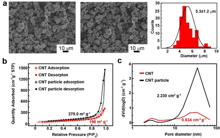
**Figure S2.** Characterization of the CNT particles. (a) SEM micrographs and the diameter distribution histogram of the CNT particles. (b) Argon adsorption/desorption isotherms of the pristine CNT and the CNT particles. (c) The pore-size distribution of pristine CNT and the CNT particles.
