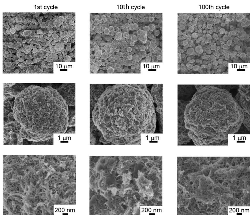
**Figure S7.** SEM images of the Li-CNT electrodes after different cycles at  $0.5 \text{ mA cm}^{-2}$ . The Li-CNT electrode shows almost no dendrite formation and the spherical structure remains.
