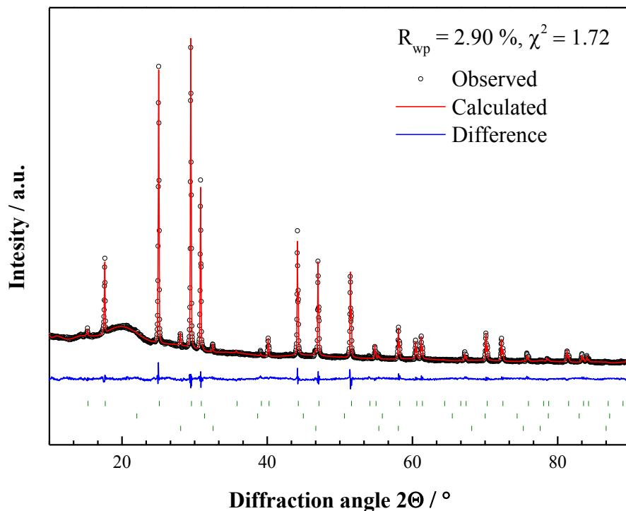
Figure S10. X-ray powder diffraction data for  $\text{Li}_{6.25}\text{P}_{0.75}\text{Si}_{0.25}\text{S}_5\text{Br}$  and the corresponding Rietveld refinements. Shown are the collected data, the profile fit, the profile residuals and the Bragg reflections for the main phase (top).
