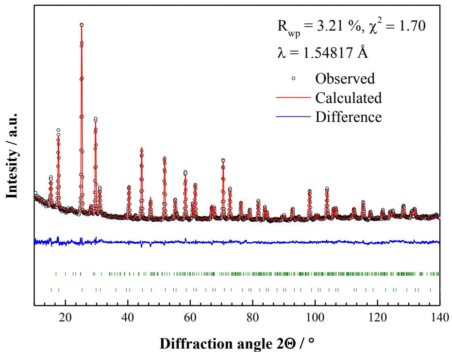
Figure S15. Neutron powder data for  $\text{Li}_{6.25}\text{P}_{0.75}\text{Si}_{0.25}\text{S}_5\text{Br}$  and the corresponding Rietveld refinements. Shown are the collected data, the profile fit, the profile residuals and the Bragg reflections for the main phase (top).
