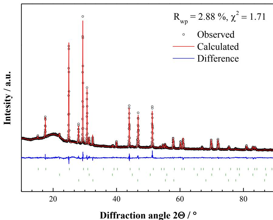
Figure S13. X-ray powder diffraction data for  $\text{Li}_{6.50}\text{P}_{0.50}\text{Si}_{0.50}\text{S}_5\text{Br}$  and the corresponding Rietveld refinements. Shown are the collected data, the profile fit, the profile residuals and the Bragg reflections for the main phase (top).
