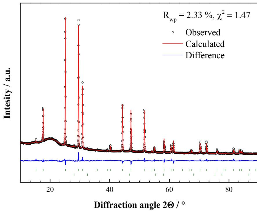
Figure S5. X-ray powder diffraction data for  $\text{Li}_{6.10}\text{P}_{0.90}\text{Si}_{0.10}\text{S}_5\text{Br}$  and the corresponding Rietveld refinements. Shown are the collected data, the profile fit, the profile residuals and the Bragg reflections for the main phase (top).
