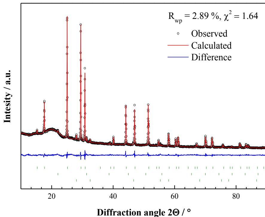
Figure S11. X-ray powder diffraction data for  $\text{Li}_{6.30}\text{P}_{0.70}\text{Si}_{0.30}\text{S}_5\text{Br}$  and the corresponding Rietveld refinements. Shown are the collected data, the profile fit, the profile residuals and the Bragg reflections for the main phase (top).
