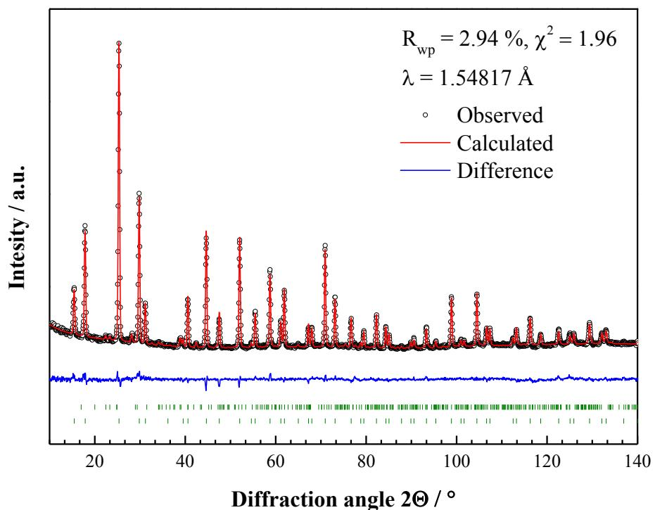
Figure S14. Neutron powder data for  $\text{Li}_6\text{PS}_5\text{Br}$  and the corresponding Rietveld refinements. Shown are the collected data, the profile fit, the profile residuals and the Bragg reflections for the main phase (top).
