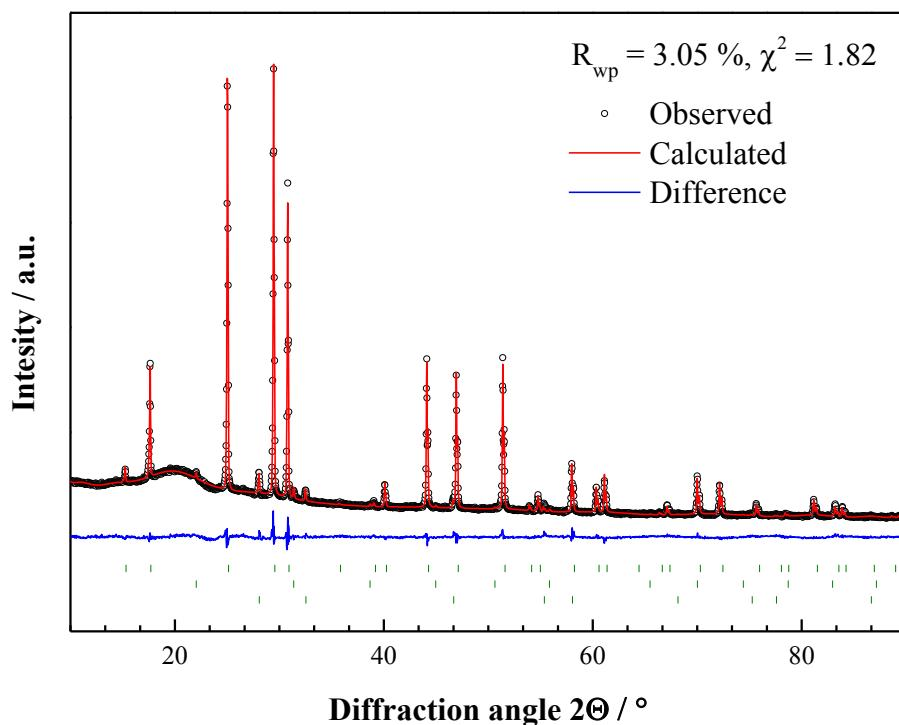
Figure S12. X-ray powder diffraction data for  $\text{Li}_{6.35}\text{P}_{0.65}\text{Si}_{0.35}\text{S}_5\text{Br}$  and the corresponding Rietveld refinements. Shown are the collected data, the profile fit, the profile residuals and the Bragg reflections for the main phase (top).
