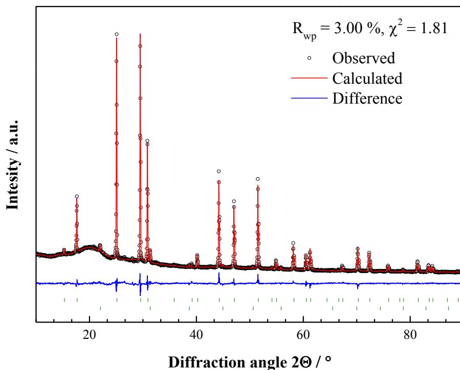
Figure S8. X-ray powder diffraction data for  $\text{Li}_{6.20}\text{P}_{0.80}\text{Si}_{0.20}\text{S}_5\text{Br}$  and the corresponding Rietveld refinements. Shown are the collected data, the profile fit, the profile residuals and the Bragg reflections for the main phase (top).
