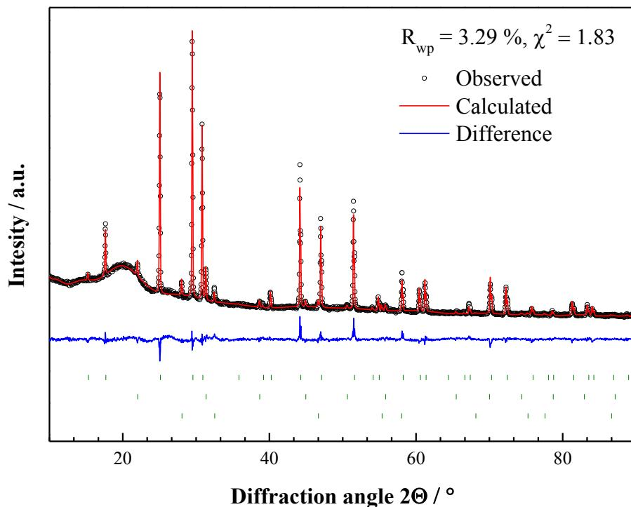
Figure S9. X-ray powder diffraction data for  $\text{Li}_{6.225}\text{P}_{0.775}\text{Si}_{0.225}\text{S}_5\text{Br}$  and the corresponding Rietveld refinements. Shown are the collected data, the profile fit, the profile residuals and the Bragg reflections for the main phase (top).
