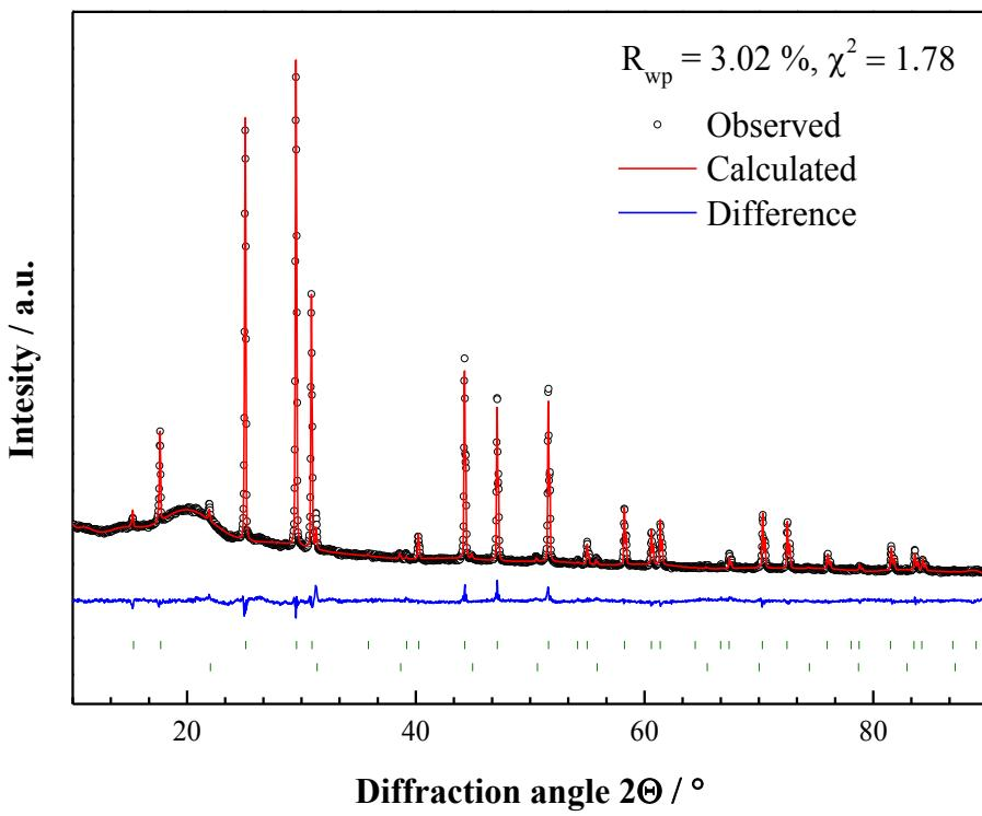
Figure S4. X-ray powder diffraction data for  $\text{Li}_{6.075}\text{P}_{0.925}\text{Si}_{0.075}\text{S}_5\text{Br}$  and the corresponding Rietveld refinements. Shown are the collected data, the profile fit, the profile residuals and the Bragg reflections for the main phase (top).
