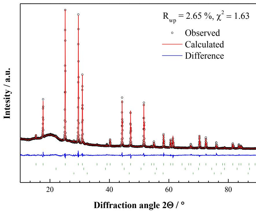
Figure S6. X-ray powder diffraction data for  $\text{Li}_{6.15}\text{P}_{0.85}\text{Si}_{0.15}\text{S}_5\text{Br}$  and the corresponding Rietveld refinements. Shown are the collected data, the profile fit, the profile residuals and the Bragg reflections for the main phase (top).
