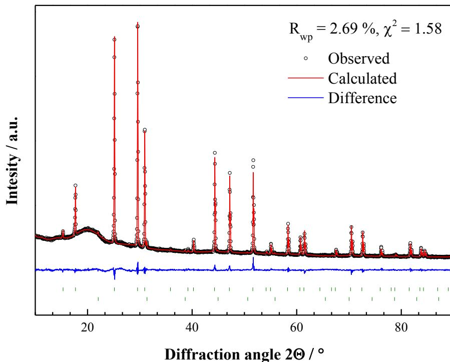
Figure S2. X-ray powder diffraction data for  $\text{Li}_{6.025}\text{P}_{0.975}\text{Si}_{0.025}\text{S}_5\text{Br}$  and the corresponding Rietveld refinements. Shown are the collected data, the profile fit, the profile residuals and the Bragg reflections for the main phase (top).
