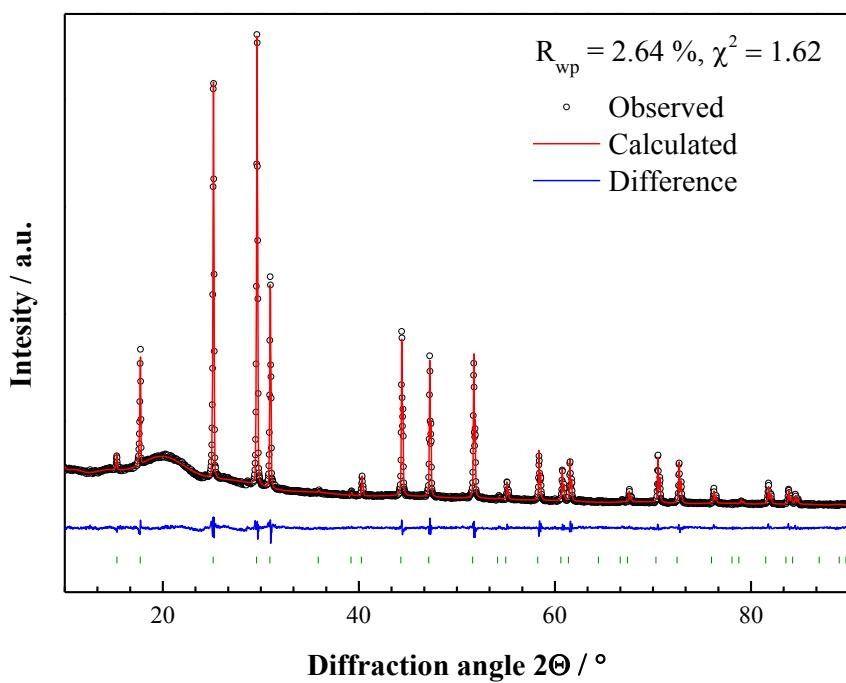
Figure S1. X-ray powder diffraction data for  $\text{Li}_6\text{PS}_5\text{Br}$  and the corresponding Rietveld refinements. Shown are the collected data, the profile fit, the profile residuals and the Bragg reflections for the main phase (top).
