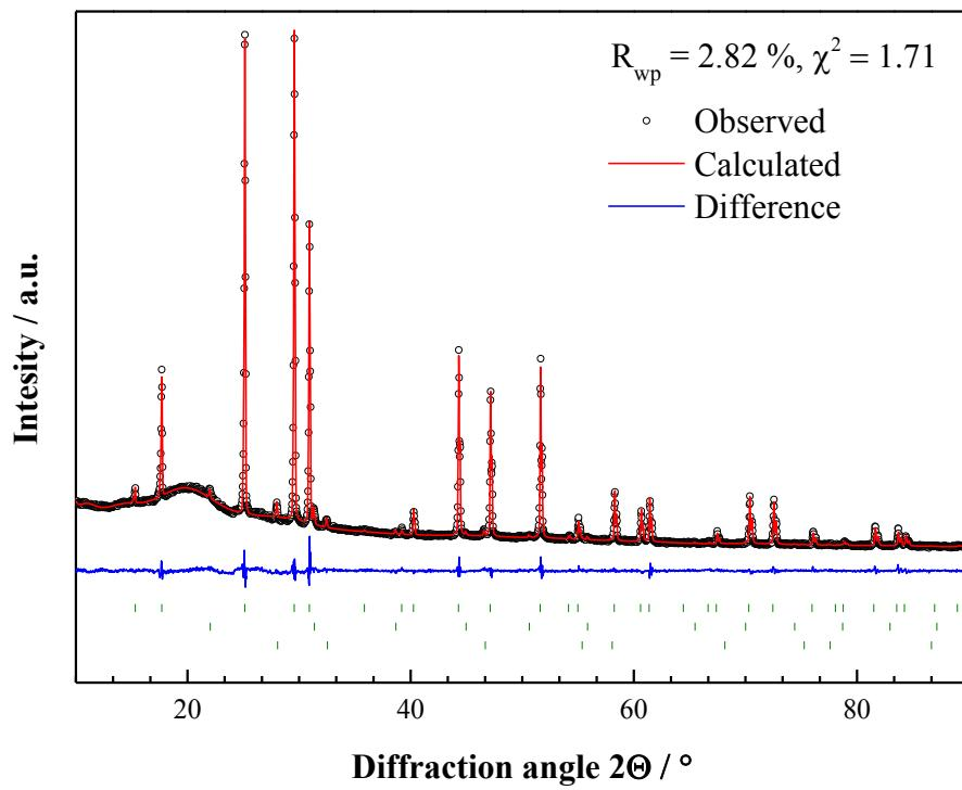
Figure S3. X-ray powder diffraction data for  $\text{Li}_{6.05}\text{P}_{0.95}\text{Si}_{0.05}\text{S}_5\text{Br}$  and the corresponding Rietveld refinements. Shown are the collected data, the profile fit, the profile residuals and the Bragg reflections for the main phase (top).
