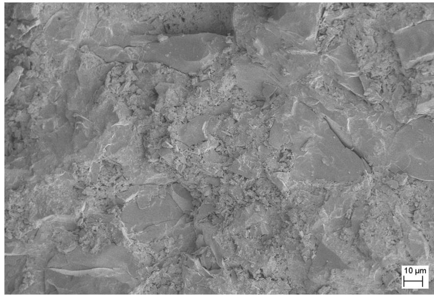
Figure S16: Scanning electron micrograph of  $\text{Li}_6\text{PS}_5\text{Br}$ , showing highly dense samples with good grain contact.
