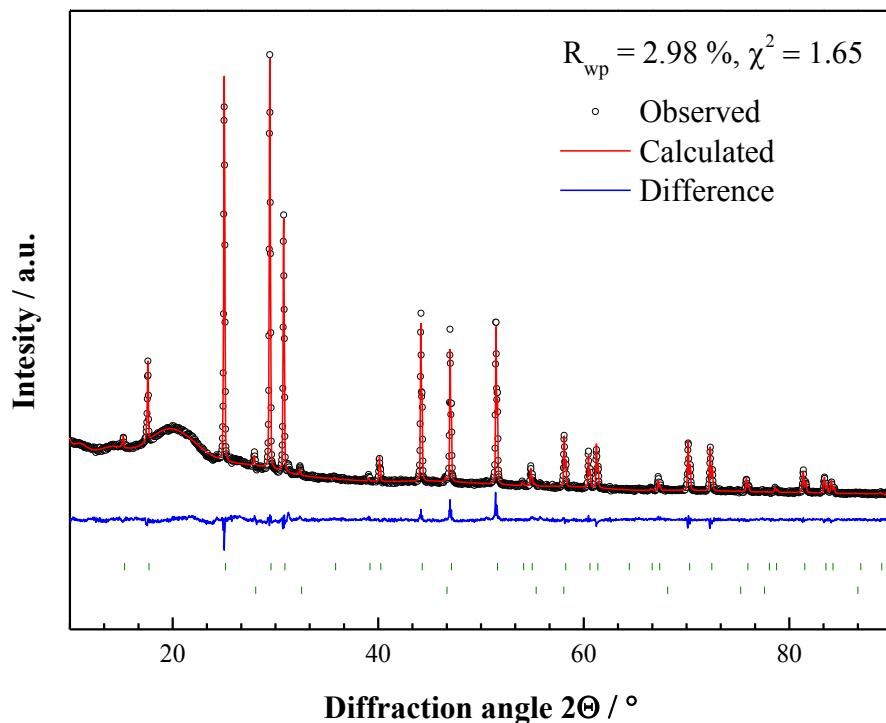
Figure S7. X-ray powder diffraction data for  $\text{Li}_{6.175}\text{P}_{0.825}\text{Si}_{0.175}\text{S}_5\text{Br}$  and the corresponding Rietveld refinements. Shown are the collected data, the profile fit, the profile residuals and the Bragg reflections for the main phase (top).
