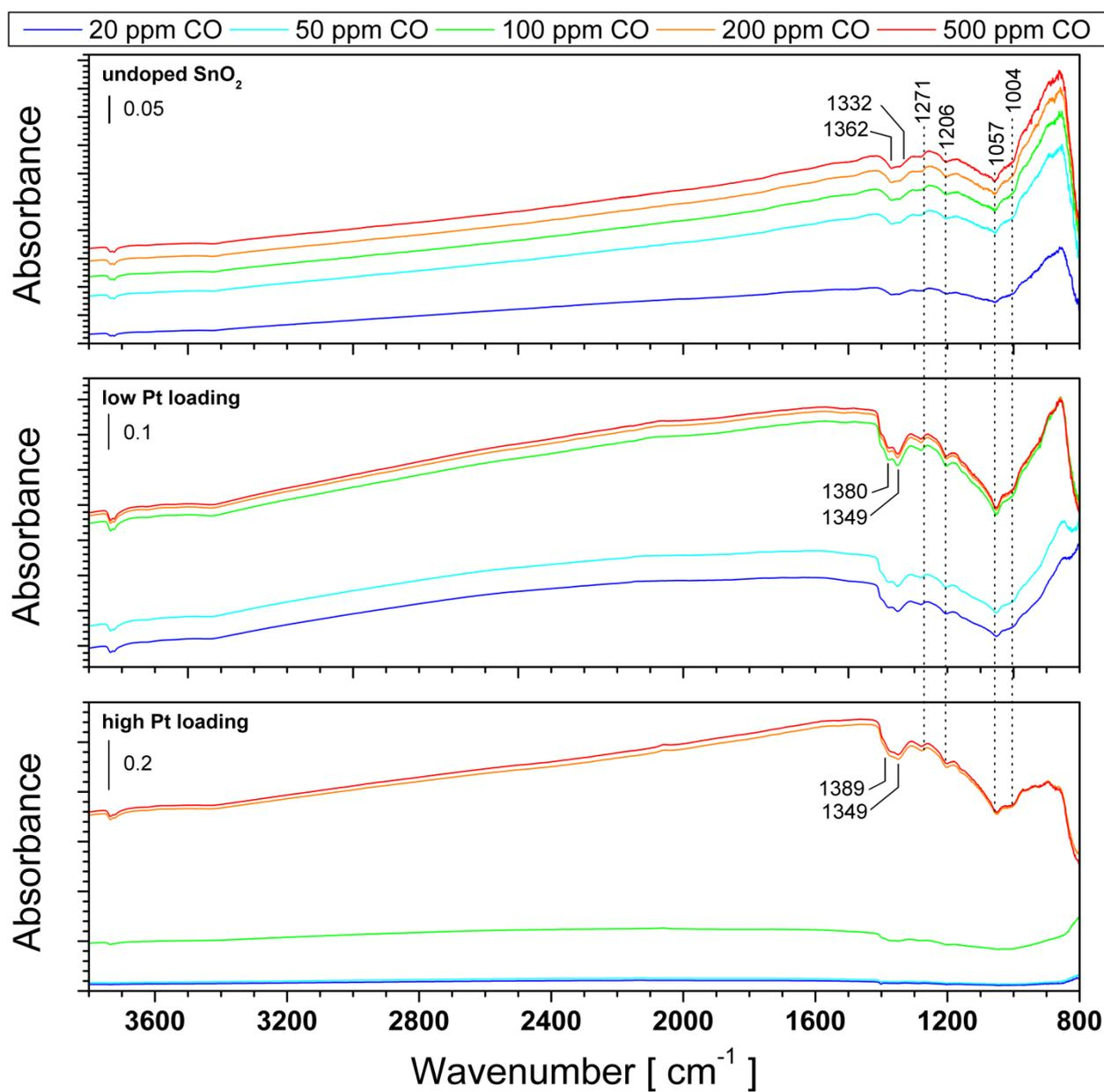
Figure S9. Full DRIFT spectra of undoped (top), LL (middle) and HL (bottom) sample recorded during CO exposure in low oxygen backgrounds.
