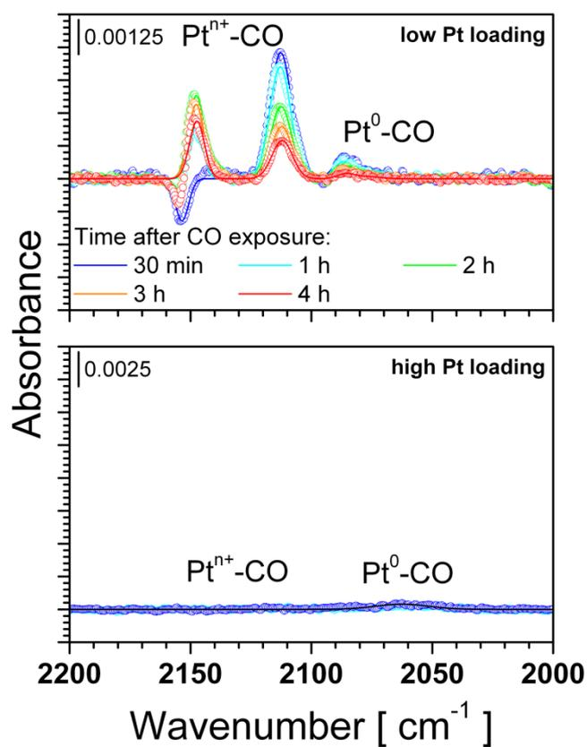
**Figure S11.** Baseline corrected DRIFT spectra of the LL (top) and HL (bottom) sample recorded after the CO exposure in low oxygen backgrounds. The spectra recorded during exposure are shown in the manuscript (Figure 7), the corresponding resistance measurements in Figure S10.
