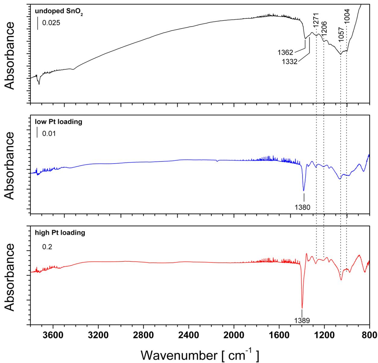
Figure S8. DRIFT spectra of the undoped (black), LL (blue) and HL (red) samples exposed to 10% r.h.; the spectra are referenced to dry air.
