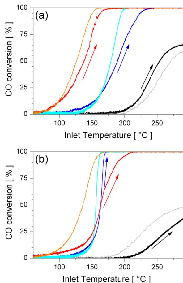
**Figure S6.** CO conversion curves (1<sup>st</sup> heating-cooling cycle) of SnO<sub>2</sub> (black/gray), LL (blue/cyan) and HL (red/orange) samples in dry air (a) and 50% r.h. (b) CO containing atmosphere. The dark colors refer to the heating and the light colors to the cooling process of the catalysts (heating indicated by arrows); Catalyst amount: 100 mg, GHSV = 23000 h<sup>-1</sup>, total gas flow 350 mL/Min, 300 ppm CO, 21% O<sub>2</sub>, N<sub>2</sub> balance.
