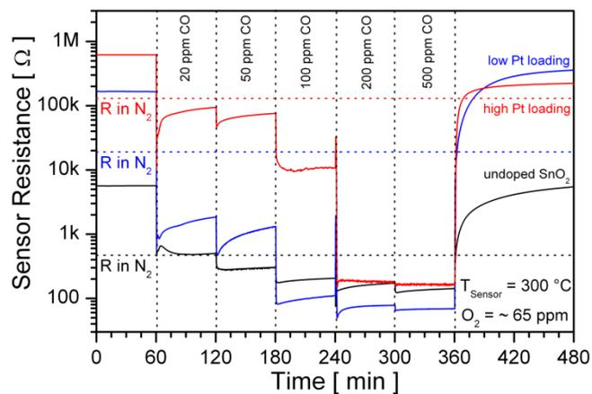
**Figure S10.** Resistance measurements of undoped (black), LL (blue) and HL (red) samples during DRIFTS in low oxygen backgrounds. The horizontal lines ( $R$  in  $N_2$ ) show the sensor resistance in pure  $N_2$ .
