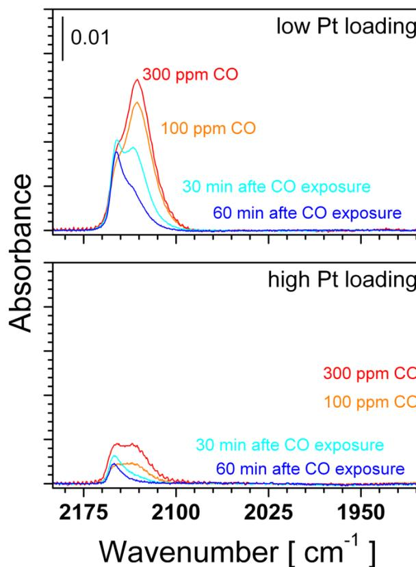
**Figure S7.** DRIFT spectra of LL (top) and HL (bottom) sample during and after the CO exposure at 300 °C in dry air.
