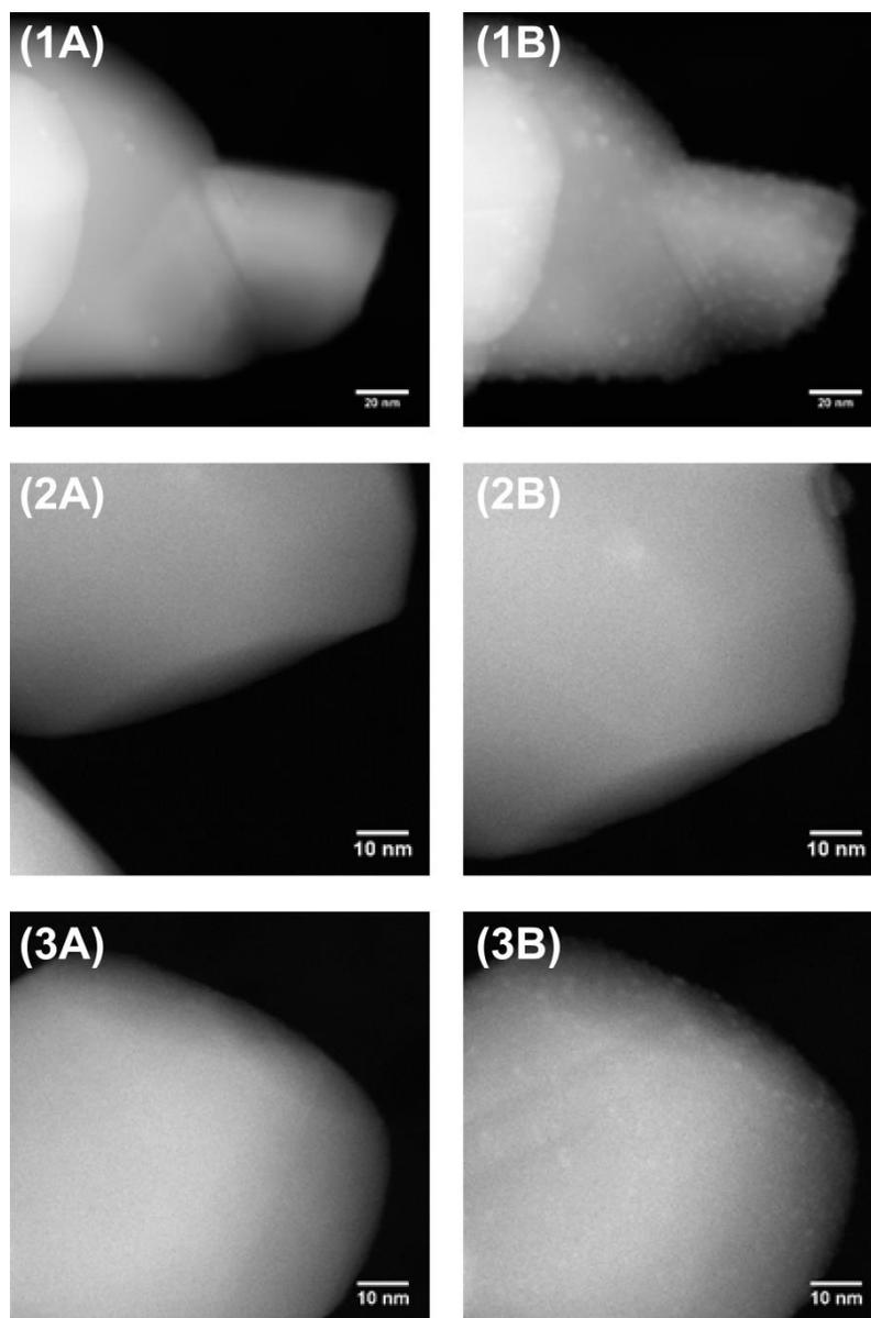
Figure S5. STEM-HAADF images of the unused (1) and used (2,3) sensor materials. The HL sample is shown in (1) and (3) and the LL sample in (2). On the left (A) the original material is shown and on the right (B) the one after beam exposure for 7 min (2B & 3B) or 5 min (1B). lowly Pt-loaded SnO<sub>2</sub> (A) original material, (B) after 7 min electron beam exposure (5 min in case of (1B)).
