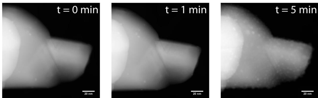
Figure S4. HAADF-STEM images of unused HL sample after 0, 1 and 5 min of electron beam exposure.
