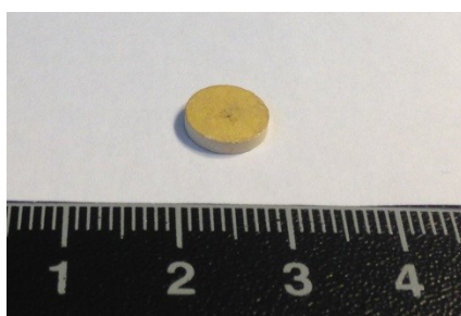
Figure S6. Shape and size of La 2 LiNbO 6 pellet used to study the electric response on RH%.
