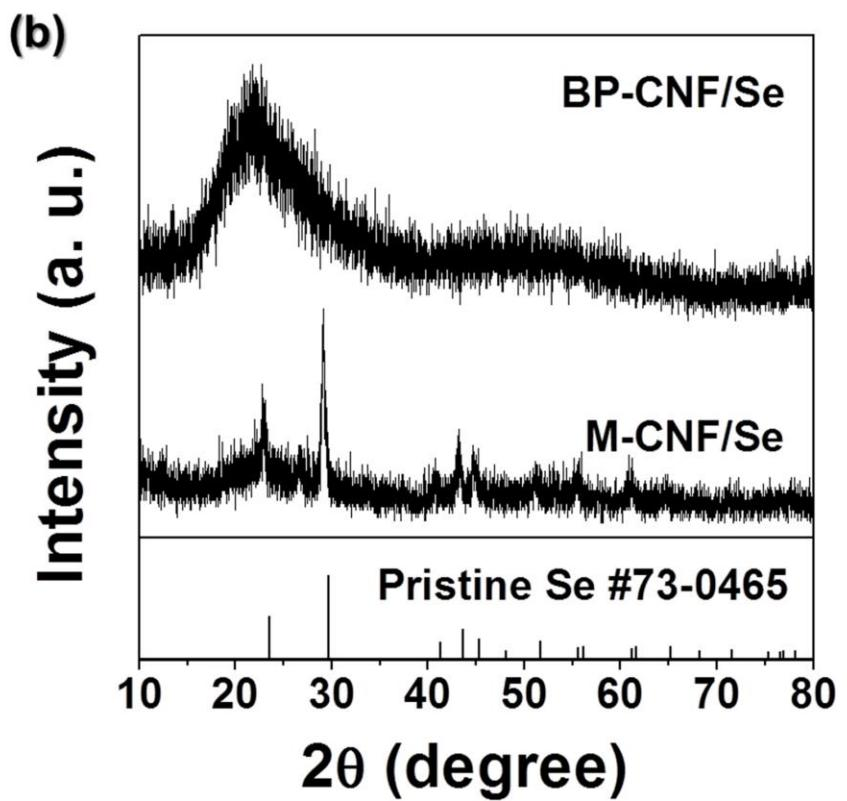
**Fig. S5.** (a) SEM image of M-CNF/Se, (b) XRD patterns of M-CNF/Se and BP-CNF/Se, and (c) SEM image of BP-CNF/Se.
