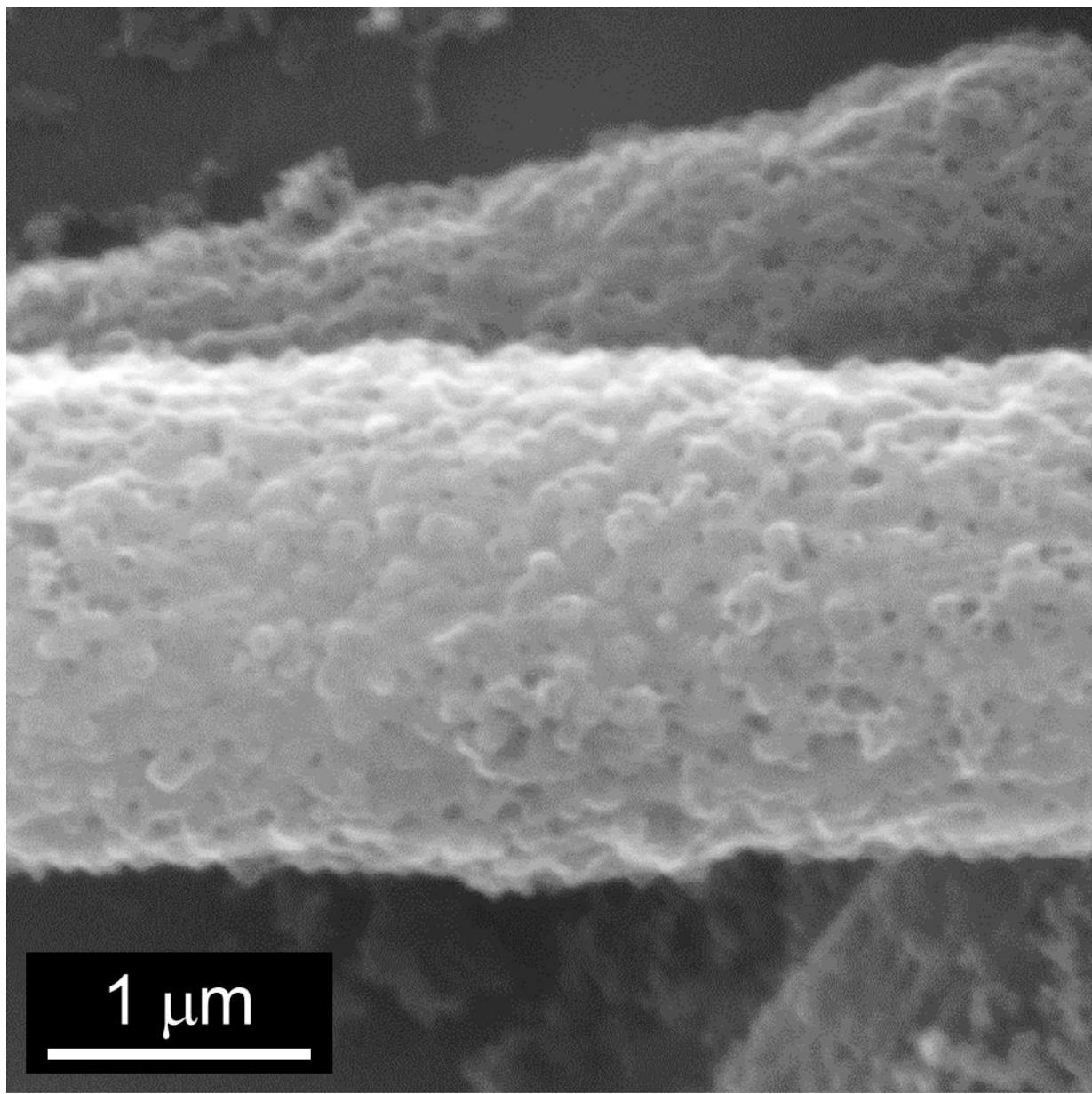
**Fig. S7.** SEM image of BP-CNF/Se nanofiber after 50 cycles at 0.5 C.
