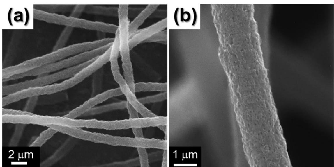
**Fig. S2.** (a) Low and (b) high resolution SEM images of M-CNF.
