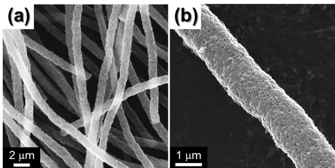
**Fig. S4.** (a) Low and (b) high resolution SEM images of BP-CNF.
