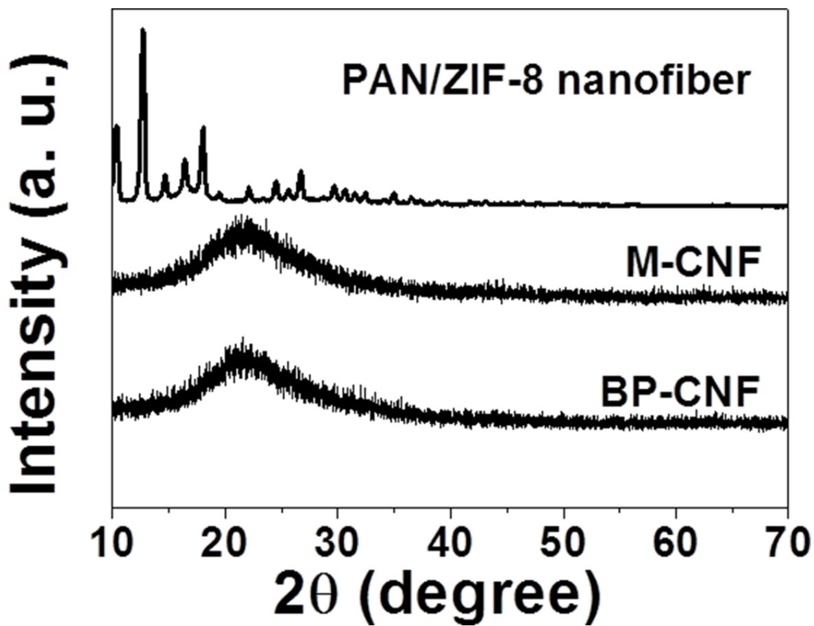
**Fig. S3.** XRD patterns of PAN/ZIF-8 nanofiber, M-CNF, and BP-CNF.
