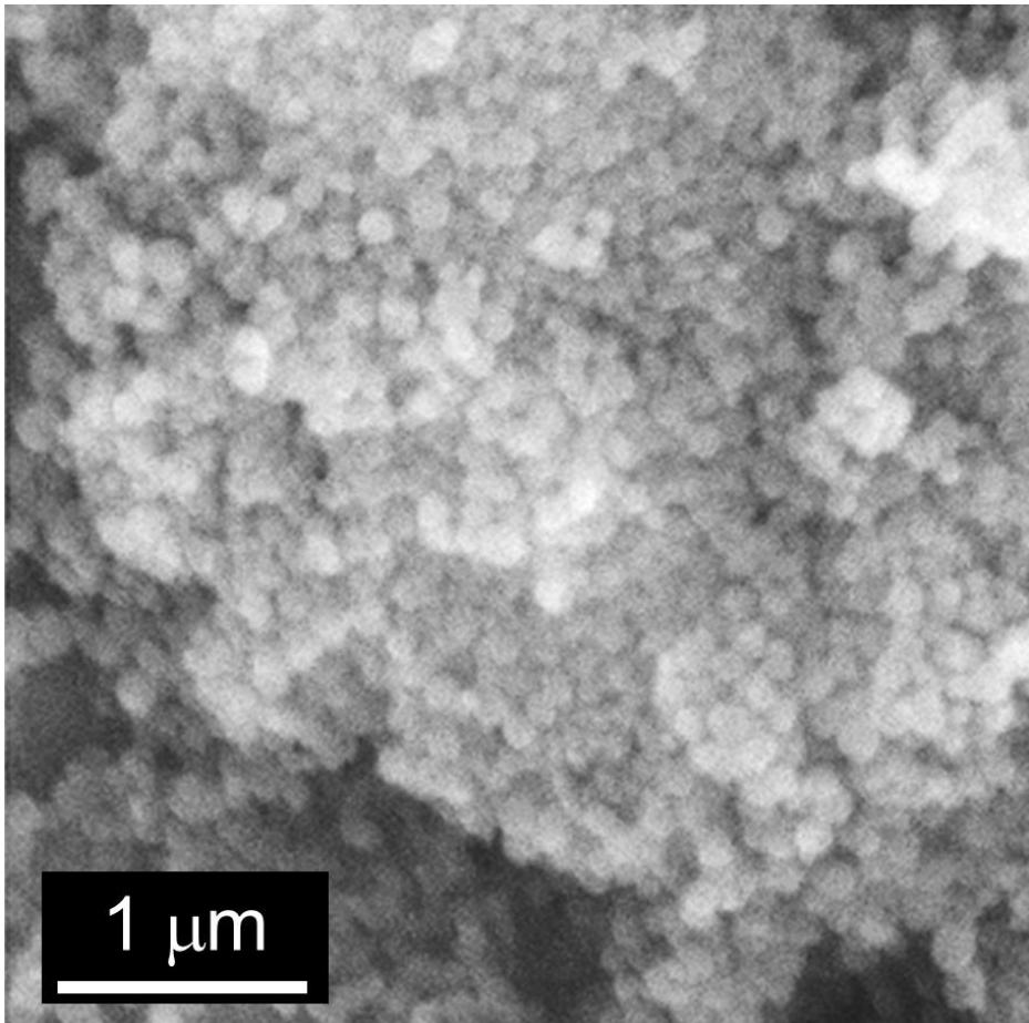
**Fig. S1.** SEM images of ZIF-8 nanoparticles constituting PAN/ZIF-8 nanofibers.
