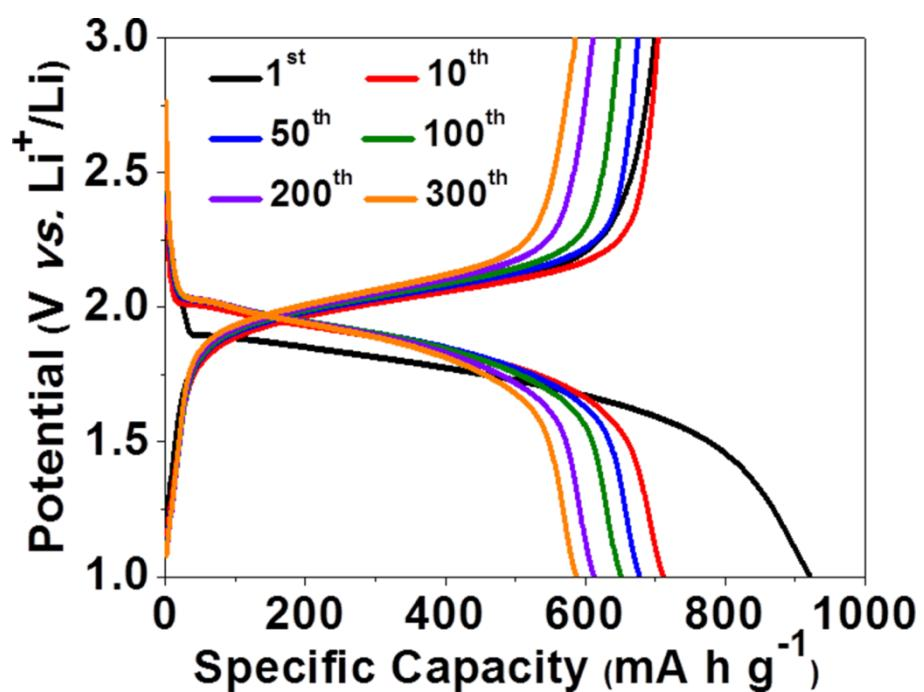
**Fig. S6.** Charge-discharge profiles of BP-CNF/Se electrode at 1<sup>st</sup>, 10<sup>th</sup>, 50<sup>th</sup>, 100<sup>th</sup>, 200<sup>th</sup>, and 300<sup>th</sup> cycles.
