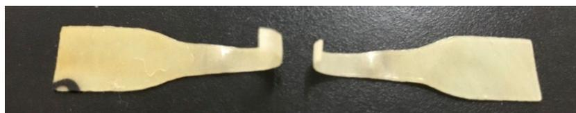
**Fig. S13** The photograph of tensile-failure PUU- $g$ -C<sub>3</sub>N<sub>4</sub> NSs-1.0 nanomaterials
