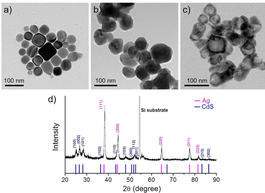
**Fig. S8** TEM images of (a) Ag NPs, (b) Ag@Ag<sub>2</sub>S core-shell NPs, and (c) CdS HNPs. CdS HNPs with distinct hollow interior were prepared by the cation exchange reaction of Ag@Ag<sub>2</sub>S core-shell NPs, which were produced by the sulfidation reaction of Ag NPs. (d) XRD pattern of CdS HNPs. The positions of Ag and CdS references in the XRD pattern were taken from the JCPDS database (Ag: 04-0783, CdS: 41-1049).
