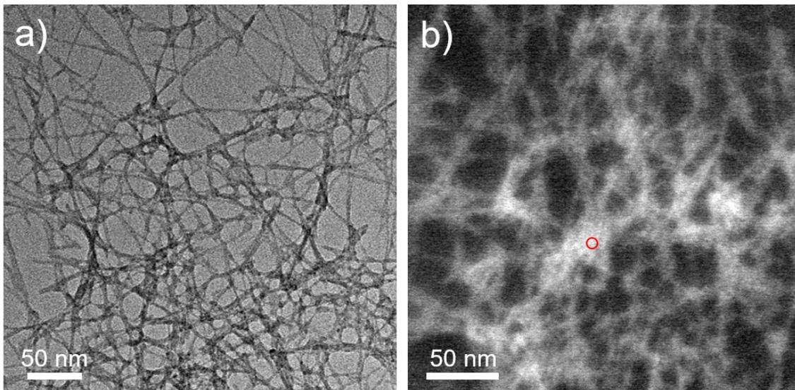
**Fig. S6** (a) Bright- and (b) dark-field TEM images of tangled nanowires consisting Ag and Cd formed by the addition of  $\text{NaBH}_4$  to the reaction mixture after the cation exchange reaction. The EDS-determined Ag:Cd atomic ratio of nanowires was 1:6.9. The position of EDS analysis is denoted by a red circle in b.
