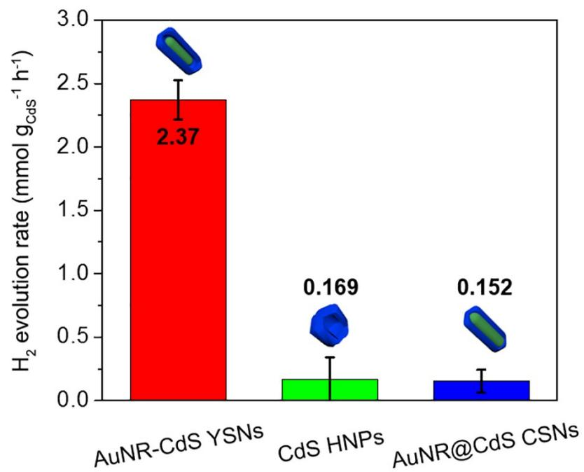
**Fig. S9** Hydrogen evolution rates of different catalysts with respect to the mass of CdS in catalysts.
