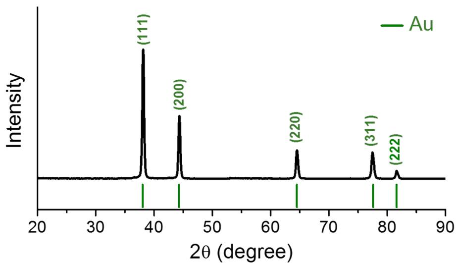
**Fig. S1** XRD pattern of AuNRs. The positions of Au reference were taken from the JCPDS database (Au: 65-2870).
