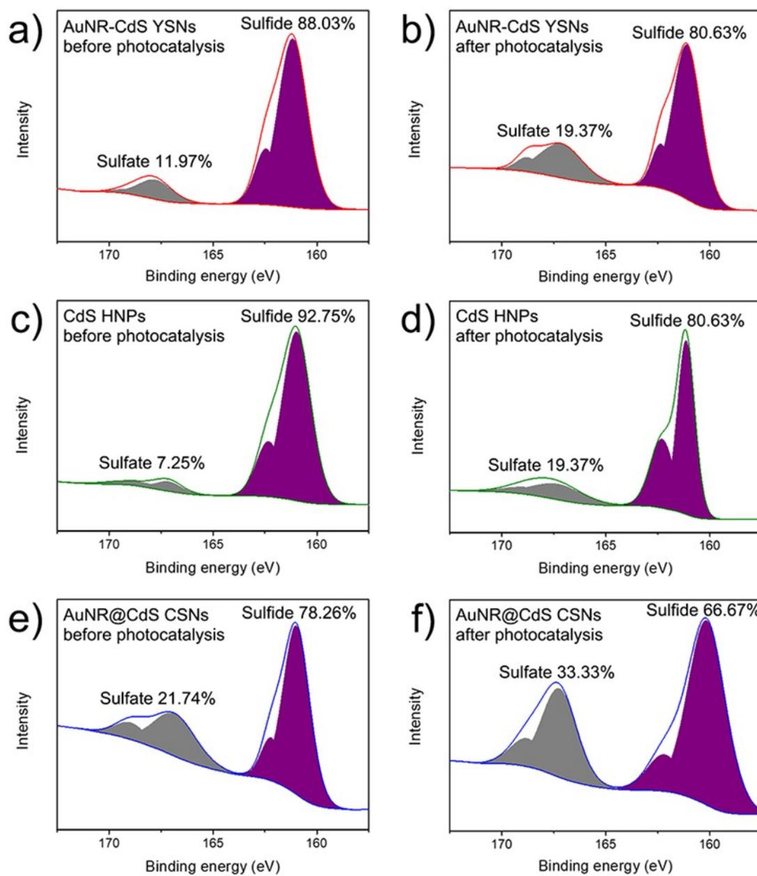
**Fig. S10** XPS spectra of S 2p regions for (a,b) AuNR-CdS YSNs, (c,d) CdS HNPs, and (e,f) AuNR@CdS CSNs.
