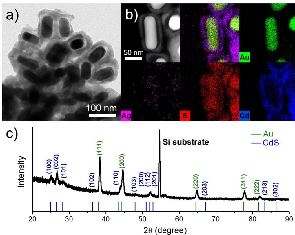
**Fig. S4** (a) TEM, (b) HAADF-STEM and corresponding EDS elemental mapping images, and (c) XRD pattern of AuNR@CdS YSNs obtained after a cation exchange reaction in water, while keeping other reaction conditions the same as the typical synthesis of the AuNR-CdS YSNs. The positions of Au and CdS references in the XRD pattern were taken from the JCPDS database (Au: 65-2870, CdS: 41-1049).
