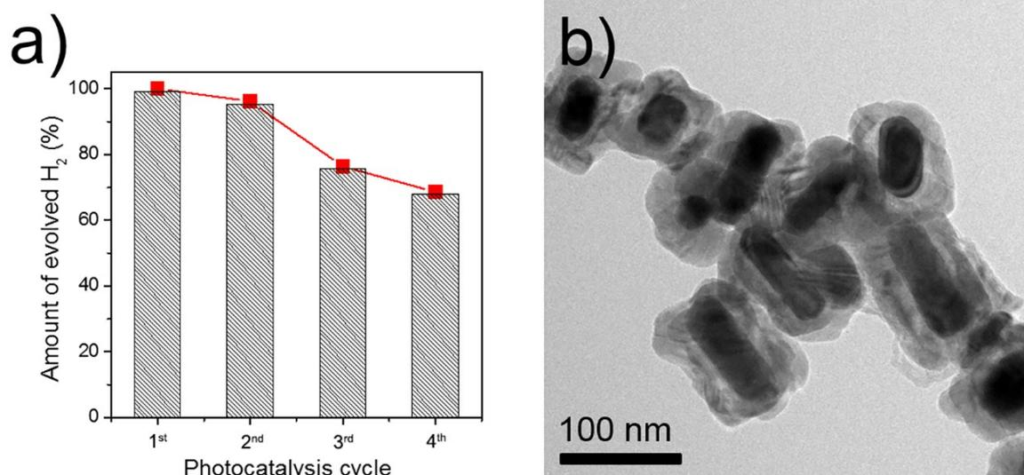
**Fig. S12** (a) Recyclability of AuNR-CdS YSNs for photocatalytic hydrogen evolution. Each photocatalysis cycle was conducted for 2 h. After each photocatalysis run, the catalysts were collected from the reaction solution by centrifuging (8,000 rpm for 7 min), and then subjected to the next photocatalytic reaction. (b) TEM image of AuNR-CdS YSNs after the fourth cycle of photocatalysis, revealing that most of the nanostructures maintained their original morphology.
