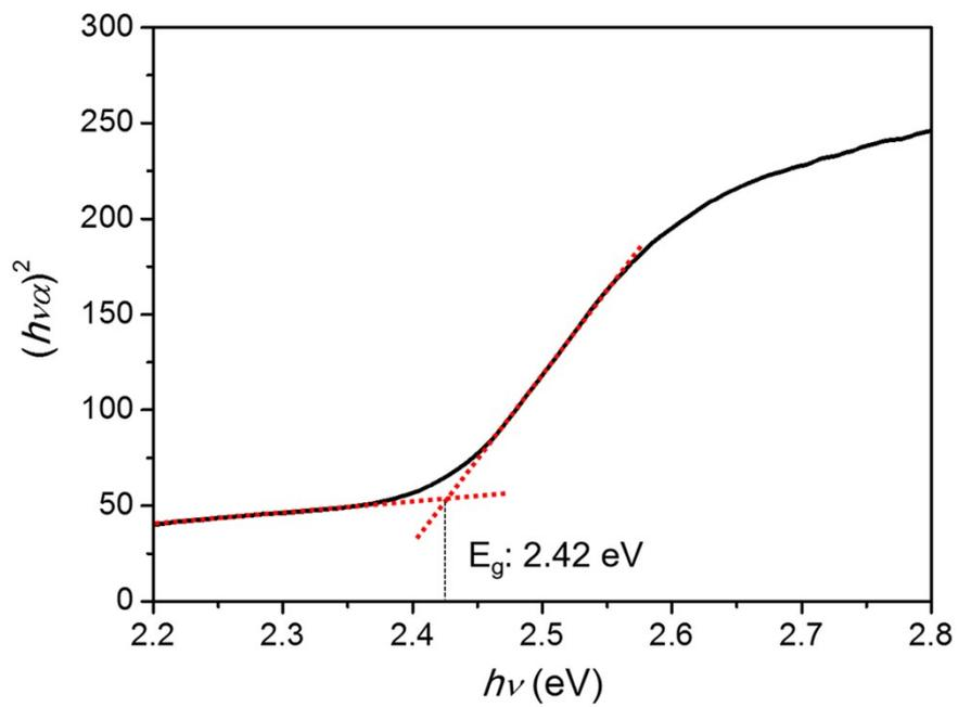
**Fig. S14** Tauc plot for calculating the band gap energy ( $E_g$ ) of CdS HNPs. The  $E_g$  of CdS HNPs was calculated to be 2.42 eV.
