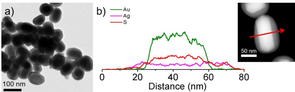
**Fig. S7** (a) TEM image and (b) HAADF-STEM image and corresponding EDS cross-sectional compositional line profiles of AuNR@Ag@Ag<sub>2</sub>S CSSNs stored in methanol containing TBP for 24 h.
