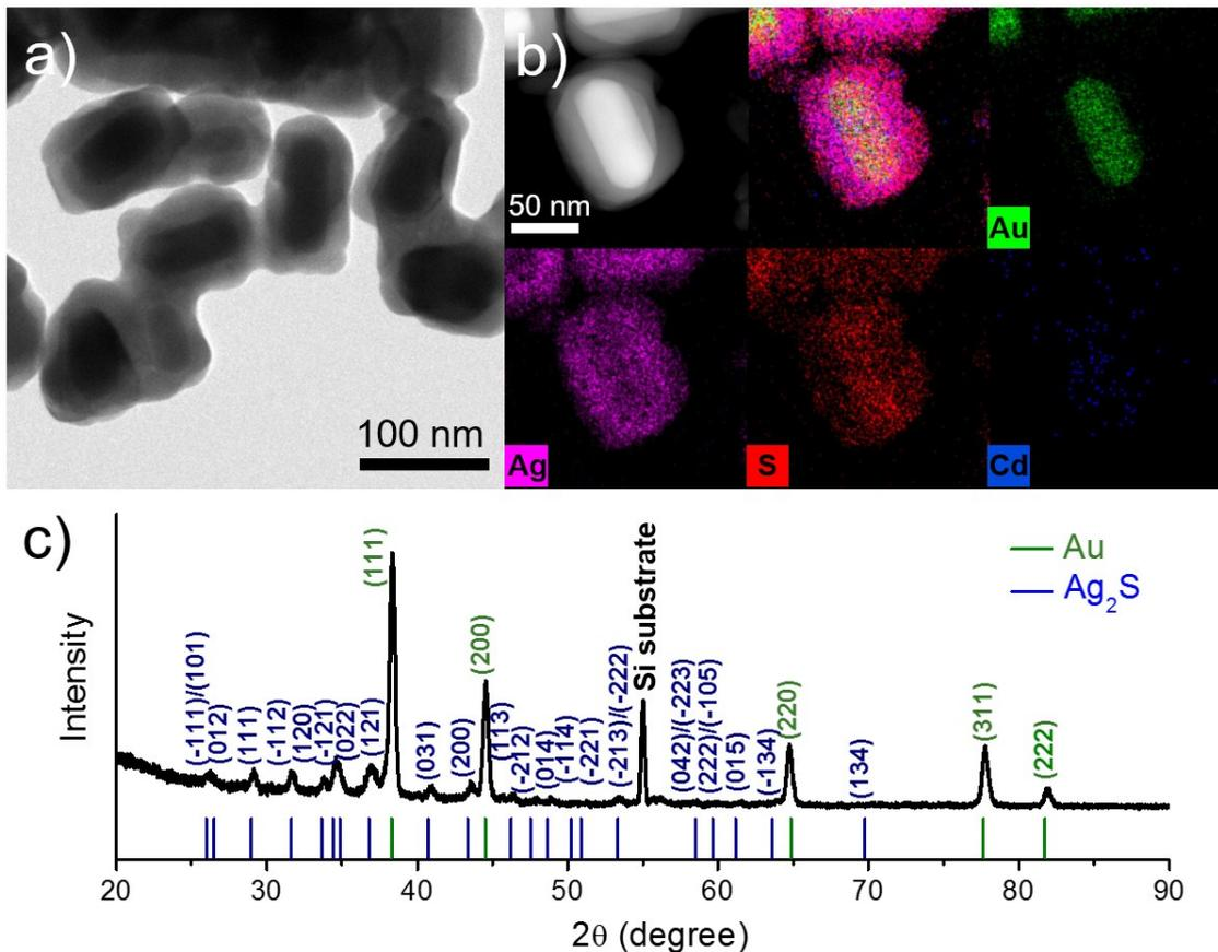
**Fig. S3** (a) TEM, (b) HAADF-STEM and corresponding EDS elemental mapping images, and (c) XRD pattern of AuNR@Ag@Ag<sub>2</sub>S CSSNs obtained after a cation exchange reaction in the absence of TBP, while keeping other reaction conditions the same as the typical synthesis of the AuNR-CdS YSNs. The positions of Au and Ag<sub>2</sub>S references in the XRD pattern were taken from the JCPDS database (Au: 65-2870, Ag<sub>2</sub>S: 14-0072).
