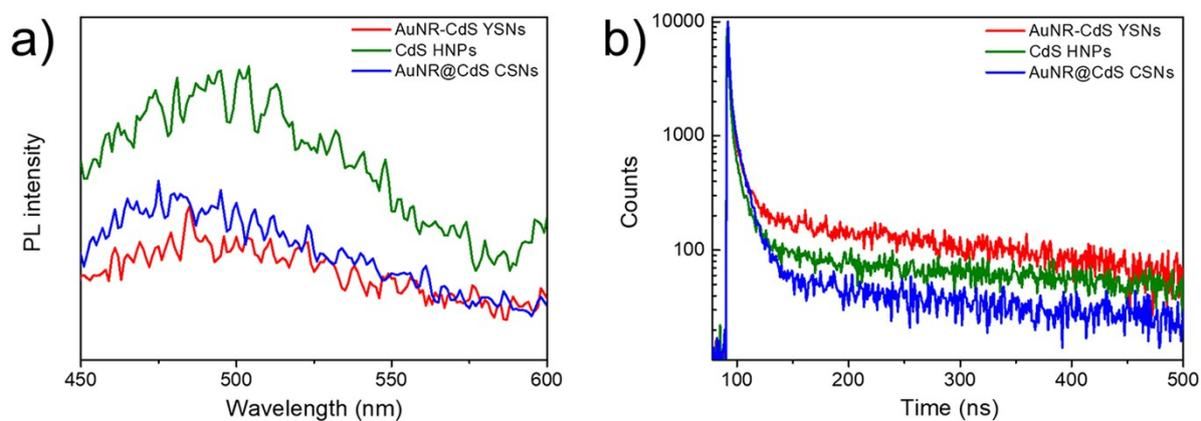
**Fig. S11** (a) Steady-state PL spectra and (b) time-resolved PL decays of AuNR-CdS YSNs, CdS HNPs, and AuNR@CdS CSNs in an aqueous solution containing  $\text{Na}_2\text{S}$  (0.25 M) and  $\text{Na}_2\text{SO}_3$  (0.35M). The excitation wavelength was 375 nm.
