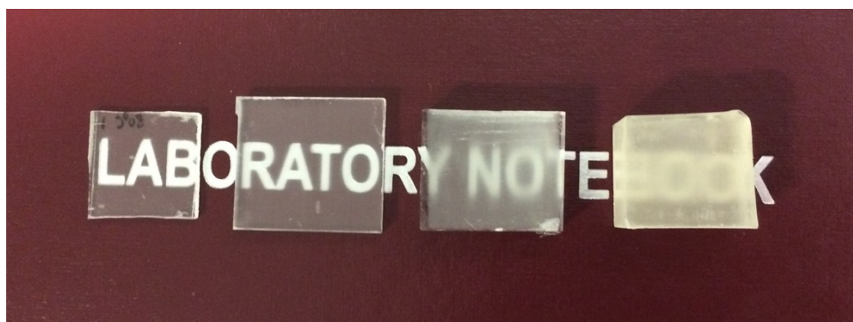
Figure S1 Photograph of acetylated transparent wood with thickness of 1.5, 3, 7, and 10 mm.
