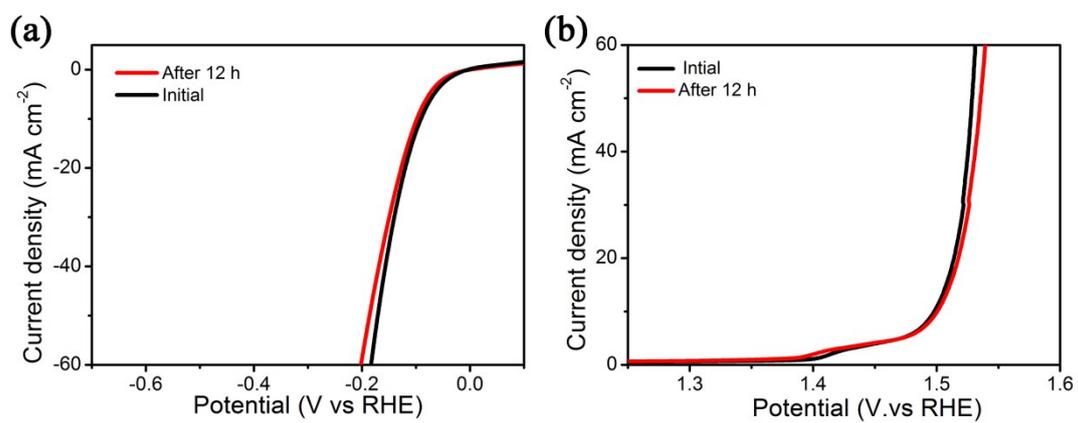
**Fig. S11** (a, b) The stability of Co<sub>3</sub>O<sub>4</sub>@MoS<sub>2</sub>/CC for HER and OER.
