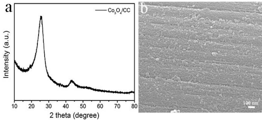
**Fig. S2** (a) The XRD pattern of  $\text{Co}_3\text{O}_4/\text{CC}$ ; (b) the SEM images of  $\text{Co}_3\text{O}_4/\text{CC}$ .
