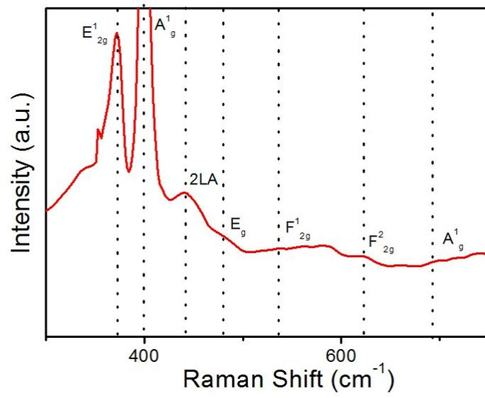
Fig. S5 the Raman spectra of Co<sub>3</sub>O<sub>4</sub>@MoS<sub>2</sub>/CC.
