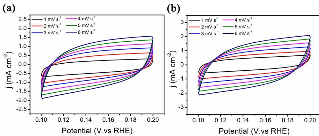
**Fig. S7** Cyclic voltammograms at different scan rates in the region between -100 and -200 mV (vs. RHE): (a)  $\text{Co}_3\text{O}_4@\text{MoS}_2$ , (b)  $\text{MoS}_2$
