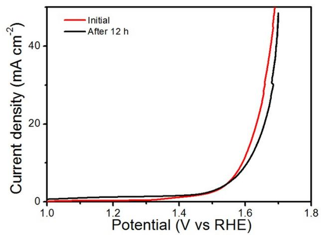
**Fig. S10** the LSV of water splitting after long time test.
