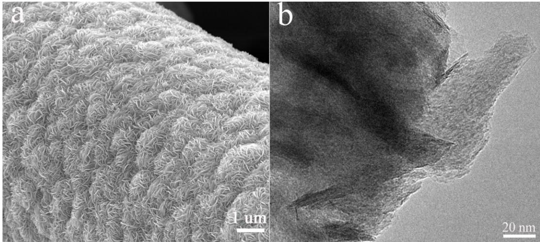
**Fig. S4** (a) The SEM image of MoS<sub>2</sub>; (b) TEM image of MoS<sub>2</sub>.
