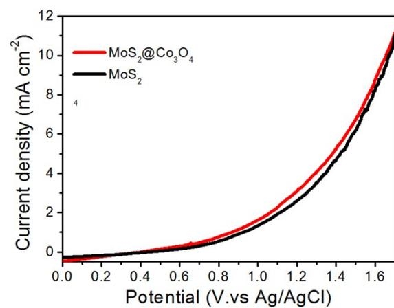
**Fig. S9.** The OER polarizaiton curves of MoS<sub>2</sub>, Co<sub>3</sub>O<sub>4</sub> and Co<sub>3</sub>O<sub>4</sub>@MoS<sub>2</sub> in 0.5 M H<sub>2</sub>SO<sub>4</sub>. Scan rate: 2 mV s<sup>-1</sup>.
