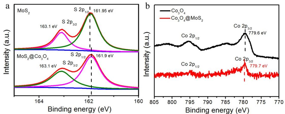
**Fig. S3** (a) the S XPS spectra of MoS<sub>2</sub>/CC and Co<sub>3</sub>O<sub>4</sub>@MoS<sub>2</sub>/CC; (b) the Co XPS spectra of Co<sub>3</sub>O<sub>4</sub>/CC and Co<sub>3</sub>O<sub>4</sub>@MoS<sub>2</sub>/CC.
