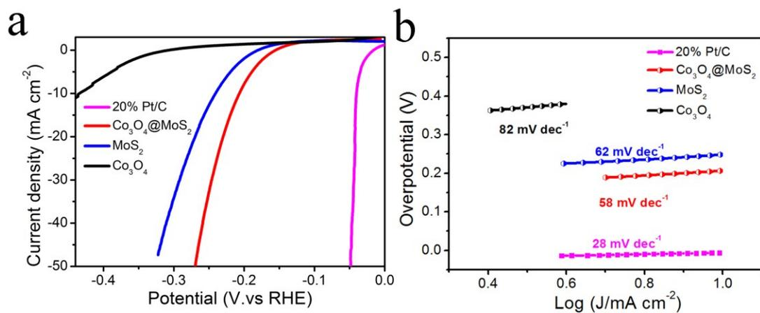
**Fig. S6** Electrochemical characterization of hydrogen evolution reaction. (a) Polarization curves (b) corresponding Tafel plots of 20% Pt/C, MoS<sub>2</sub>, Co<sub>3</sub>O<sub>4</sub> and Co<sub>3</sub>O<sub>4</sub>@MoS<sub>2</sub> in 1 M KOH. Scan rate: 5 mV s<sup>-1</sup>.
