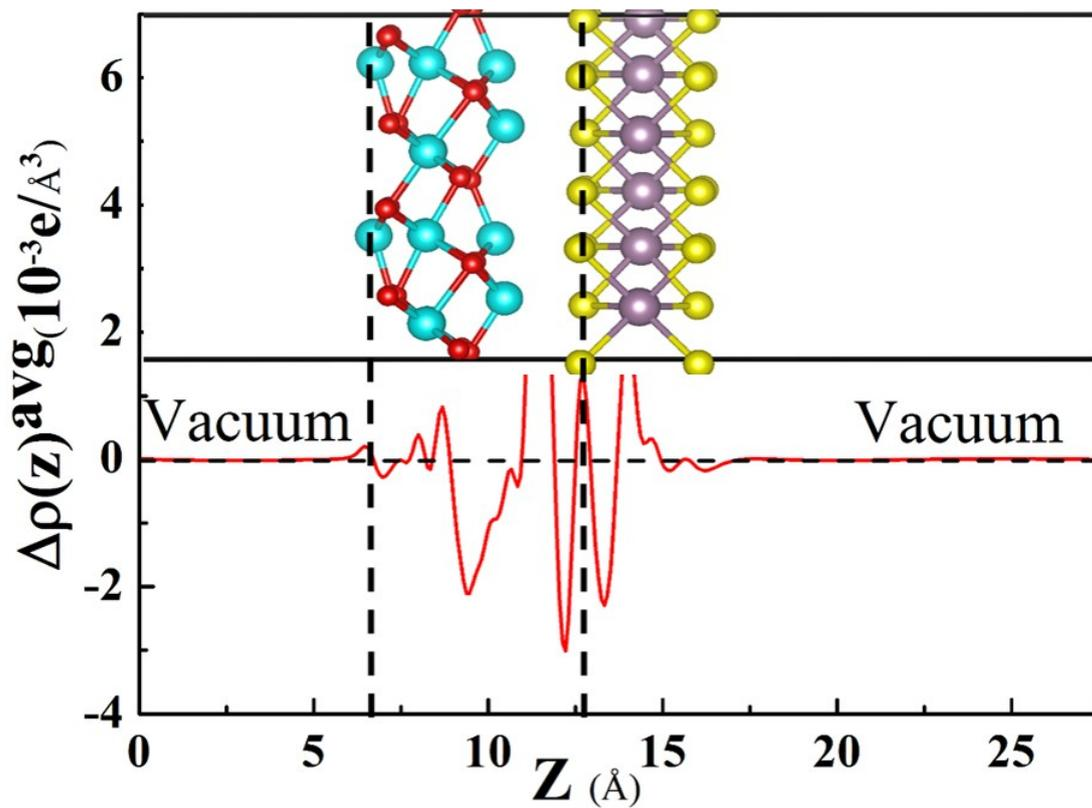
Fig. S1 isosurface of local charge density difference of  $\text{Co}_3\text{O}_4$ @ $\text{MoS}_2$  interface.
