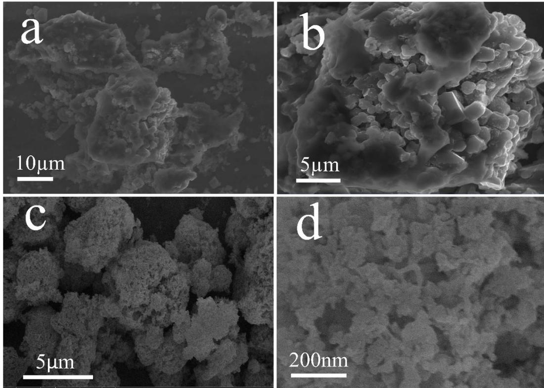
**Fig. S3** SEM images of (a)-(b) as-prepared Mg<sub>2</sub>Si, (c)-(d) pSi nanoparticles from 200 mesh commercial Si as the raw material.
