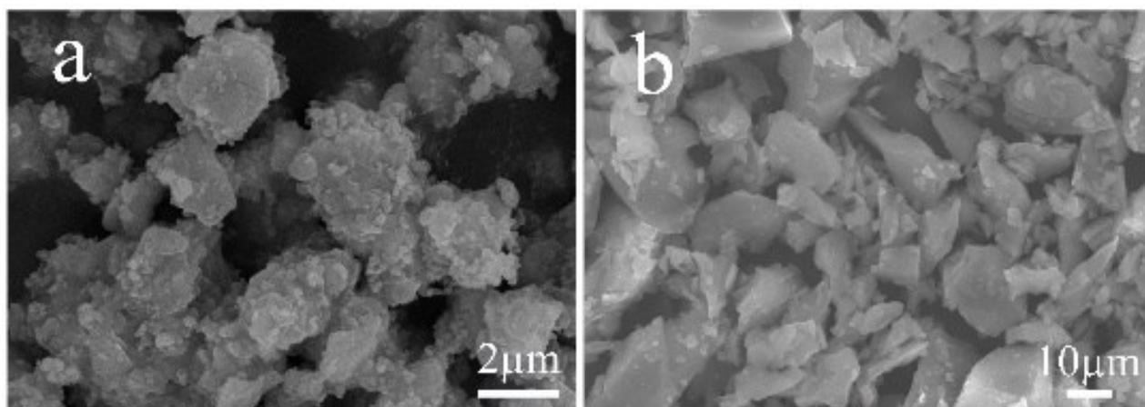
**Fig. S1** SEM images of the size and morphologies of (a)  $\sim 2\mu\text{m}$  Si powders and (b) 200 mesh commercial Si powders.
