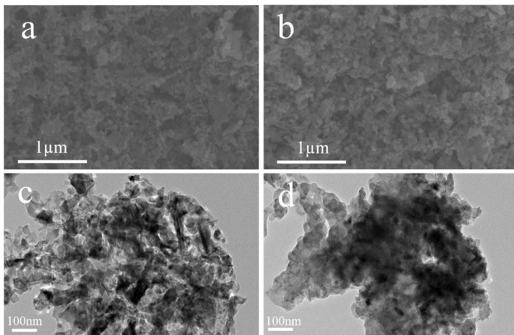
**Fig. S13** SEM images of B-doped porous Si electrodes before (a) and (b) after 100 cycles and TEM images of B-doped porous Si materials before (c) and (d) after 100 cycles.
