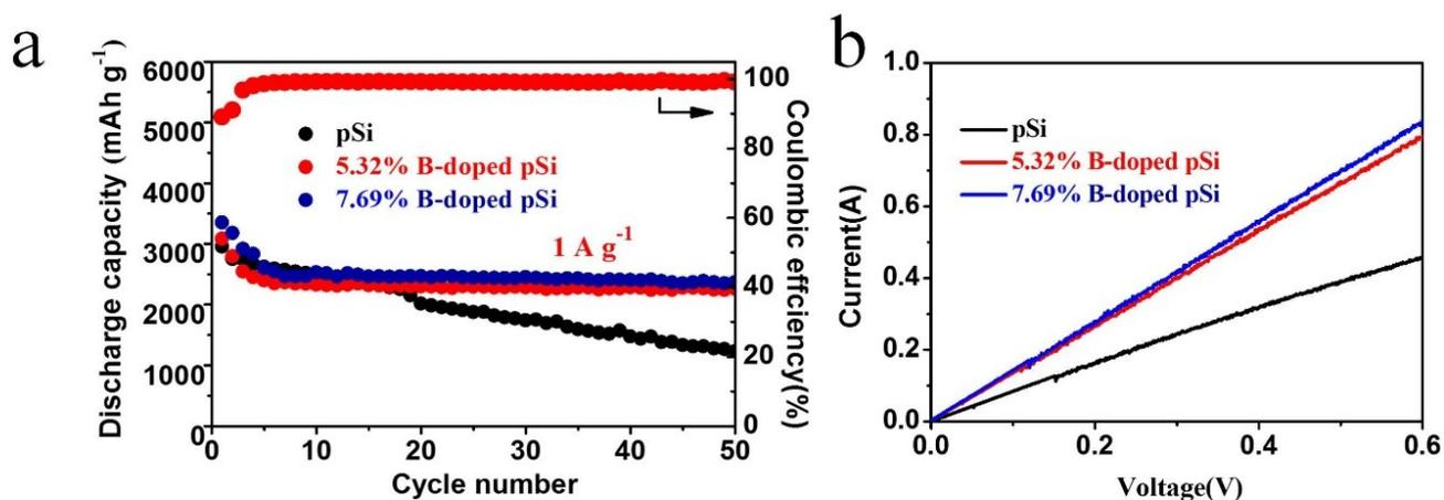
**Fig. S10** (a) Cycling performances of porous Si and B-doped porous Si (5.32% and 7.69% of B) electrodes at  $1 \text{ A g}^{-1}$ . (b) I-V curves of porous Si and B-doped porous Si (5.32% and 7.69% of B) powders at  $10 \text{ mV/s}$ .
