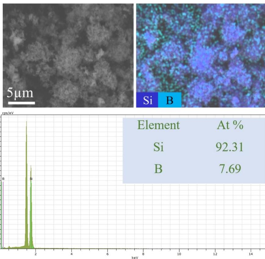
**Fig. S9** EDS mapping and spectrum of HB-doped porous Si material.
