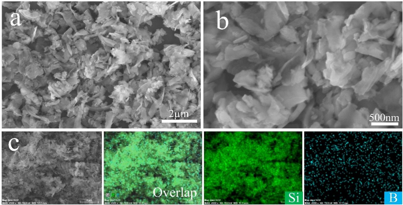
**Fig. S4** SEM images of  $\sim 2\mu\text{m}$  B-doped Si powders milled from commercial p-type Si wafers and corresponding EDS elemental mapping images of Si (green) and B (blue).
