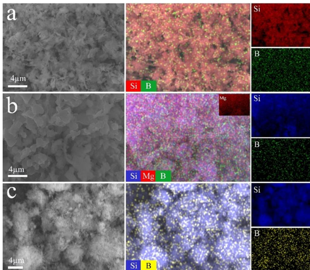
**Fig. S6** EDS mapping images of  $\sim 2 \mu\text{m}$  B-doped Si powders milled from commercial p-type Si wafers (a), the intermediate product of B-doped  $\text{Mg}_2\text{Si}$  alloys (b) and B-doped porous Si material (c).
