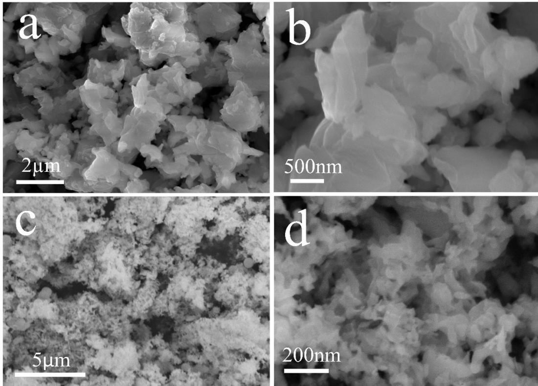
**Fig. S2** SEM images of (a)-(b) as-prepared  $\text{Mg}_2\text{Si}$ , (c)-(d) pSi nanoplates from  $\sim 2\mu\text{m}$  Si powders as the raw material.
