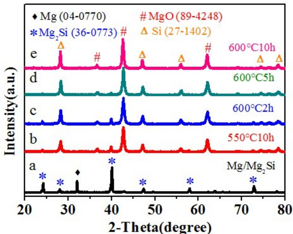
**Fig. S7** XRD patterns of (a) Mg<sub>2</sub>Si/Mg powder, and the as-prepared samples after the air-oxidation process at (b) 550°C for 10 h, (c) 600°C for 2 h, (d) 600°C for 5 h, (e) 600°C for 10 h.
