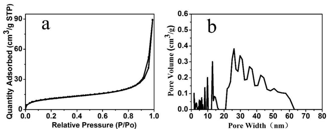
**Fig. S8** (a) Nitrogen adsorption-desorption isotherm curves (b) BJH pore diameter distribution of pSi sample.
