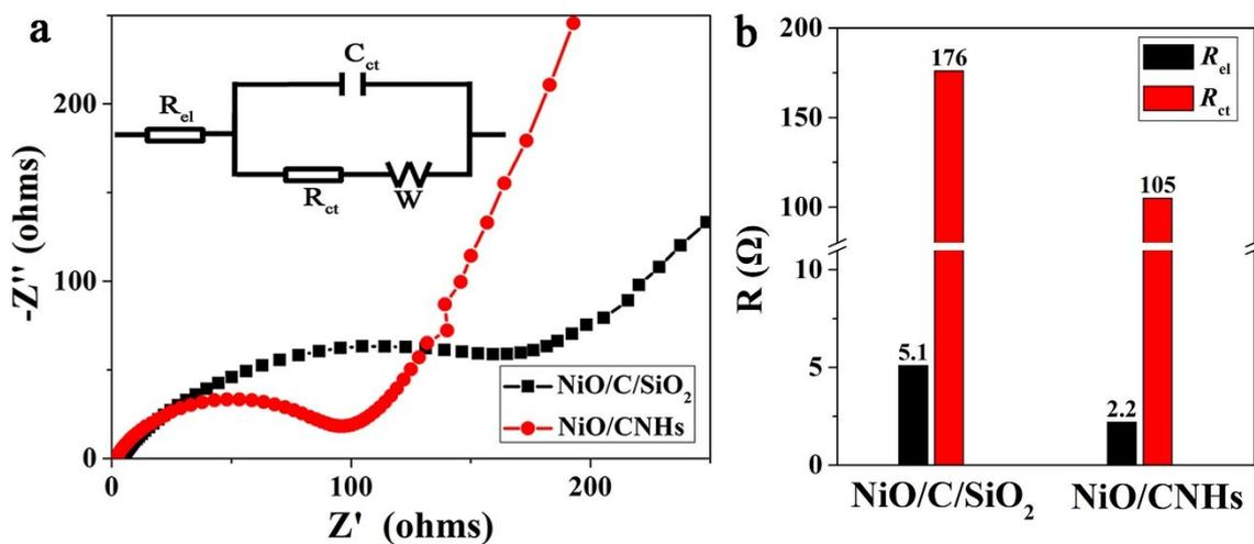
**Fig. S6** (a) EIS of NiO/C/SiO<sub>2</sub> and NiO/CNHs electrodes in fresh LIBs, where the inset shows the equivalent circuit diagram. (b) Comparisons of intrinsic electrode/electrolyte resistances ( $R_{el}$ ) and charger transfer resistances ( $R_{ct}$ ) values between NiO/C/SiO<sub>2</sub> and NiO/CNHs, which are obtained according to the equivalent circuit diagram in (a).
