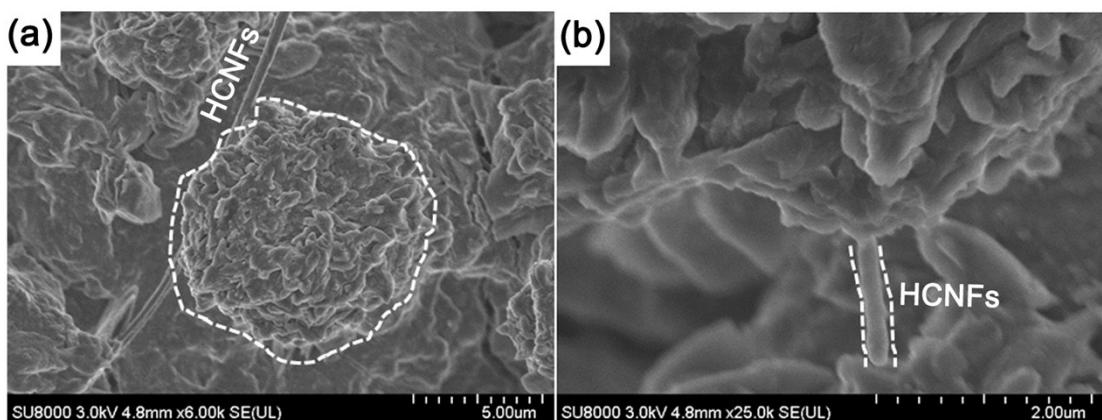
**Figure S7.** SEM images of the MnO/HCNFs composite after 100 cycles at 200 mA g<sup>-1</sup> under different magnifications.
