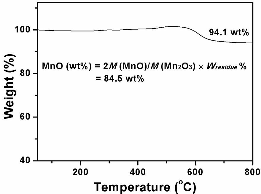
**Figure S3.** TG curve of the prepared MnO/HCNFs under air atmosphere. According to the analysis, the HCNFs content in the MnO/HCNFs composite is calculated to be 15.5 wt%.
