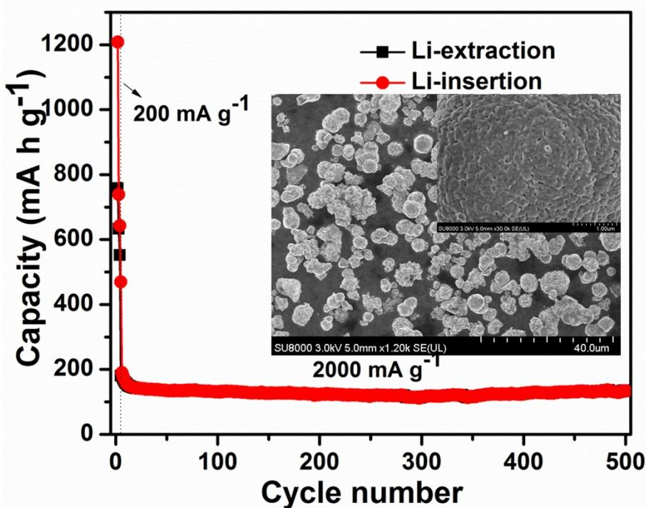
**Figure S4.** Cycling performance of pristine MnO micro-nanospheres prepared by the same method without adding HCNFs at  $2000 \text{ mA g}^{-1}$ .
