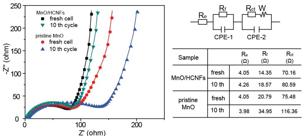
**Figure S6.** Nyquist plots and fitting results of MnO/HCNFs and pristine MnO electrodes before and after the 10th discharge–charge cycle in the voltage range of 0.005–2.9 V.
