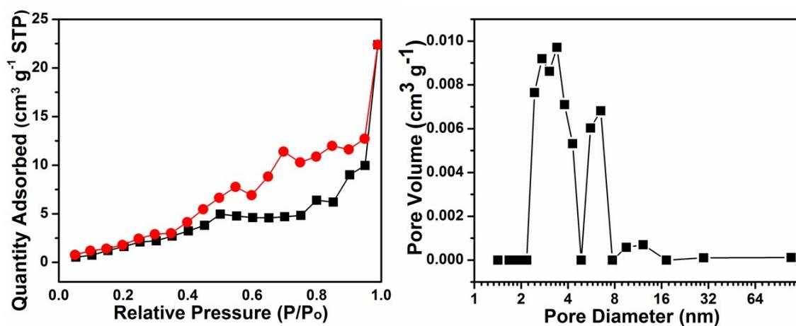
**Figure S2.**  $\text{N}_2$  adsorption–desorption isotherm and its pore size distribution of the prepared  $\text{MnO}/\text{HCNFs}$ .
