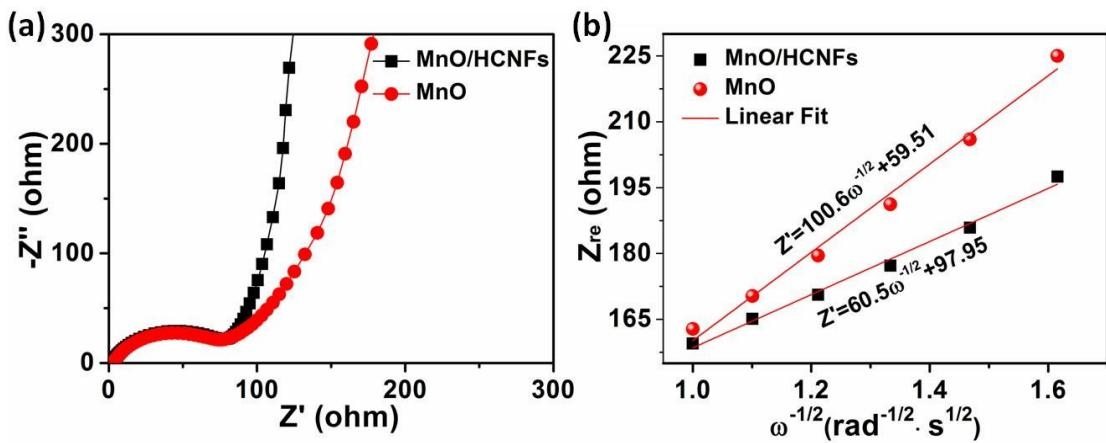
**Figure S5.** (a) Nyquist plots for the fresh cell of MnO/HCNFs and the MnO control. (b) The corresponding relationship between real resistance and frequencies, the slope of the fitting line can be adopted to calculate the ion diffusion coefficient.
