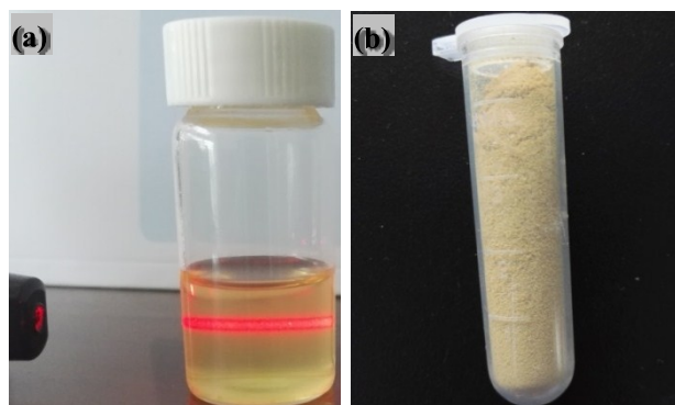
Fig. S11. Optical images of Co-LDHNS-II: (a) Tyndall effect of colloidal solutions and (b) about 100 mg of dried powders in 5 mL centrifuge tube.
