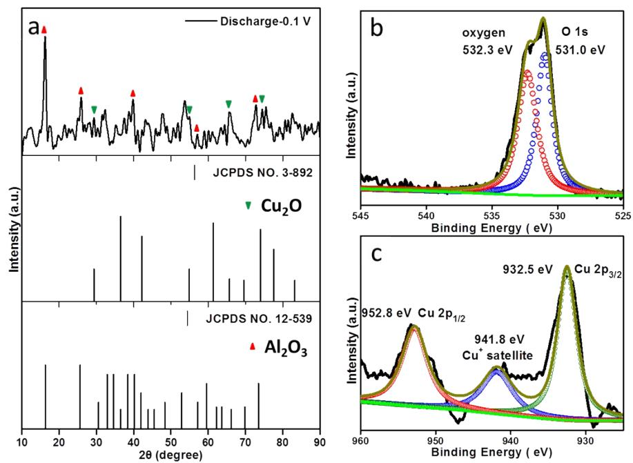
**Fig. S5** The XPS and XRD measurements of the cathode materials after 10 cycles after fully discharged to 0.1 V. (a) XRD pattern of the cathode. (b,c) XPS signals of Cu 2p and O 1s.
