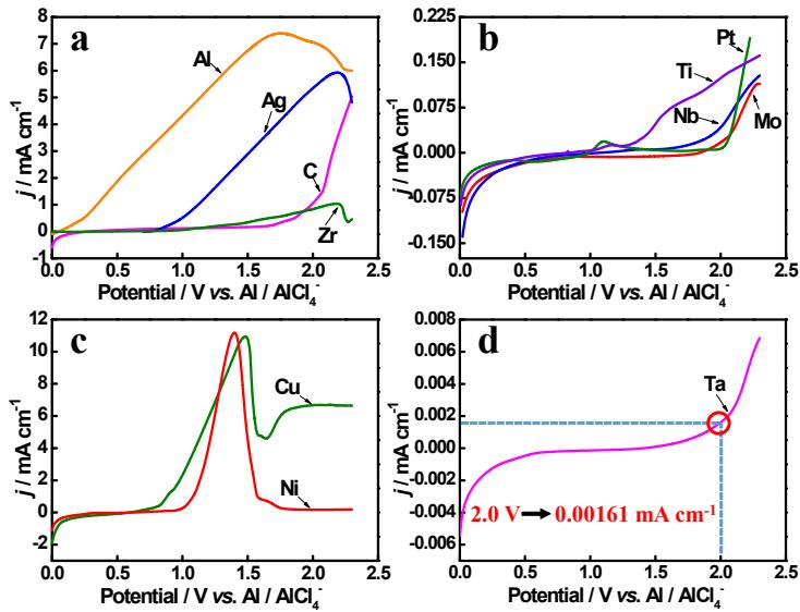
**Fig. S1** The polarization curves of various metallic and non-metallic current collectors in the  $\text{AlCl}_3/\text{[EMIm]Cl}$  ionic liquid electrolyte system. (a) Al, Ag, C and Zr. (b) Pt, Ti, Nb and Mo. (c) Cu and Ni. (d) Ta.
