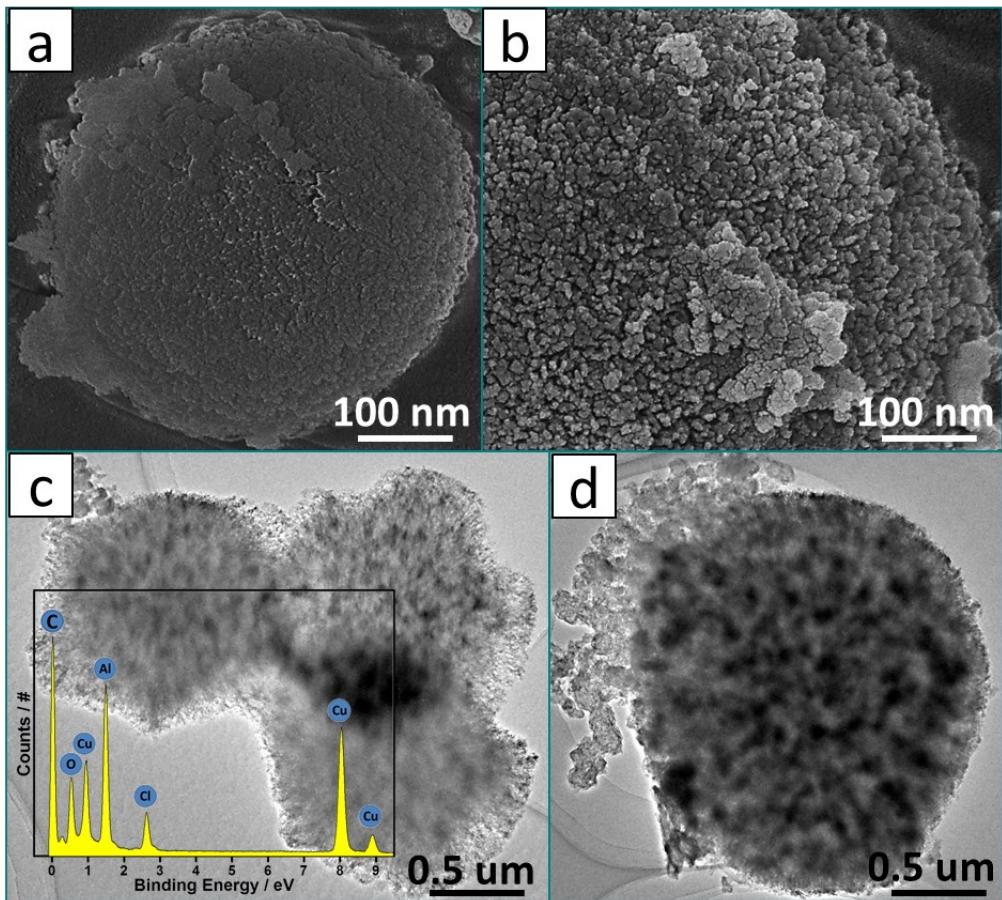
**Fig. S7** (a,b) SEM, and (c,d) TEM images of the PM-CuO after 100 cycles.
