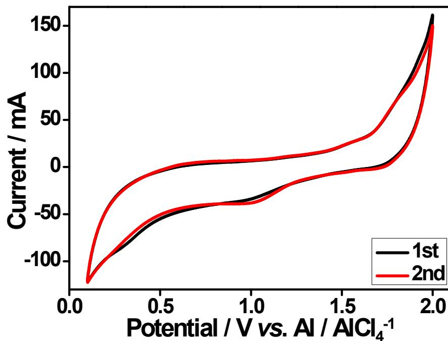
**Fig. S3** The typical CV curves of Al-Ta (cathode-Ta, anode-Al) performed in the voltage range of 0.1~2.0 V vs. Al/AlCl<sub>4</sub><sup>-</sup> at a scan rate of 1.0 mV s<sup>-1</sup>.
