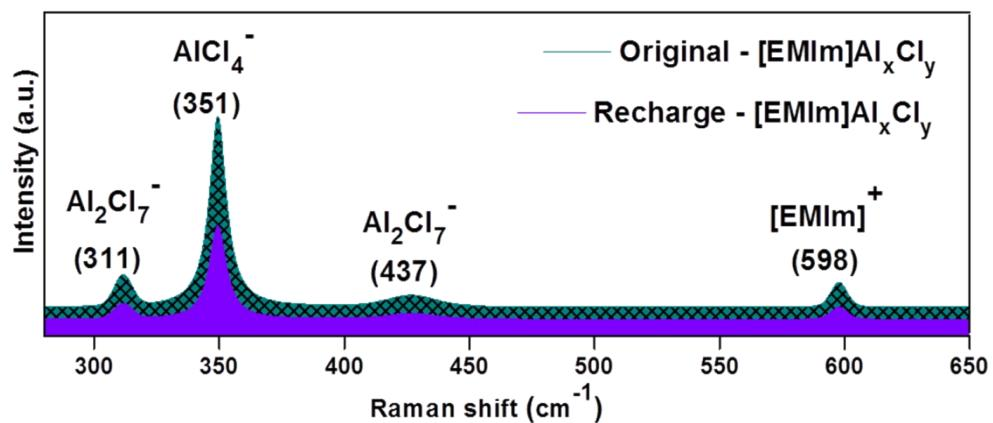
**Fig. S6** Raman spectra of the  $\text{AlCl}_3/\text{[EMIm]Cl}$  ionic liquid electrolytes with a mole ration of  $\text{AlCl}_3/\text{[EMIm]Cl}=1.3$  in different states.
