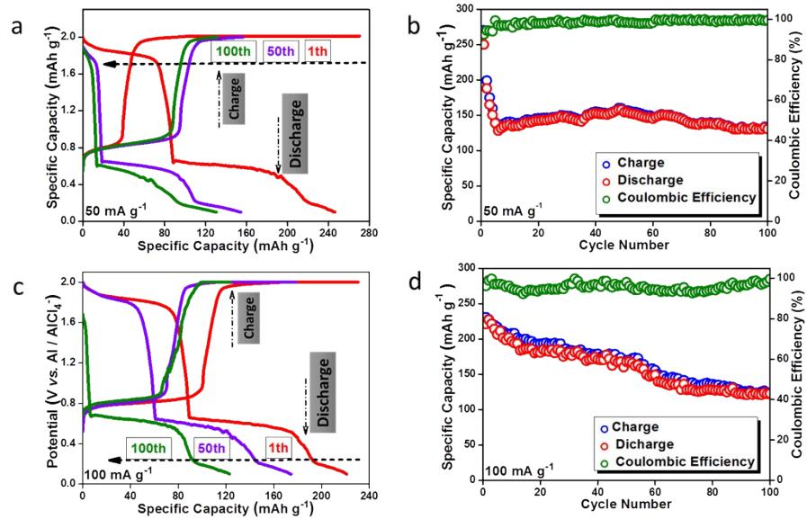
**Fig. S4** (a,b) The charge/discharge curves at the current densities of  $50 \text{ mA g}^{-1}$  from 1<sup>st</sup> to 100<sup>th</sup>, respectively. (c,d) The cycling performance at  $50$  and  $100 \text{ mA g}^{-1}$ .
