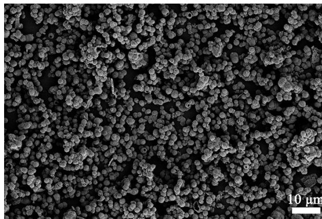
Fig. S3 Low magnification SEM image of NVPF.
