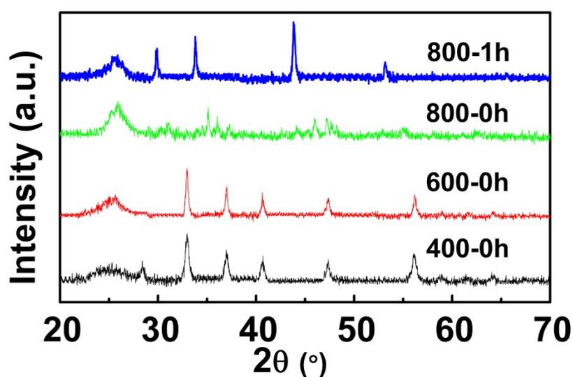
**Figure S5.** XRD patterns of the obtained products collected at different reaction temperature for different reaction time, (a) 400 °C 0 h, (b) 600 °C 0 h, (c) 800 °C 0 h, (d) 800 °C 1 h.
