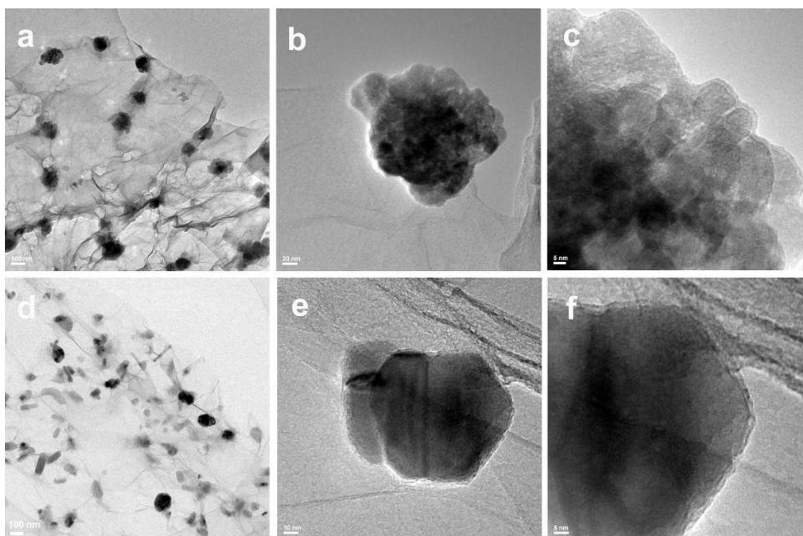
**Figure S1.** (a-c) TEM images of 3DG/FeS@C obtained at 400 °C; (d-f) TEM images of 3DG/FeS@C obtained at 600 °C.
