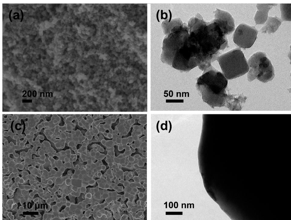
Figure S3. (a) SEM and (b) TEM images of pure PB nanoparticles; (c) SEM and (d) TEM images of FeS micro-sized particles.
