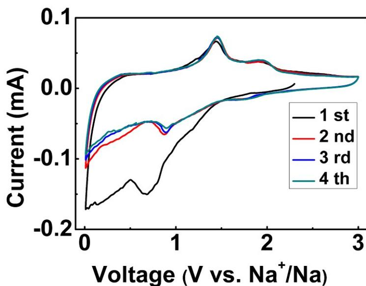
Figure S12. CV profiles of 3DG/FeS@C at a scan rate of  $0.1 \text{ mV s}^{-1}$ .
