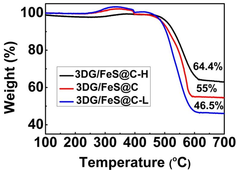
**Figure S6.** TGA curves of 3DG/FeS@C-H, 3DG/FeS@C, and 3DG/FeS@C-L at 10 °C /min in air flow.
