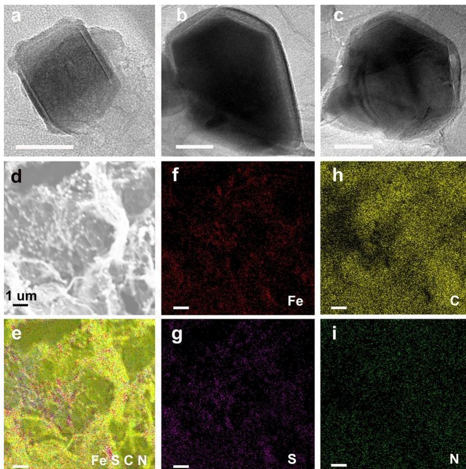
**Figure S4.** (a-c) Light-field TEM images of several FeS@C nanocomposites on 3DG. The scale bar is 50 nm. (d) SEM image of 3DG/FeS@C and corresponding Elemental mapping pictures of (e) Fe-S-C-N, (f) Fe, (g) S, (h) C and (i) N. The scale bar is 1 μm.
