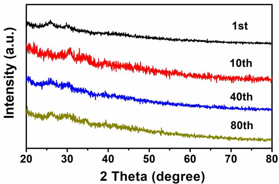
Figure S11. XRD pictures of 3DG/FeS@C at different charge cycles.
