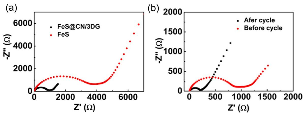
**Figure S14.** EIS plots of 3DG/FeS@C and FeS before cycle (a), and 3DG/FeS@C before and after cycle test (b).
