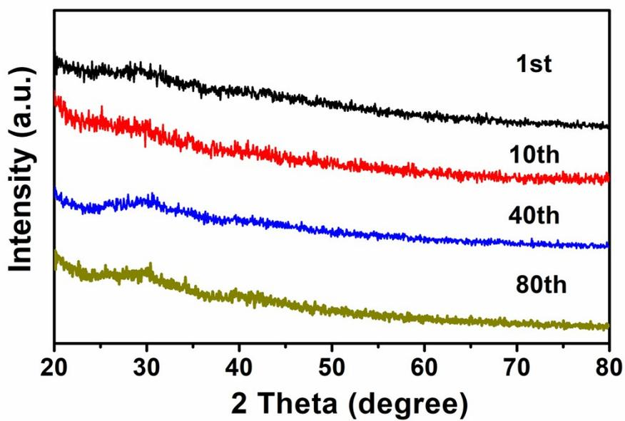
Figure S10. XRD pictures of 3DG/FeS@C at different discharge cycles.
