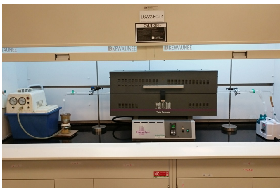
Fig. S1 Photograph of the home-built setup for ultrasonic aerosol spray. The setup used for the preparation of mesoporous metal oxide microspheres is composed of three parts from right to left: a household ultrasonic humidifier, a tube furnace and a sample collection system. In the ultrasonic humidifier, the precursor solution is atomized by the ultrasonic wave to
