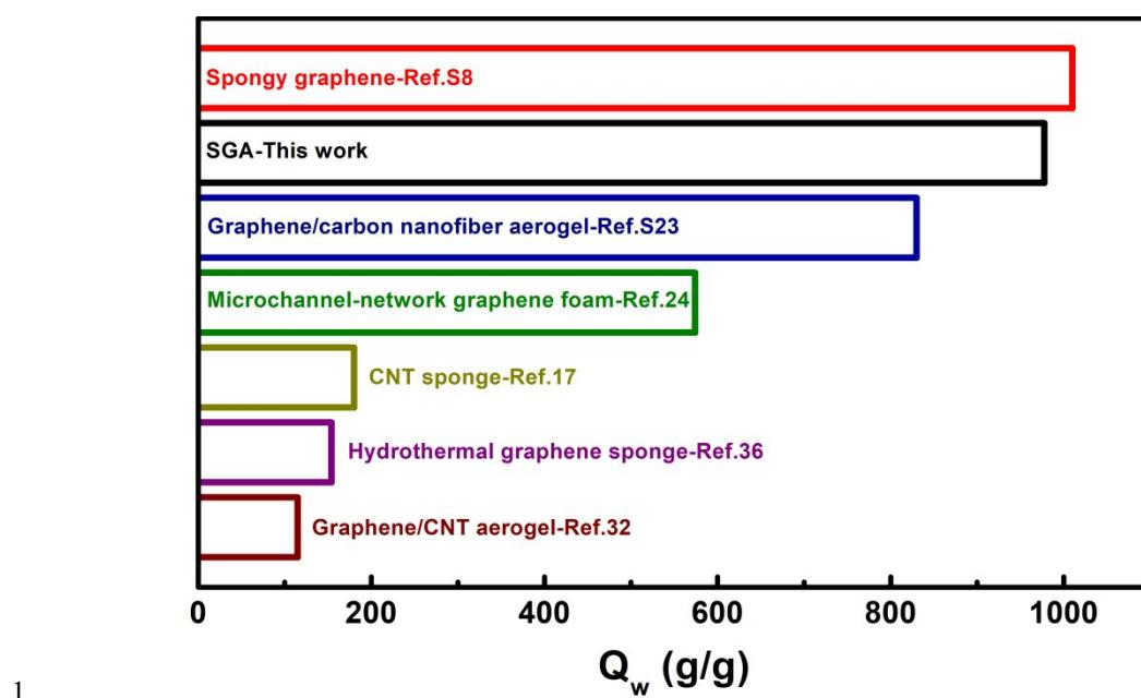
Fig. S10 A diagram of  $Q_w$  of various absorbents for chloroform.
