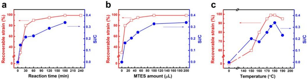
1 **Fig. S7** Recoverable strain and Si/C atom ratio of SGA with various reaction time (a,
