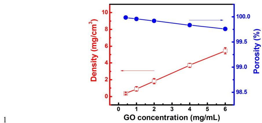
2 **Fig. S5** Density and porosity of SGA as a function of initial concentration of GO in the
