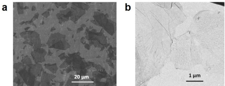
**Fig. S1** SEM (a) and TEM (b) images of GO sheets with a lateral size of  $\sim 20 \mu\text{m}$ .
