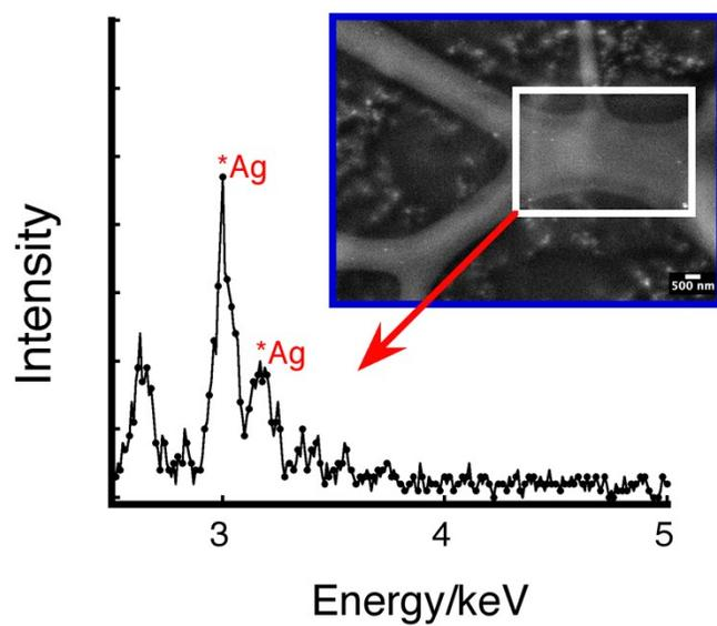
**Figure S3.** Representative EDS spectrum for a particular region, white rectangle, of collagen fibers containing spherical nanosilver. The inset in the figure corresponds to a scanning electron microscopy image for the fibers. Characteristic energy emissions for silver are indicated in the plot with red asterisks.
