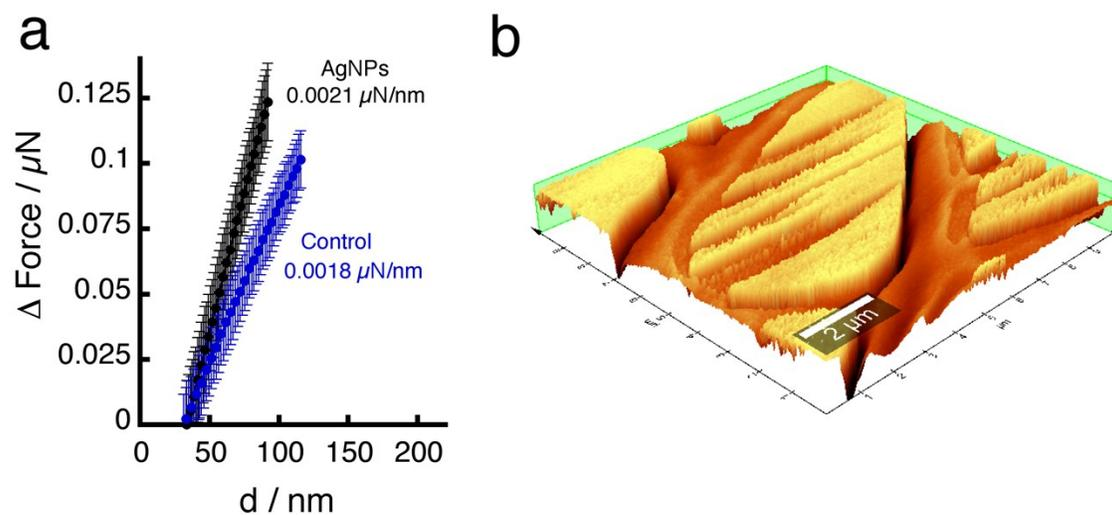
**Figure S4.** (a) Stiffness vs. displacement curves for collagen fibers (black) with and without nanosilver (blue) measured by atomic force microscopy (AFM). Error bars correspond to the standard deviation calculated from measuring 45 individual points from different random areas in the plot. (b) Representative image for collagen fibers prepared without nanosilver. False color scale represents differences in maximum force, being higher for areas shown with darkest color intensities.
