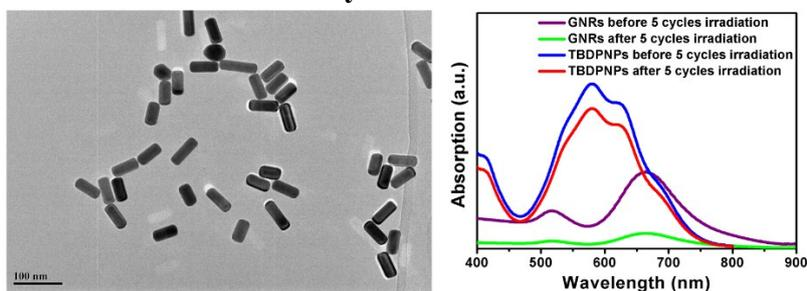
Figure S2. The TEM image of GNRs (left) and the comparison of thermal stability between GNRs and TBDPNPs (right).
