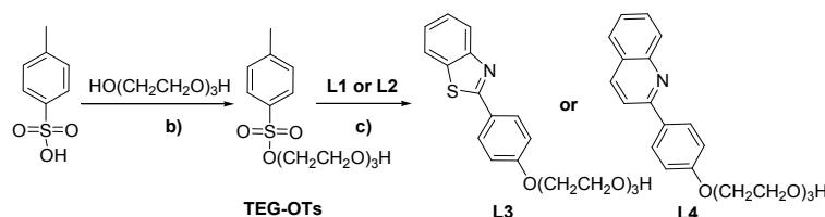
**Scheme S2.** Synthetic route of the ligands L3 and L4. Conditions: (b) pyridine, DCM,  $0^\circ\text{C}$ ; (c) Tetrabutyl ammonium bromide,  $\text{K}_2\text{CO}_3$ ,  $\text{CH}_3\text{CN}$ , reflux  $80^\circ\text{C}$
