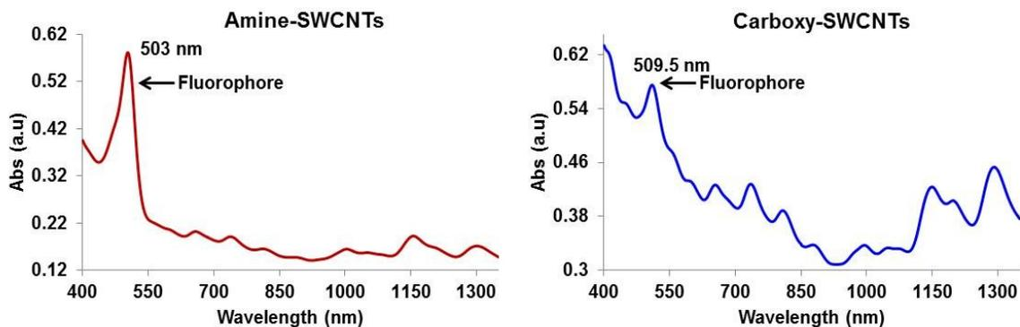
**Figure S3.** UV-Vis-near-infrared (NIR) absorption spectra of fluorophore -polymer-SWCNT complexes in water, showing peaks from fluorophore (fluorescein was conjugated to amine-SWCNTs and Alexa 488 was conjugated to carboxy-SWCNTs) and SWCNTs.
