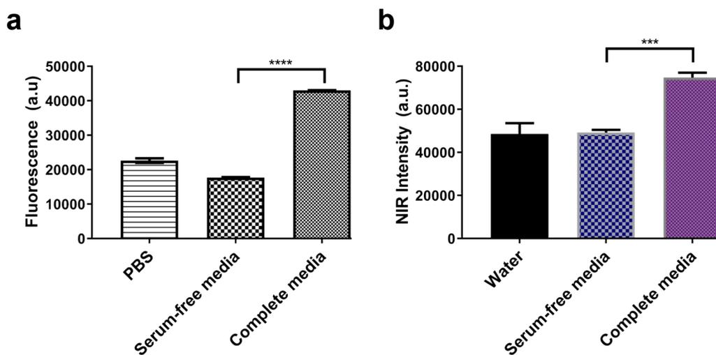
**Figure S6.** Effect of cell culture media on carboxy-SWCNTs emission. **a)** Visible fluorescence from Alexa 488/fluorescein on the polymer-nanotube complexes. **b)** NIR fluorescence of carbon nanotubes on the complexes (concentration = 0.8 mg/L). A phenol red-free media was used in panel a (nanotube concentration = 2 mg/L).
