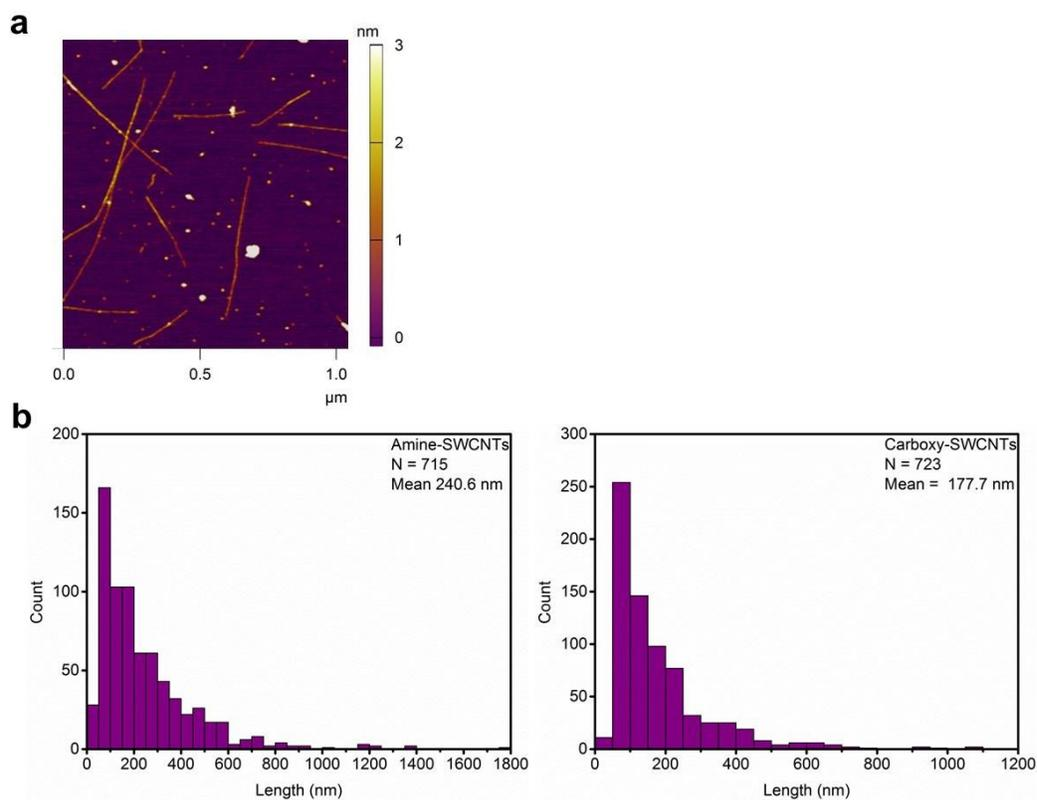
**Figure S2.** Atomic force microscopy (AFM) of polymer-SWCNTs. **a)** Representative AFM micrograph of Amine-SWCNTs. **b)** Length distribution of the samples as quantified from AFM images of amine-SWCNTs (left) and carboxy-SWCNTs (right).
