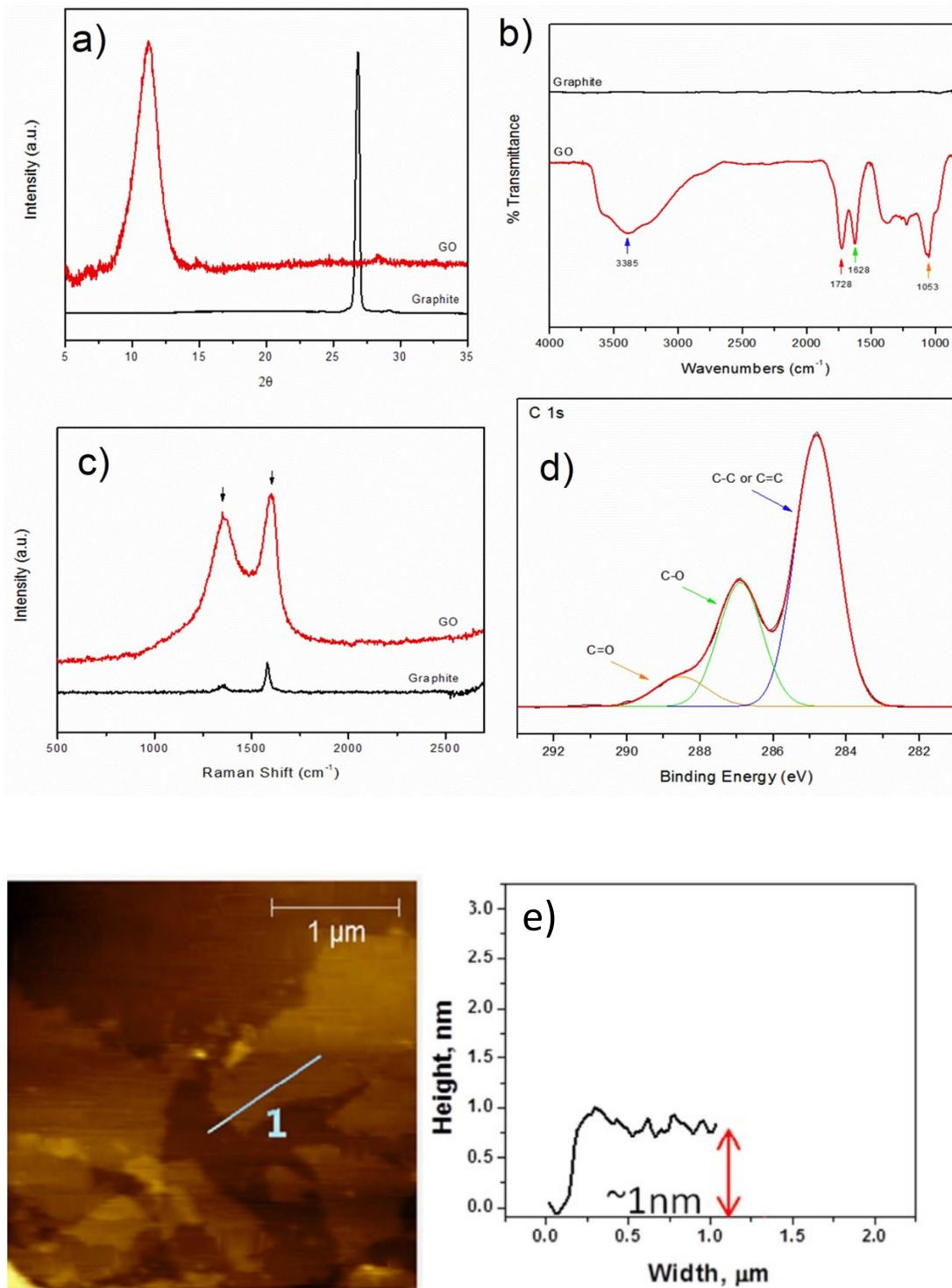
**Fig. S1:** a) XRD spectrum showing the peak 2 theta at 11.25 (representative of GO peak); b) FTIR with characteristic peaks of GO functional groups (-C-OH, -C=O, -COOH and -C-O); c) Raman spectrum showing 1350 (cm<sup>-1</sup>) for functional group in GO; d) XPS with GO bonding for the functional groups and e) AFM analysis of GO showing the height ~ 1nm.
