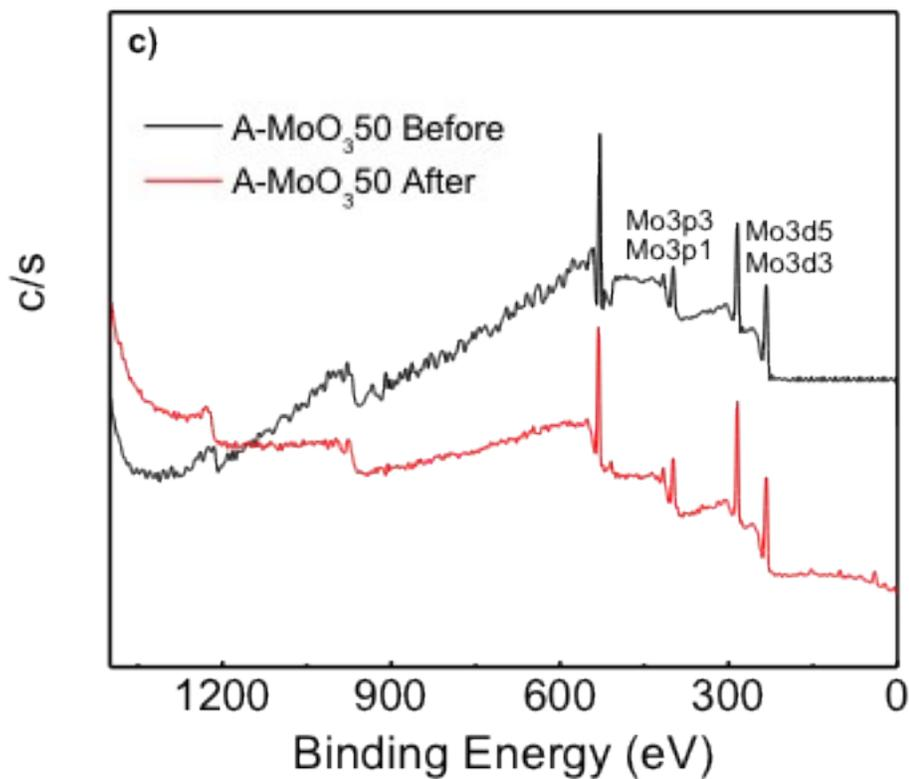
**Fig. S4:** FTIR of C-PEI75 (a), XPS spectrum of C-PEI75 (b) and XPS of A-MoO<sub>3</sub>50 (c) before and after leaching process showing there was no significant changes of the samples in term of compositions.
