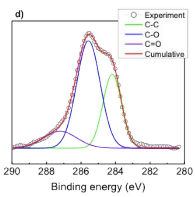
**Fig. S12:** XPS spectra of the coatings: adhesive A only and A-MoO<sub>3</sub>50 (adhesive A with 50% *h*-MoO<sub>3</sub>) which showing the presence of Mo on the coated surface indicating the presence of MoO<sub>3</sub> and adhesive (a). The high resolution of C1s for adhesive A only (b), Mo<sup>6+</sup> (c) and C1s of A-MoO<sub>3</sub>50 (d) were expressed in this figure.
