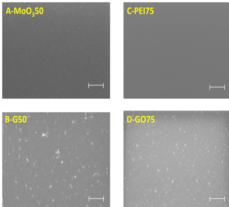
**Fig. S5:** SEM images of the antimicrobial coatings after 24h leaching. Scale bar 1 μm.
