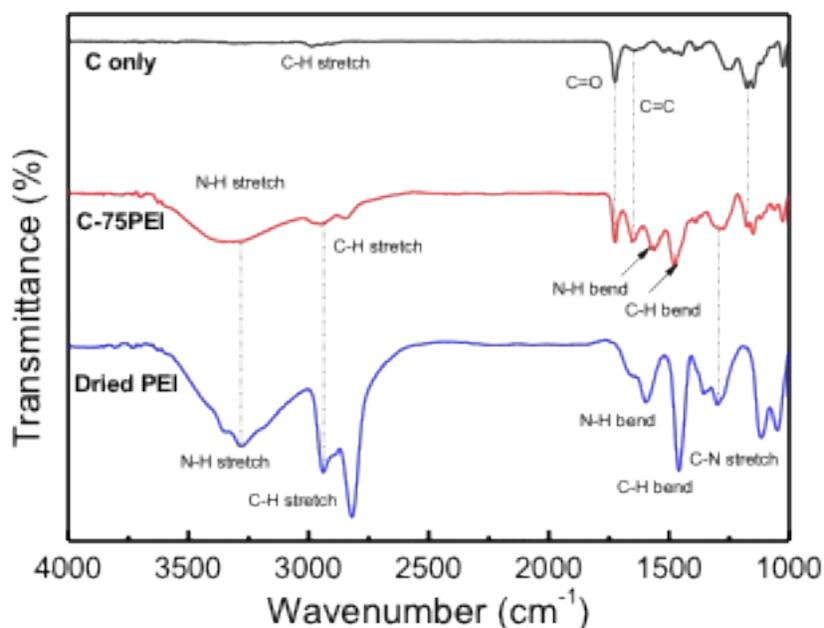
**Fig. S11:** FTIR spectra of successful coating of dried PEI, C and C-PEI75 showing the essential functional groups of PEI and adhesive on the surface of the coating.
