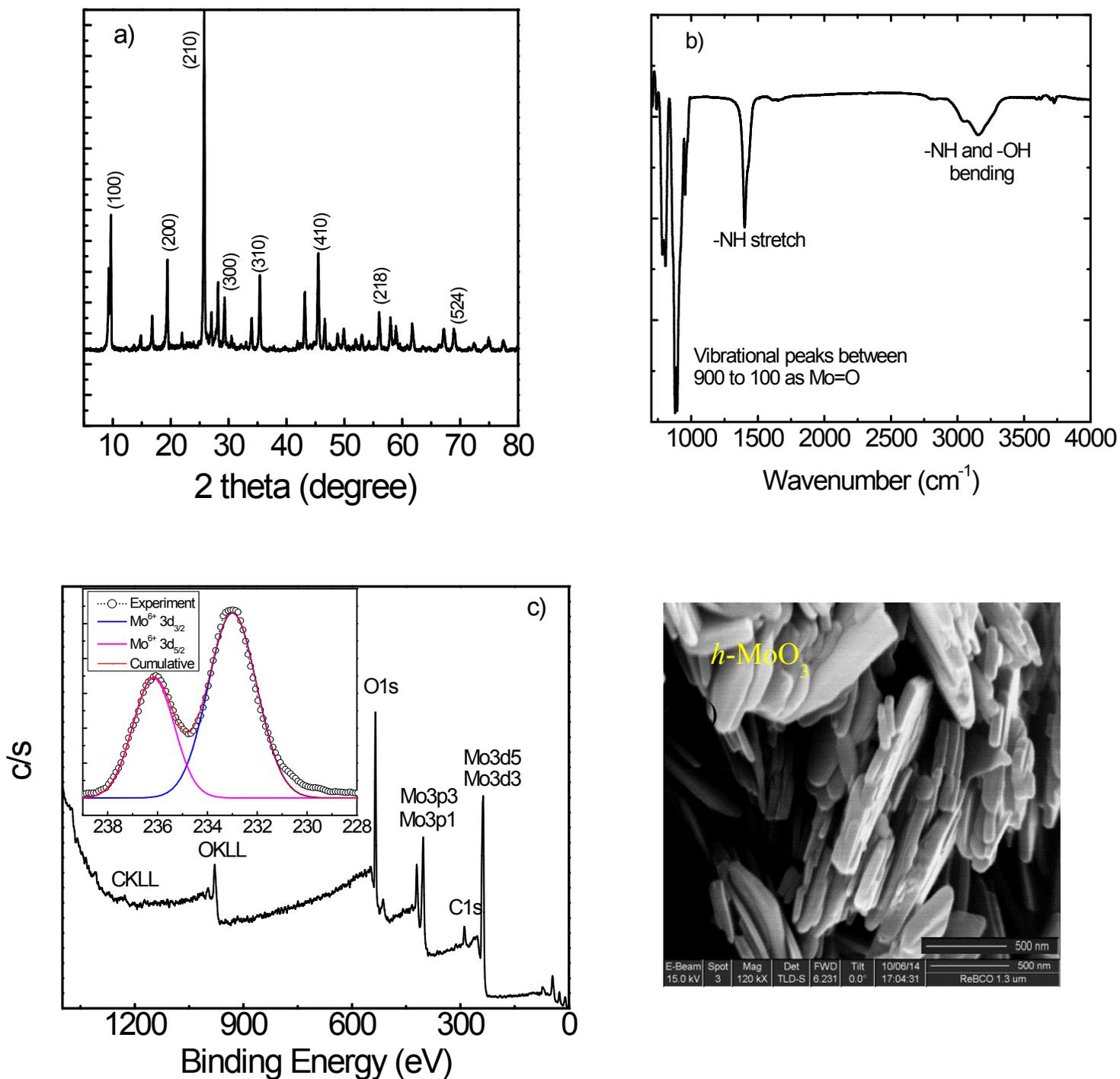
**Fig. S2:** (a) X-ray diffraction (XRD) spectra of  $h$ - $\text{MoO}_3$  the spectra confirmed the successful synthesis of both  $\text{MoO}_3$  structure with the characteristic peaks<sup>1</sup> (b) FTIR spectra of  $\text{MoO}_3$  ( $h$ - $\text{MoO}_3$ ) with the spectra matched where Mo in the previous publication in  $\text{MoO}_3$ <sup>2</sup> and (c) X-ray photoelectron spectroscopy (XPS) spectrum and (d) Scanning Electron Microscope (SEM) image of  $h$ - $\text{MoO}_3$
