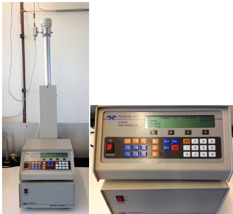
Figure S2: ISCO 260D® pump with one cylinder and LCD control unit.
