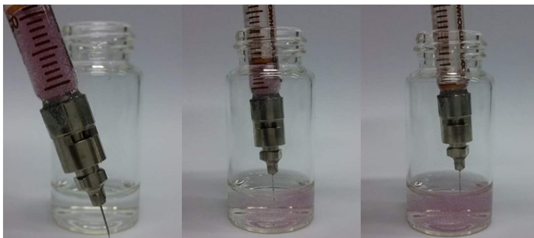
Figure S15. The injectability of \text{PCL}_{2k}\text{@PGNP}_{0.5\%} microspheres dispersed in an aqueous solution with 26 gauge needle.
