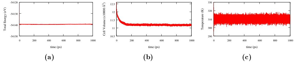
**Figure S8:** Solution I: (a) Total energy vs simulation time, (b) cell volume vs simulation time and (c) temperature vs simulation time during the first ns of production run in an NPT ensemble.
