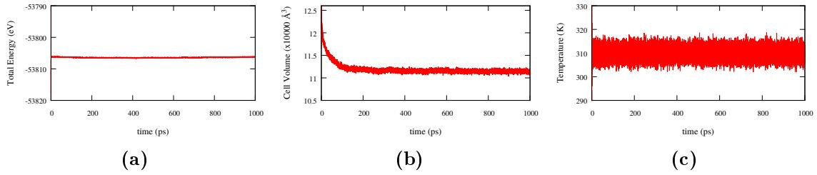
**Figure S11:** Solution I(a): (a) Total energy vs simulation time, (b) cell volume vs simulation time and (c) temperature vs simulation time during the first ns of production run in an NPT ensemble.
