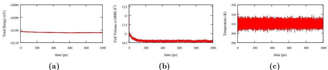
**Figure S13:** Solution III(a): (a) Total energy vs simulation time, (b) cell volume vs simulation time and (c) temperature vs simulation time during the first ns of production run in an NPT ensemble.
