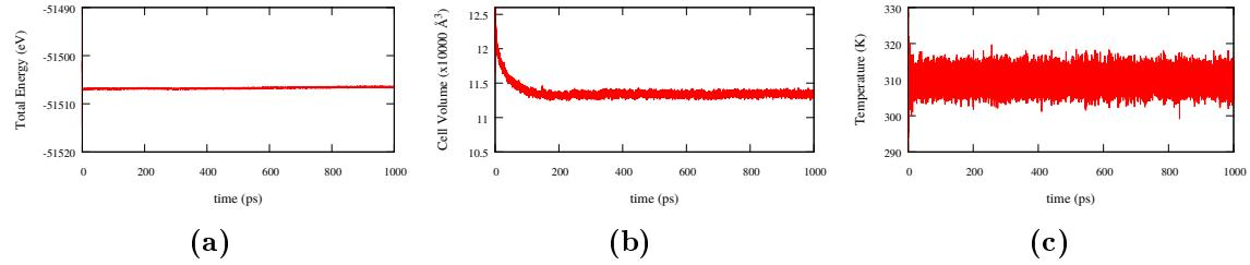
**Figure S9:** Solution II: (a) Total energy vs simulation time, (b) cell volume vs simulation time and (c) temperature vs simulation time during the first ns of production run in an NPT ensemble.
