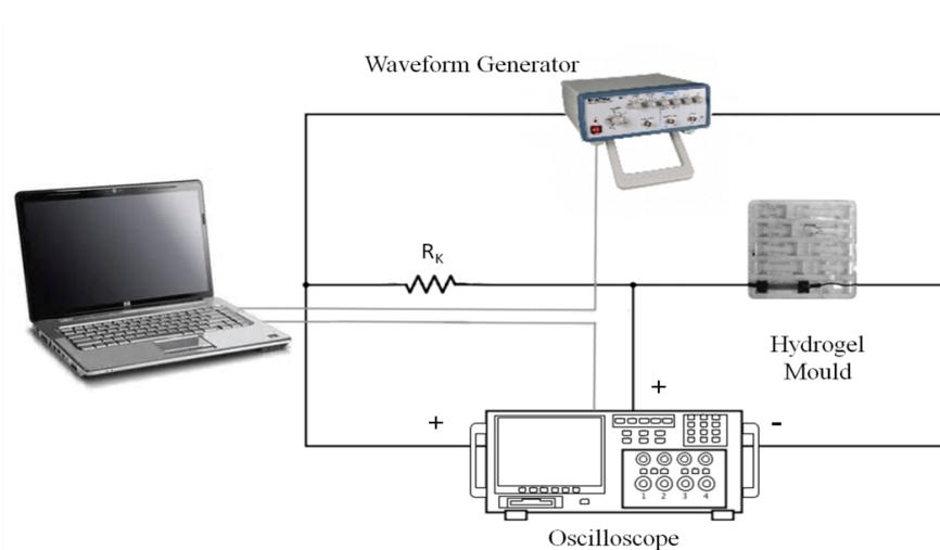
**Figure S1** Schematic representation of the custom designed impedance analyser,  $R_k$  is a known resistor.
