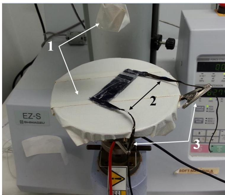
**Figure S2** Setup for analysis of capacitive pressure sensor. **1.** Duct tape is used to insulate compressive plates. **2.** Carbon fibre used to connect hydrogel to multimeter clips. **3.** Alligator clips to connect the device to digital multimeter.
