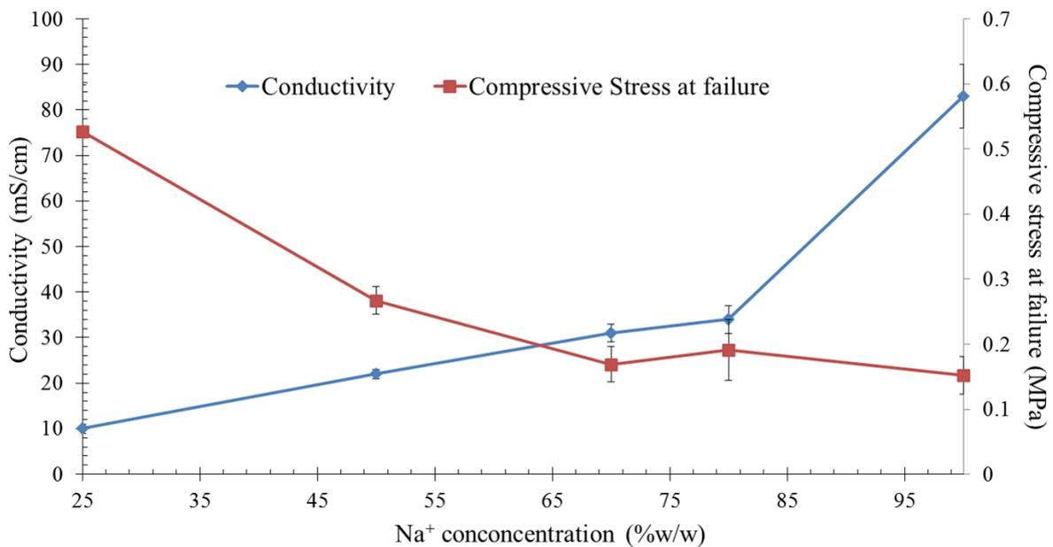
**Figure S3** Summary of conductivity and compressive stress at failure as a function  $\text{Na}^+$  %w/w concentration at 21°C. Data from Table 5.
