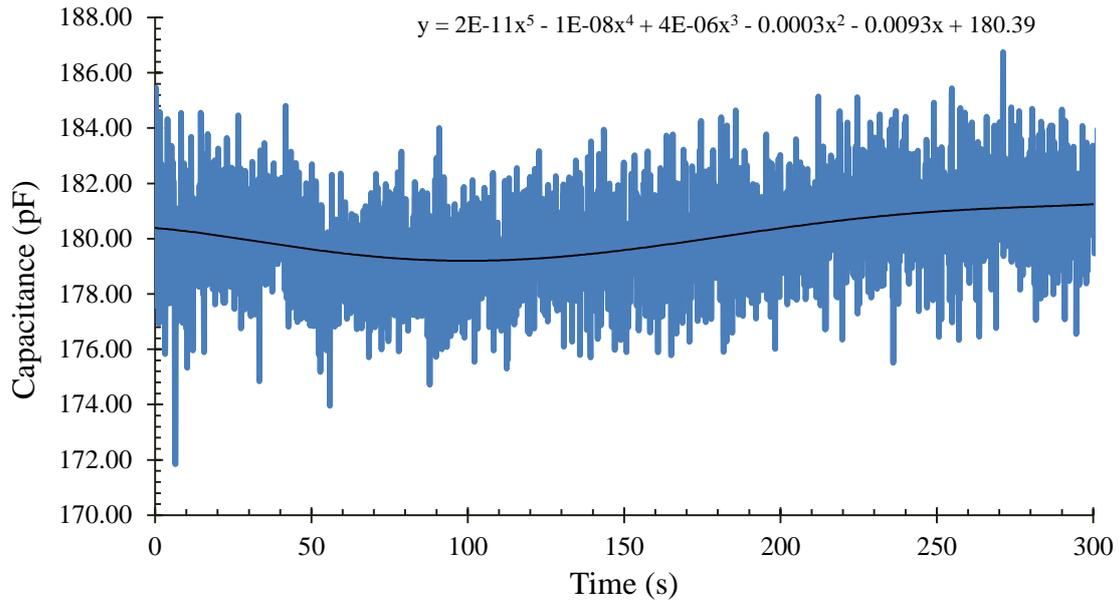
**Figure S4:** Capacitance reading of a typical sensor under ambient conditions with no applied force.
