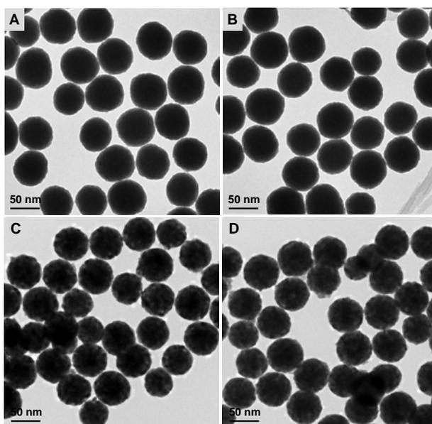
**Figure S2.** TEM images of monodispersed (A) NaF-doped Gd<sub>2</sub>O<sub>2</sub>S:Tb with protective layer, (B) NaF-doped Y<sub>2</sub>O<sub>2</sub>S:Yb/Tm with protective layer, (C) Gd<sub>2</sub>O<sub>2</sub>S:Tb without NaF doping, (D) Y<sub>2</sub>O<sub>2</sub>S:Yb/Tm without NaF doping.
