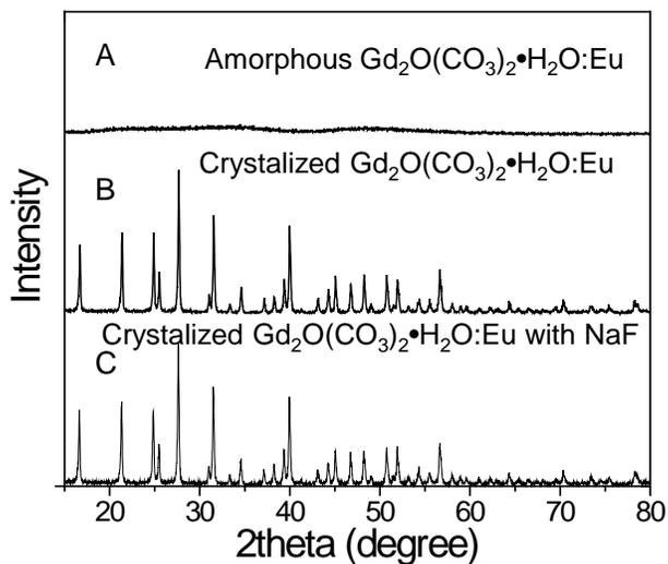
**Figure S1.** XRD powder patterns of (A) Gd<sub>2</sub>O(CO<sub>3</sub>)<sub>2</sub>•H<sub>2</sub>O:Eu, (B) crystallized Gd<sub>2</sub>O(CO<sub>3</sub>)<sub>2</sub>•H<sub>2</sub>O:Eu during annealing in the glycerol, (C) crystallized Gd<sub>2</sub>O(CO<sub>3</sub>)<sub>2</sub>•H<sub>2</sub>O:Eu with encapsulated NaF during annealing in the glycerol.
