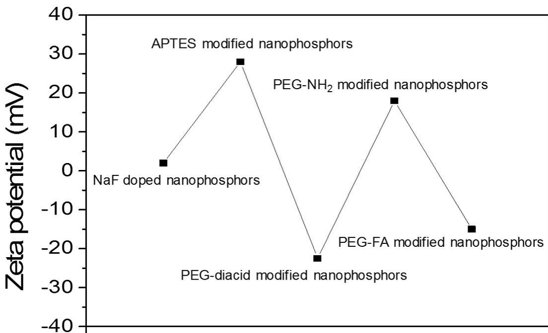
**Figure S11.** Zeta potential of the nanophosphors at different stages of surface modification.
