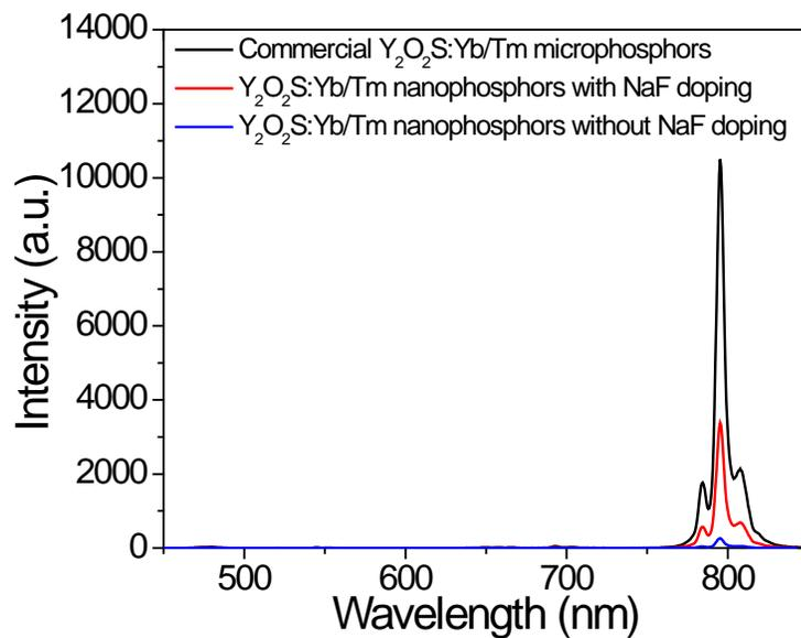
**Figure S6.** Comparison of upconversion luminescence of different types of  $Y_2O_2S:Yb/Tm$  phosphors (0.25 mg/mL).
