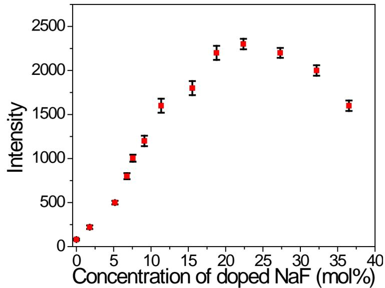
**Figure S5.** Effect of NaF-doping concentration on the X-ray excited optical luminescence intensity at 620 nm for  $Gd_2O_2S:Eu$  nanophosphors.
