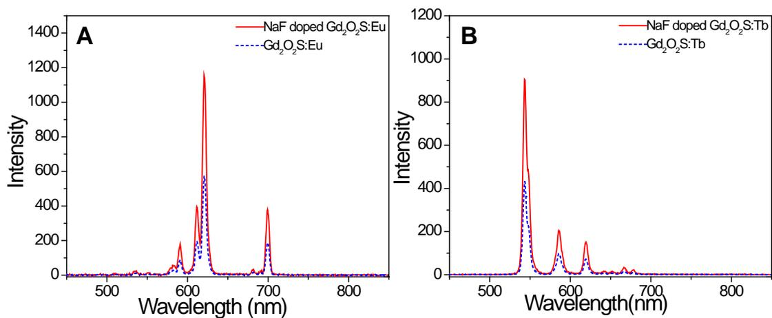
**Figure S4.** Fluorescence emission spectra, using 480 nm excitation, for (A) Gd<sub>2</sub>O<sub>2</sub>S:Eu with and without 7.6 mol% NaF doping and (B) Gd<sub>2</sub>O<sub>2</sub>S:Tb with and without 7.6 mol% NaF doping.
