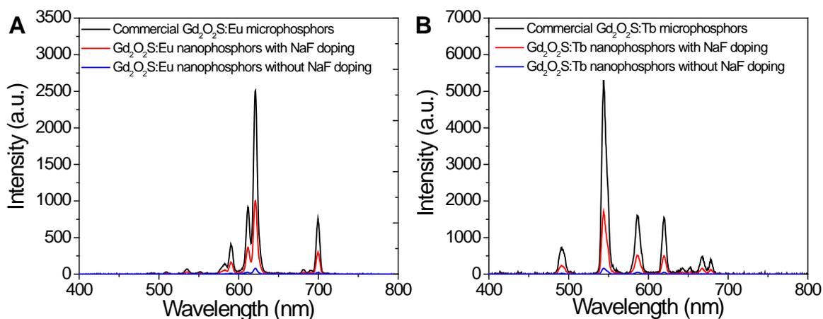
**Figure S3.** Comparison of X-ray excited luminescence of different types of (A) Gd<sub>2</sub>O<sub>2</sub>S:Eu phosphors (1 mg/mL) and (B) Gd<sub>2</sub>O<sub>2</sub>S:Tb (1 mg/mL).
