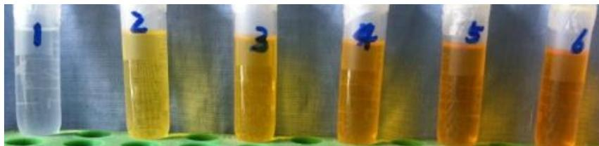
**Figure S10.** The colors for different concentrations of HD solution containing acetic acid and ethanol (No.1-No.6 from left to right)
