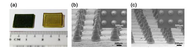
**Fig. S1. (a)** Photograph of a 3D printed template and of the resulting suckerin microneedle array. **(b)** SEM micrograph of 3D printed template microneedles. The inset shows the top view of the microneedles. **(c)** SEM micrograph of suckerin microneedles prepared from the 3D printed template. The inset shows the top view of the microneedles.
