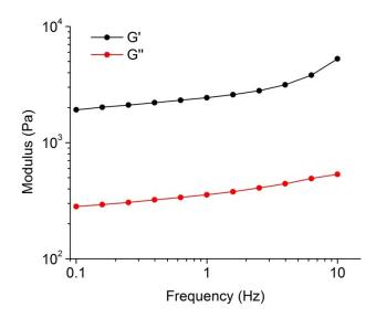
**Fig. S3.** Mechanical properties (measured by rheometry) of suckerin microneedle arrays incubated in 2M urea solution. The sample was initially measured by amplitude-sweep to identify the viscoelastic regime. Subsequently the frequency-sweep measurements were done at 0.5% strain.
