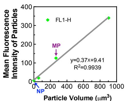
Figure S2. The linear relationship between the fluorescence intensity and the volume of chitosan particles. Particles at a size range from nano to micro were prepared and tested. Comparative data for NP (400 nm) and MP (8 µm) were highlighted by the arrows.
