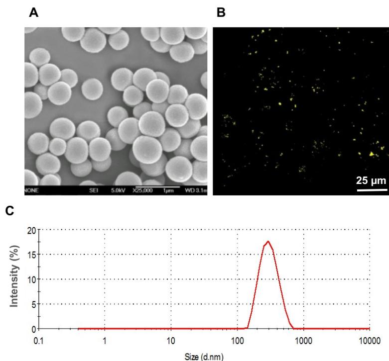
Figure S1. SEM image (A), confocal image (B) and the size distribution (C) of the nanoparticles (400 nm).
