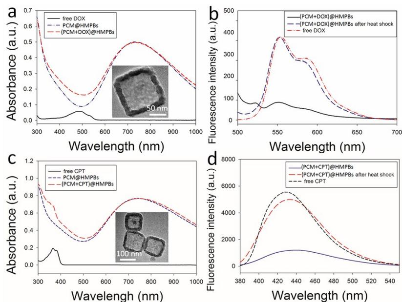
**Fig. S6** a) UV-vis-NIR spectra of free DOX, PCM@HMPBs and (PCM+DOX)@HMPBs (inset: TEM image of (PCM+DOX)@HMPBs); b) fluorescent spectra of free DOX and (PCM+DOX)@HMPBs before and after methanol treatment; c) UV-vis-NIR spectra of free CPT, PCM@HMPBs and (PCM+CPT)@HMPBs (inset: TEM image of (PCM+CPT)@HMPBs); d) fluorescent spectra of free CPT and (PCM+CPT)@HMPBs before and after methanol treatment.
