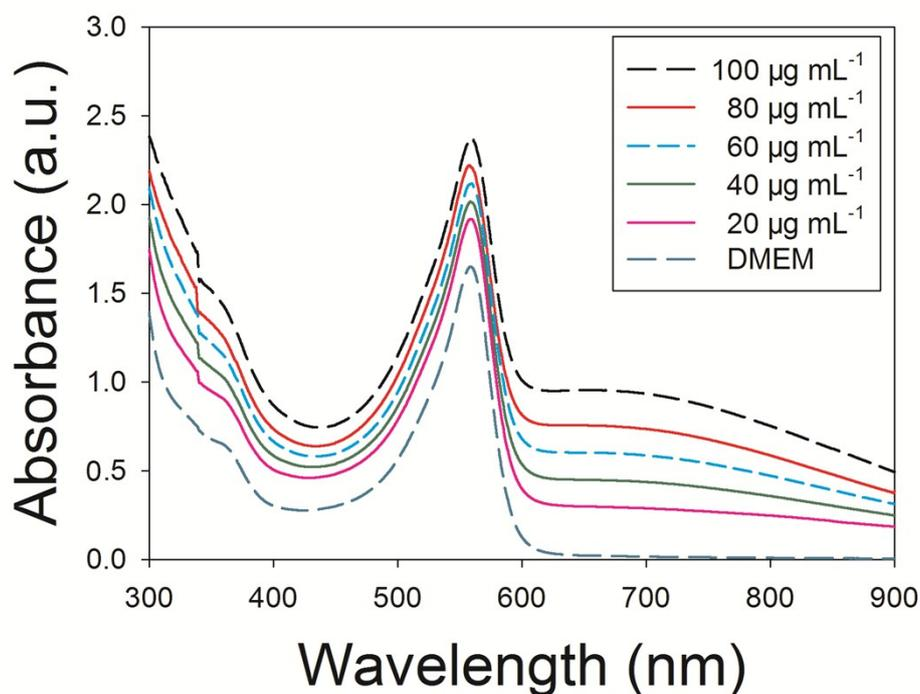
**Fig. S1** UV-vis-NIR spectra of PCM@HMPBs dispersed in DMEM cell culture medium with a test background of DI water
