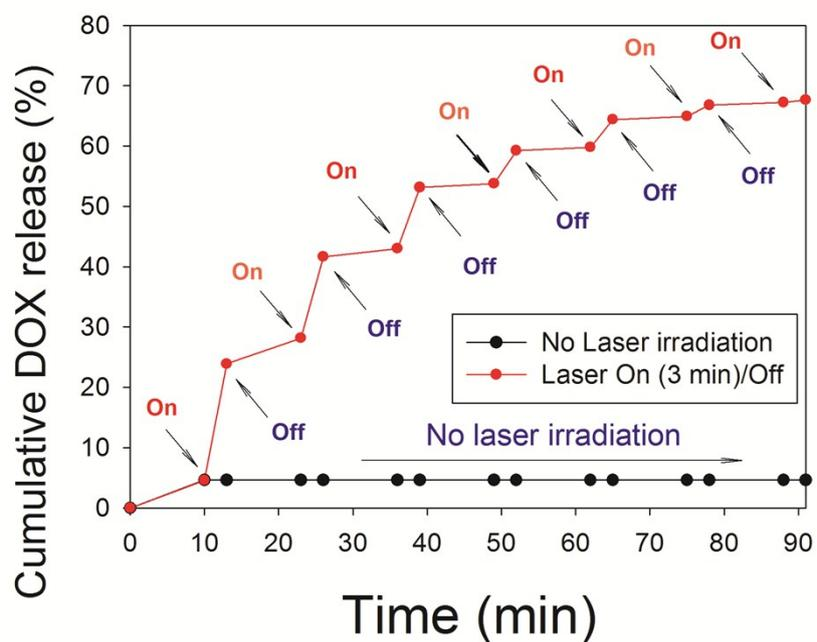
**Fig. S9** The “on” and “off” switch of DOX release profiles of (PCM+DOX)@HMPBs under NIR light irradiation (808 nm, 2.0 W).
