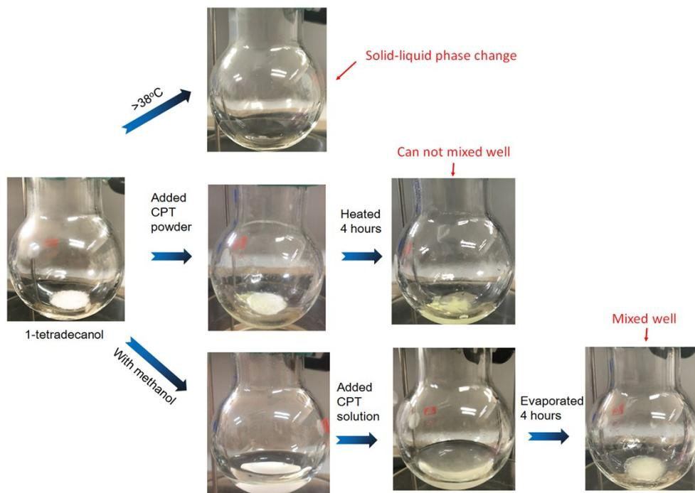
**Fig. S5** Miscible property of 1-tetradecanol and hydrophobic CPT.
