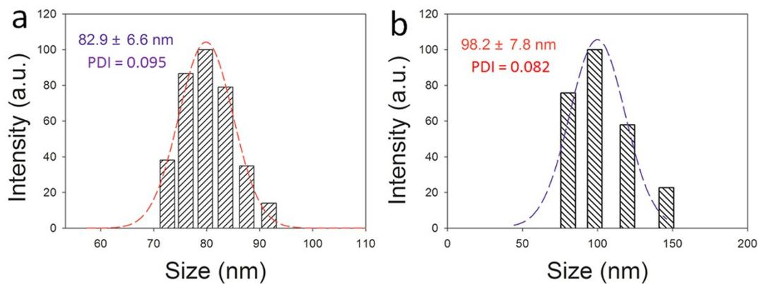
**Fig. S2** Diameter distribution of a) HMPBs and b) PCM@HMPBs in DI Water from DLS test.
