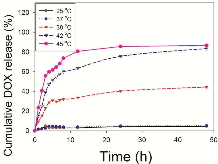
**Fig. S7** Thermo-responsive release profiles of DOX from (PCM+DOX)@HMPBs at different temperatures.
