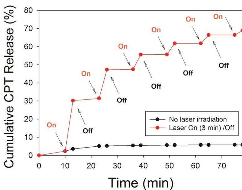
**Fig. S10** The “on” and “off” switch of CPT release profiles of (PCM+CPT)@HMPBs under NIR light irradiation (808 nm, 2.0 W).
