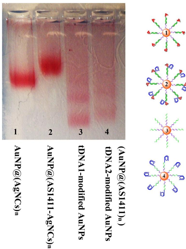
**Figure S4.** Agarose gel electrophoresis image of DNA-modified AuNPs before and after assembling with DNA-templated AgNCs.
