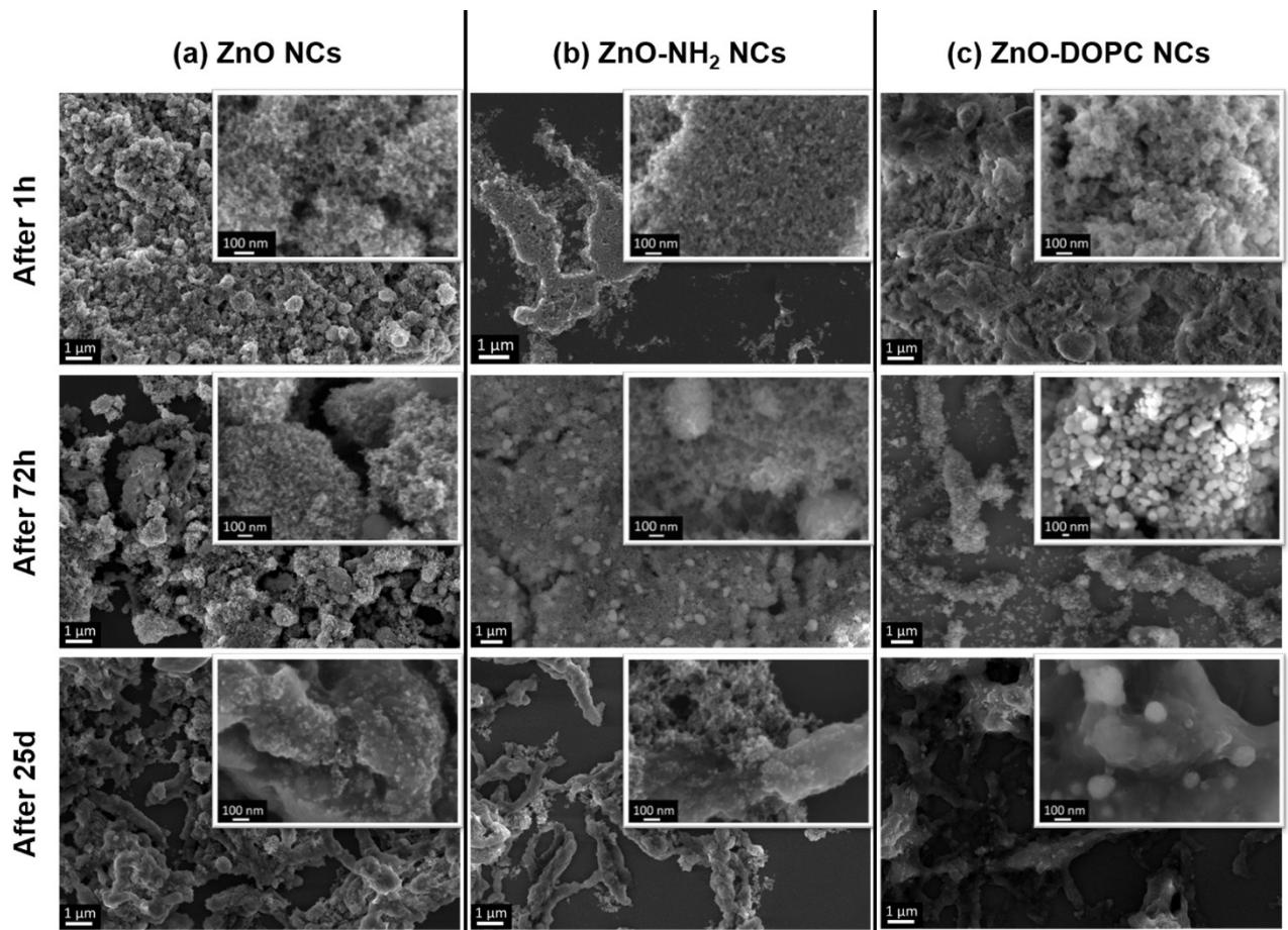
**Figure S5.** FESEM images of the biostability behavior of the three ZnO nanocrystals: (a) pristine ZnO, (b) amine-functionalized ZnO, (c) lipid-shell functionalized ZnO NCs, after different assay times (1 h, 72 h and 25 days) in EMEM.
