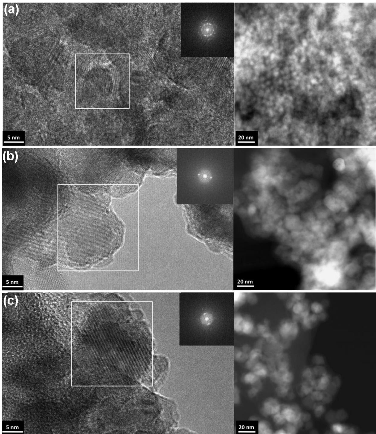
**Figure S7.** TEM with a FFT in the inset (left) and STEM (right) images of the ZnO-DOPC NCs (a) before, and after 25 days of contact with (b) SBF and (c) EMEM solutions still showing the nano-spherical shape of each NC and a smooth matrix around each of them attributed to the presence of phospholipids.
