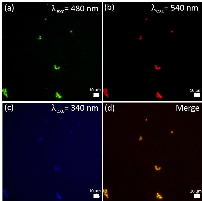
**Figure S3.** Wide-Field fluorescence microscopy image of the (a) green channel, with the lipid shell labeled by Bodipy, (b) red channel, with the ZnO-NH<sub>2</sub> labeled with Atto550, (c) self-fluorescence of the ZnO NCs exited at 340 nm, (d) co-localization image of the all merged channels.
