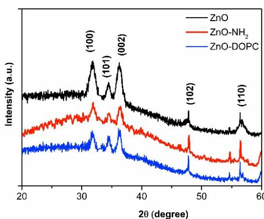
**Figure S1.** Representative X-Ray diffractogram of the ZnO nanocrystals: pristine (black curve), with amino-propyl functional groups (red curve) and coupled with DOPC lipids (blue curve). Non-indexed peaks derive from the silicon wafer used as substrates.
