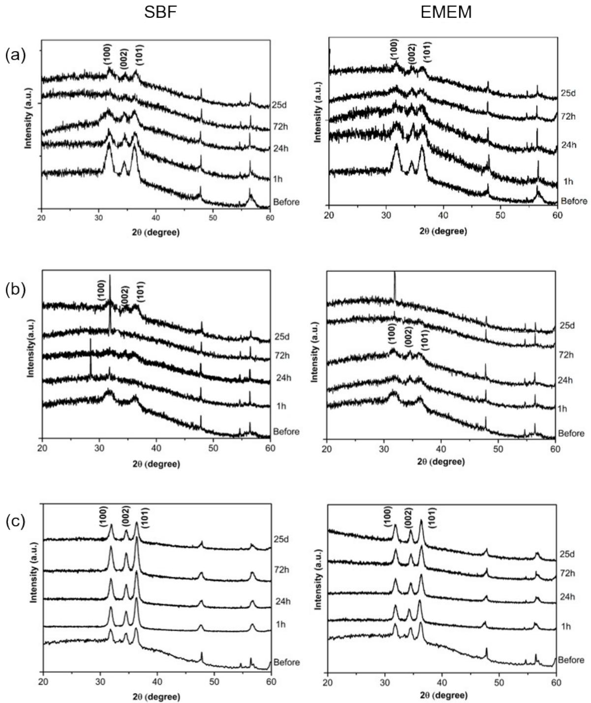
**Figure S6.** X-ray diffraction patterns of (a) ZnO NCs, (b) ZnO-NH<sub>2</sub> NCs and (c) ZnO-DOPC NCs at different time points during the biostability assays in SBF and EMEM.
