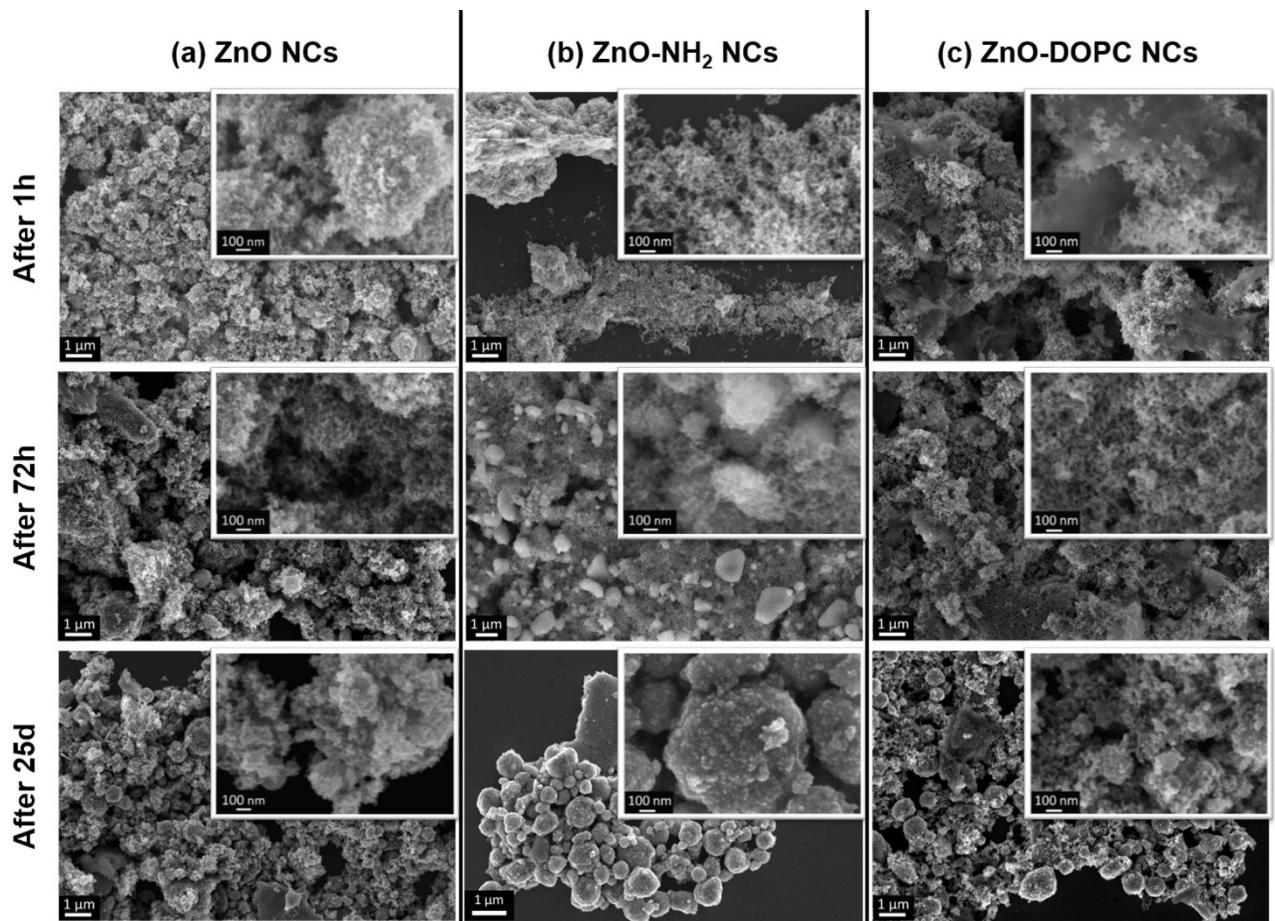
**Figure S4.** FESEM images of the biostability behavior of the three ZnO nanocrystals: (a) pristine ZnO, (b) amine-functionalized ZnO, (c) lipid-shell functionalized ZnO NCs, after different assay times (1 h, 72 h and 25 days) in SBF.
