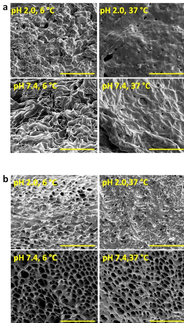
**Figure S4.** SEM micrographs of (a) FA0 and (b) FA50 hydrogels at different conditions.
