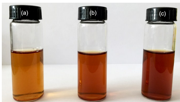
Fig. S5 Photograph of aqueous dispersions (a) GO, (b) rGO/ \beta -CD, and (c) rGO/ \beta -CD/ C_{60} (50 \mu g/mL ).
