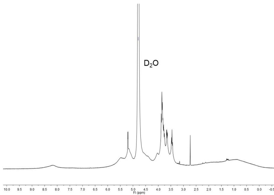
**Figure S39.** <sup>1</sup>H NMR spectrum of trehalose linear homo-glycopolymer (**13f**) in D<sub>2</sub>O.
