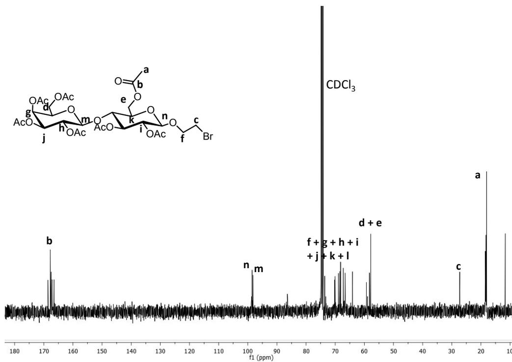
Figure S20. <sup>13</sup>C NMR spectrum of 2'-bromoethyl peracetylated lactose (**4**) in CDCl<sub>3</sub>.
