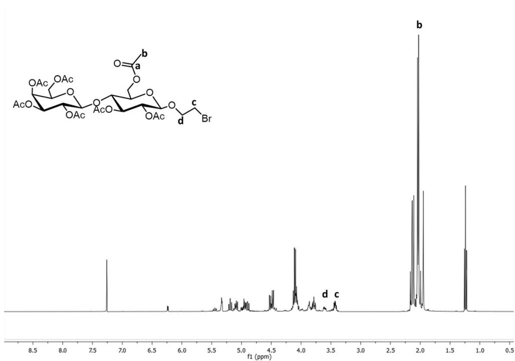
Figure S19. <sup>1</sup>H NMR spectrum of 2'-bromoethyl peracetylated lactose (**4**) in CDCl<sub>3</sub>.
