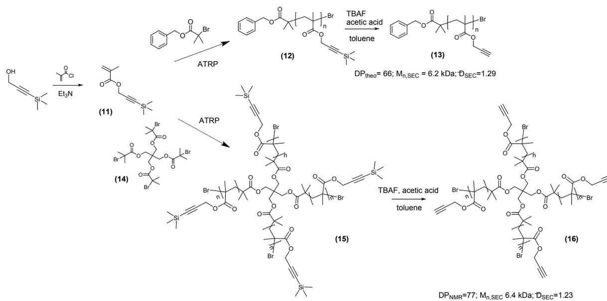
**Scheme S7.** Synthetic route to 3-trimethylsilyl-propargyl methacrylate monomer **(11)** and the corresponding linear **(13)** and star polymers **(16)**.
