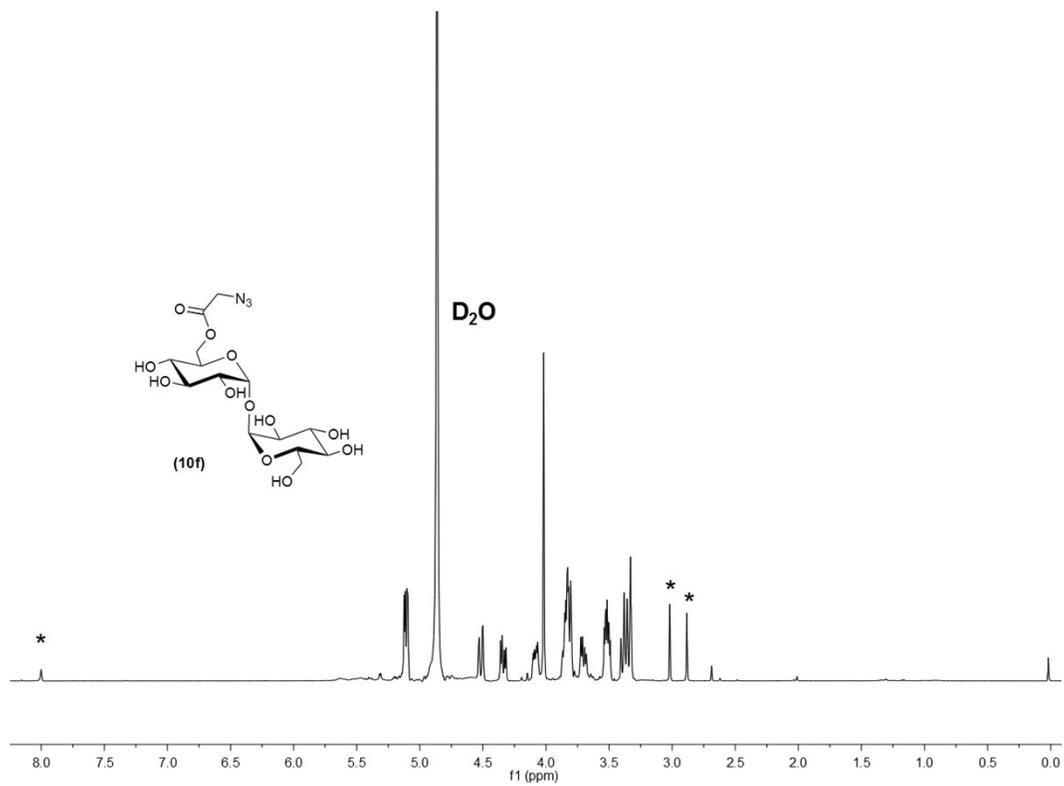
**Figure S27.**  $^1\text{H}$  NMR spectrum of trehalose azide (**10f**) in  $\text{D}_2\text{O}$ .
