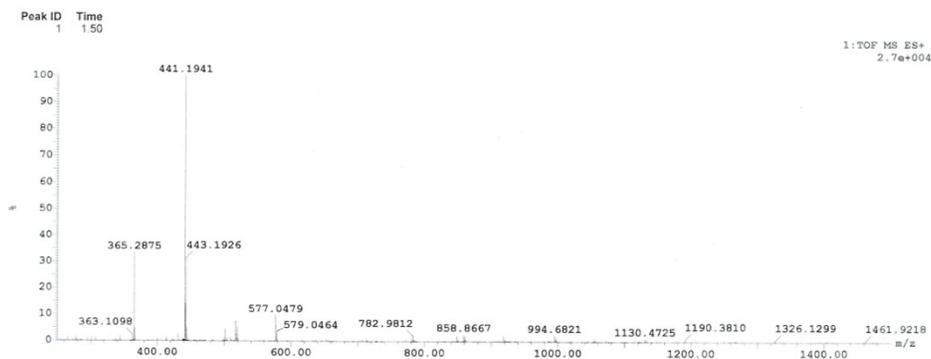
**Figure S25.** ESI-TOF mass spectroscopy of the crude mixture containing the desired 6-chloroacetyl trehalose (**6**), along this unreacted trehalose, and 6'-diesterified trehalose byproduct. (**6**): expected  $m/z$   $[M-Na]^+$  441.0770, found 441.1941.
