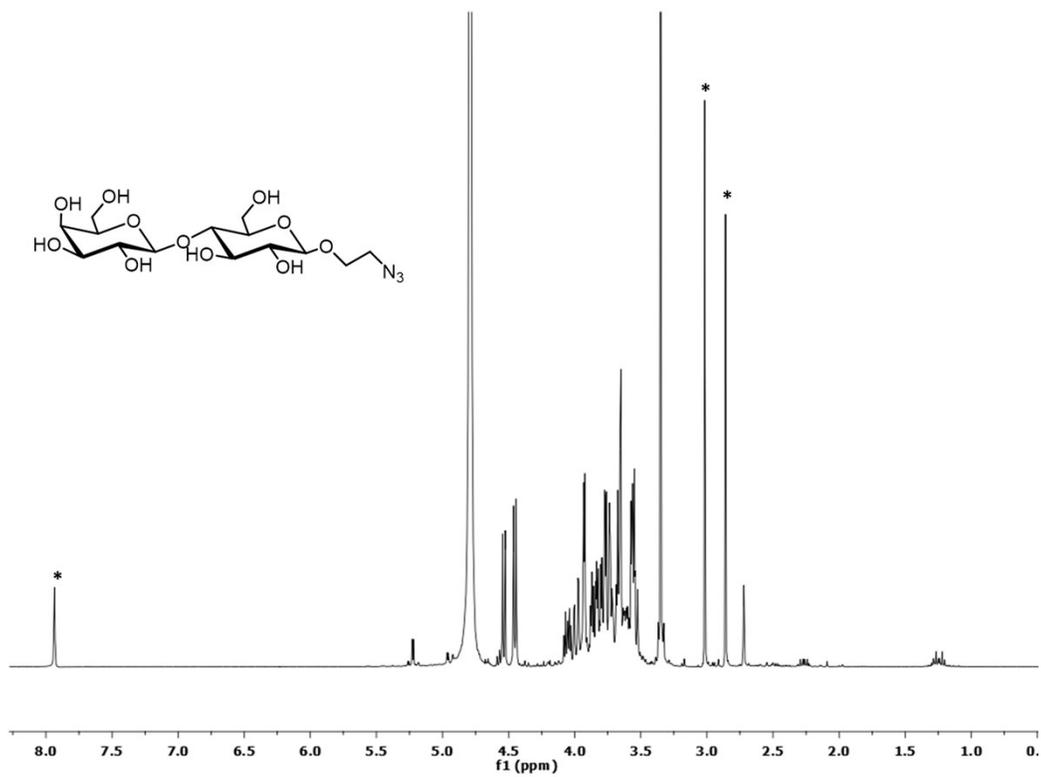
**Figure S23.**  $^1\text{H}$  NMR spectrum of 2'-azidoethyl lactose (**9e**) in  $\text{CD}_3\text{OD}$  (\* DMF).
