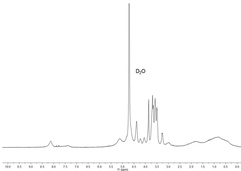
**Figure S38.** <sup>1</sup>H NMR spectrum of lactose linear homo-glycopolymer (**13e**) in D<sub>2</sub>O.
