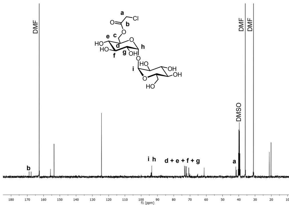
**Figure S26.**  $^{13}C$  NMR spectrum of the crude reaction mixture containing the desired 6-chloroacetyl trehalose (**6**), along this unreacted trehalose, and 6'-diesterified trehalose byproduct.
