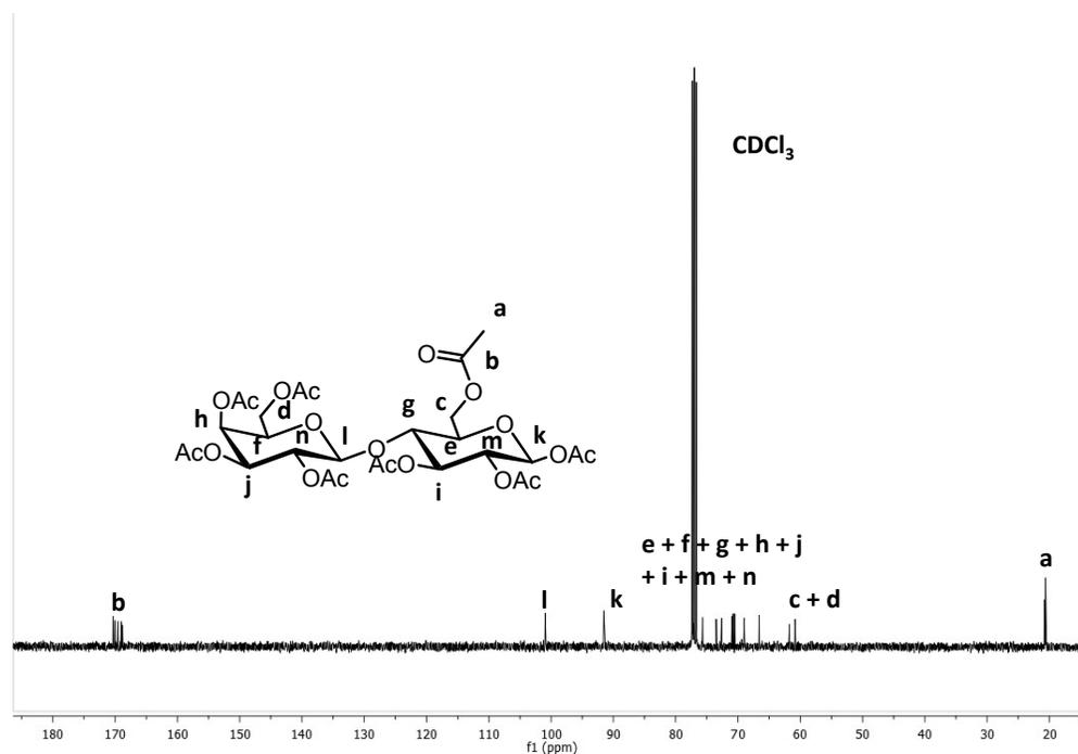
**Figure S18.**  $^{13}\text{C}$  NMR spectrum of lactose octaacetate (**3**) in  $\text{CDCl}_3$ . For clarity only one of the OAc groups is shown in its expanded structure.
