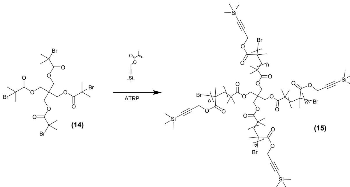
**Scheme S12.** Synthesis of 4-arm star TMS-protected poly (propargyl methacrylate) (**15**).
