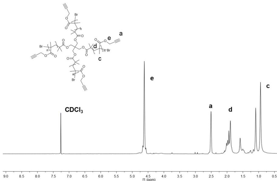
**Figure S33.**  $^1H$  NMR spectrum of star poly(propargyl methacrylate) (**16**) in  $CDCl_3$ .
