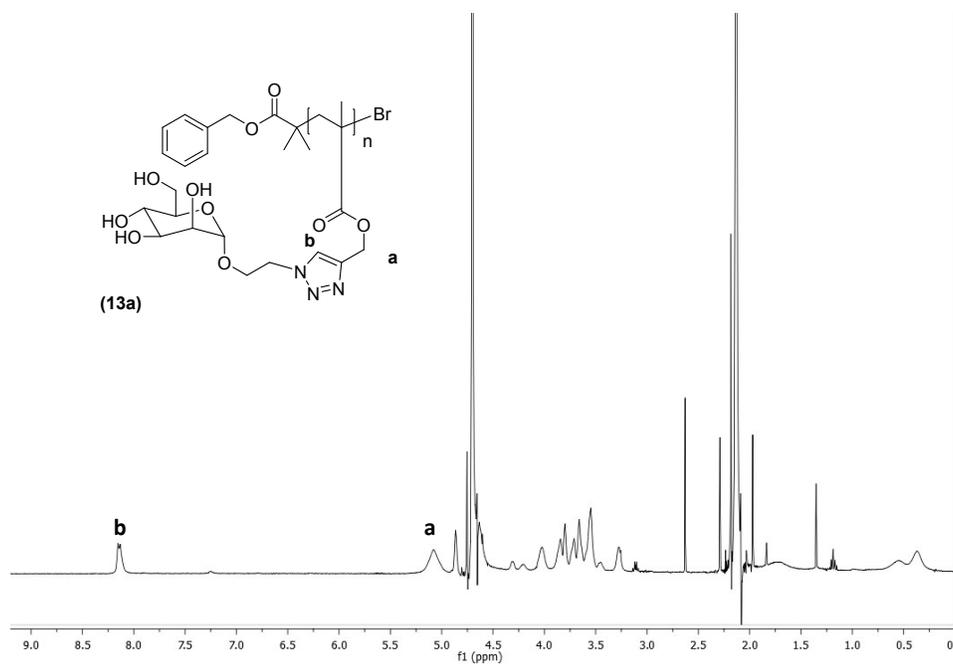
**Figure S34.** Representative spectrum of clicked glycopolymers:  $^1\text{H}$  NMR spectrum of mannosyl linear homo-glycopolymer (**13a**) in  $\text{D}_2\text{O}$ .
