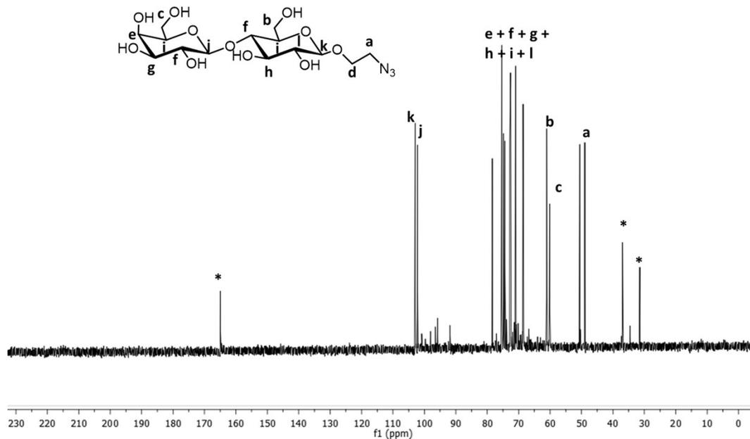
**Figure S24.**  $^{13}\text{C}$  NMR spectrum of 2'-azidoethyl lactose (**9e**) in  $\text{CD}_3\text{OD}$  (\* DMF).
