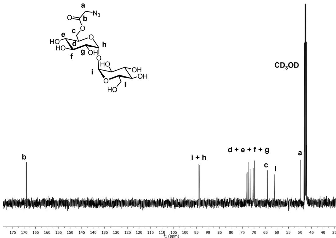
**Figure S28.** <sup>13</sup>C NMR spectrum of trehalose azide (**10f**) in CD<sub>3</sub>OD.
