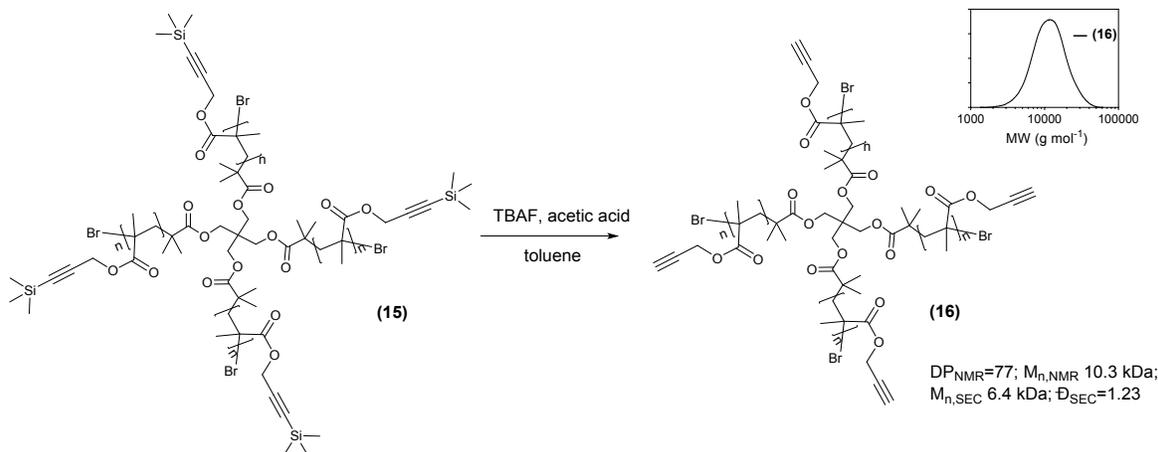
**Scheme S13.** Deprotection of TMS-protected star poly(propargyl methacrylate) (**15**) to give the star clickable scaffold (**16**) – inset:  $\text{SEC}_{\text{CHCl}_3}$  trace of (**16**).
