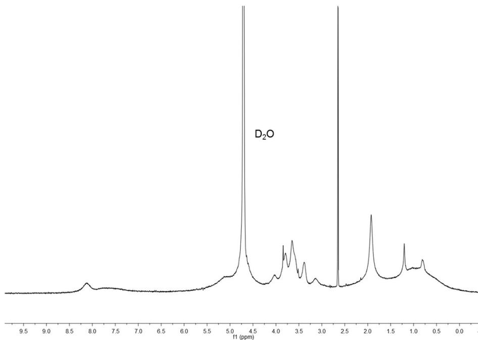
**Figure S37.** <sup>1</sup>H NMR spectrum of *N*-acetyl glucosamine linear homo-glycopolymer (**13d**) in D<sub>2</sub>O.
