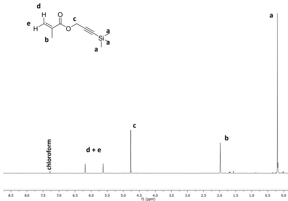
**Figure S29.** <sup>1</sup>H NMR spectrum of trimethylsilyl methacrylate monomer **(11)** in CDCl<sub>3</sub>.
