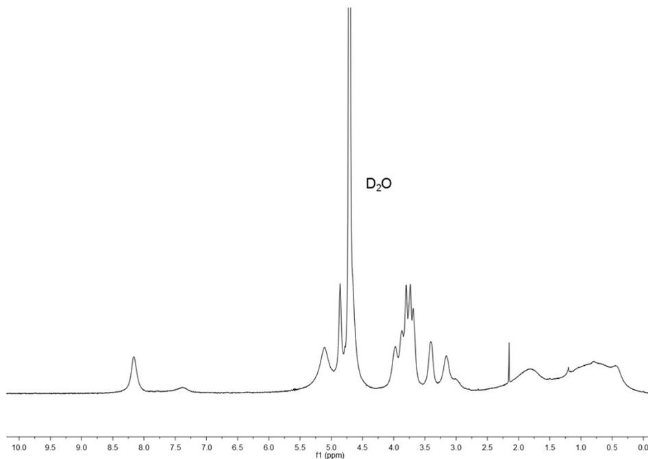
**Figure S36.** <sup>1</sup>H NMR spectrum of arabinose linear homo-glycopolymer (**13c**) in D<sub>2</sub>O.
