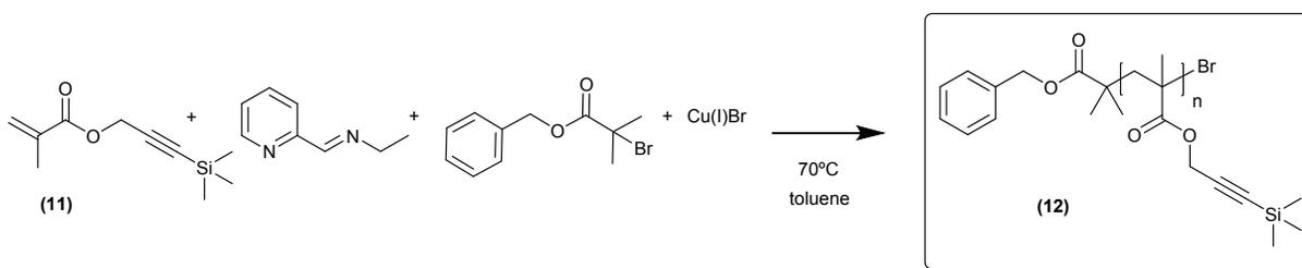
**Scheme S9.** Synthesis of linear TMS-protected poly(trimethylsilyl-propargyl methacrylate) (**12**).
