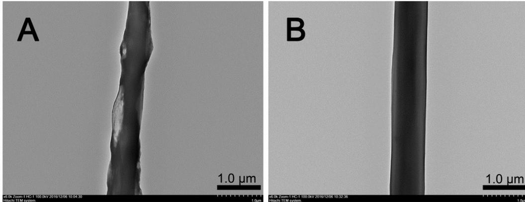
**Fig. S3** TEM images of PCL-H (A) and PCL (B) membranes.
