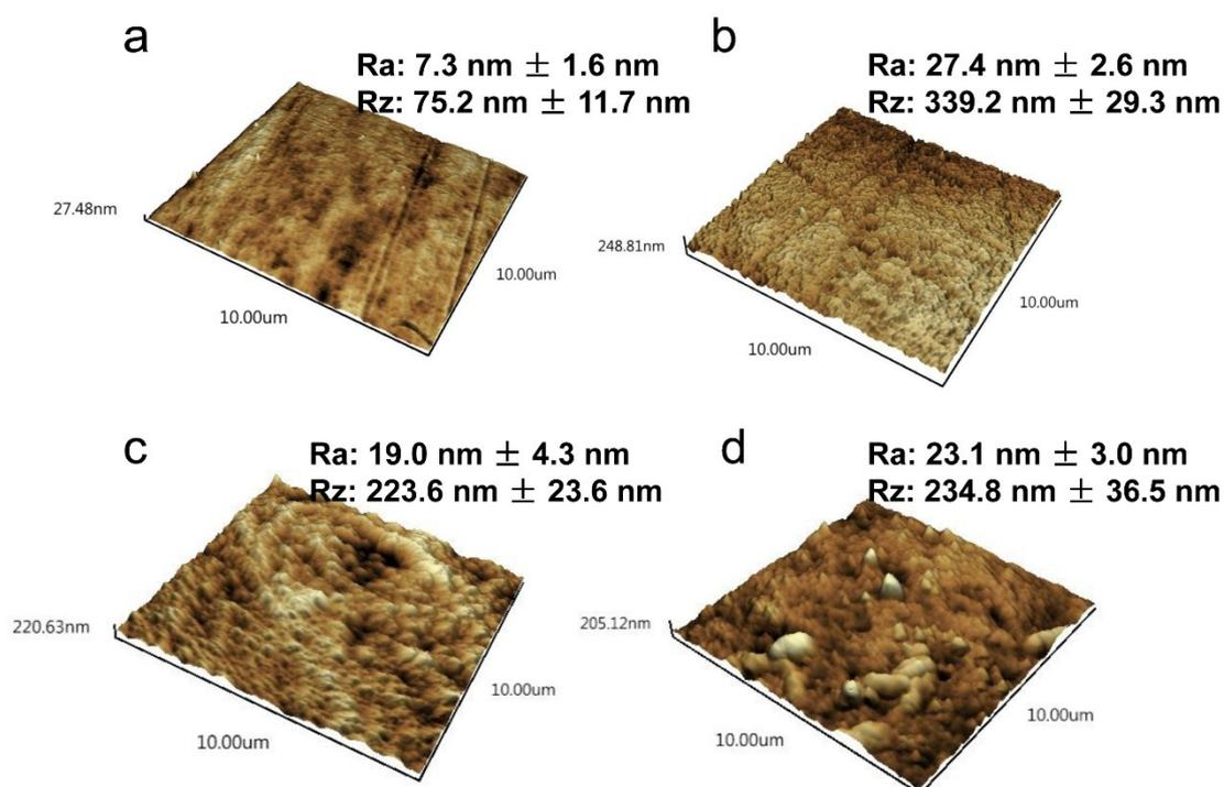
**Figure S8.** AFM images of (a) intact enamel surface, (b) acid-etched enamel surface, (c) Peptide-7 treated enamel surface, and (d) NaF treated enamel surface after 8 days of mineralization. Ra indicates the mean roughness (nm) and Rz indicates the maximum height (nm) of the tested surface.
