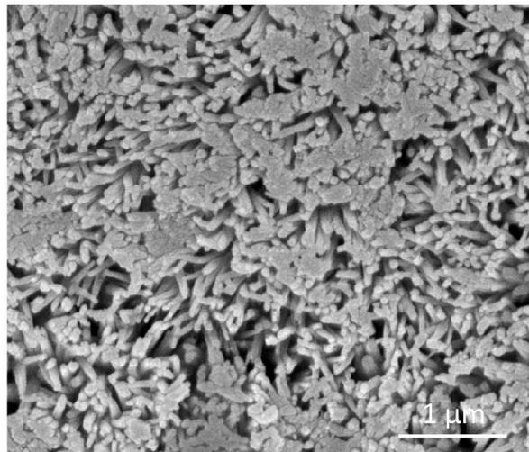
**Figure S7.** SEM image of the surface morphology of NaF treated enamel, showing rod-like microstructures on the enamel surface (Magnification ratio is 25000).
