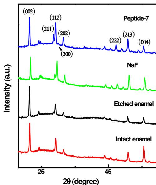
**Figure S9.** XRD patterns of the intact tooth enamel, acid-etched enamel, Peptide-7 treated enamel, and NaF treated enamel after 8 days of mineralization.
