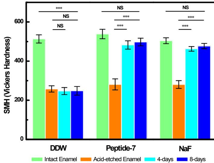
**Figure S10.** The surface micro-hardness (Vickers hardness) of DDW, Peptide-7, and NaF treated enameles after being soaked in artificial saliva for 4 days and 8 days, compared with the micro-hardness values of the original and acid-etched tooth enamel surfaces. \*\*\*,  $p < 0.005$ ; NS, no significant difference
