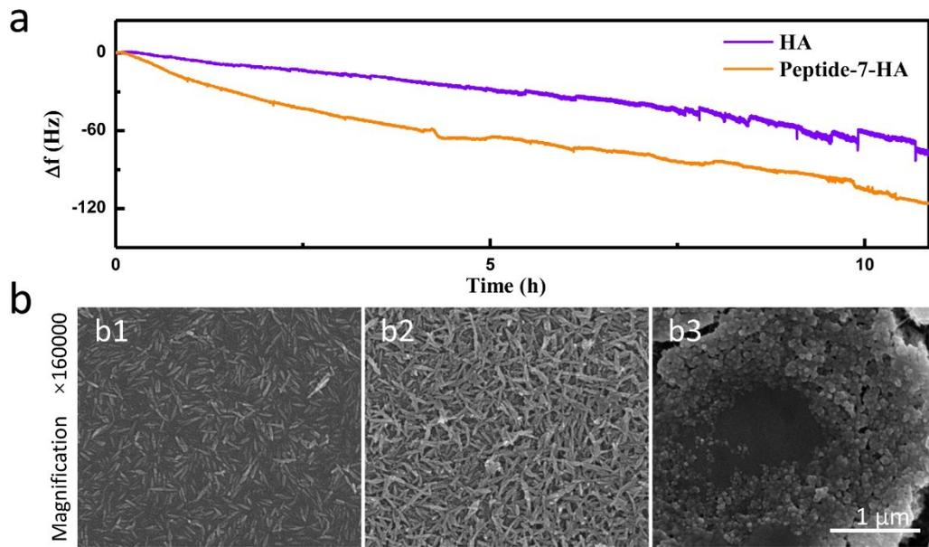
**Figure S6.** (a) QCM-D results of the mineralization ability of Peptide-7 after adsorption on HA chips. The declines in frequency were 68.73 Hz and 115.41 Hz in the control group and experimental group, respectively, over a period of 12 h. (b) SEM images of HA chips before (b1) and after incubation in flowing artificial saliva for 12 h (b2 and b3). The control group (b2) used bare HA chips and the experimental group (b3) used Peptide-7 coated HA chips (pH = 7.5).
