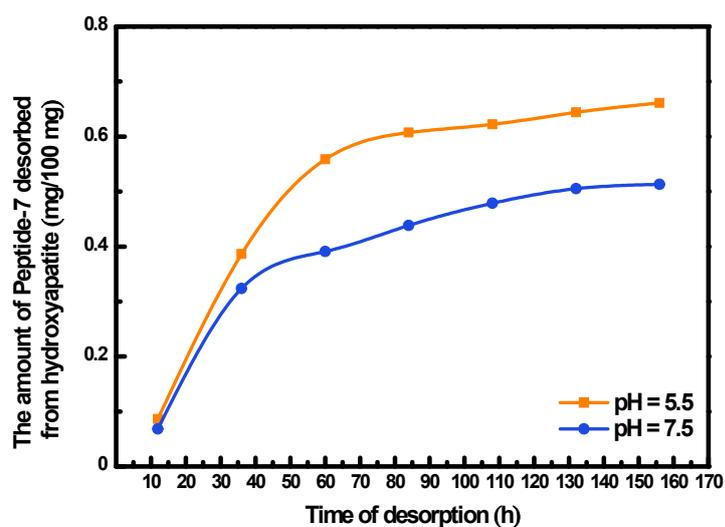
**Figure S4.** Desorption isotherm curves of Peptide-7 from HA powder. The orange line represents acidic condition (pH = 5.5) and the blue line represents neutral condition (pH = 7.5).
