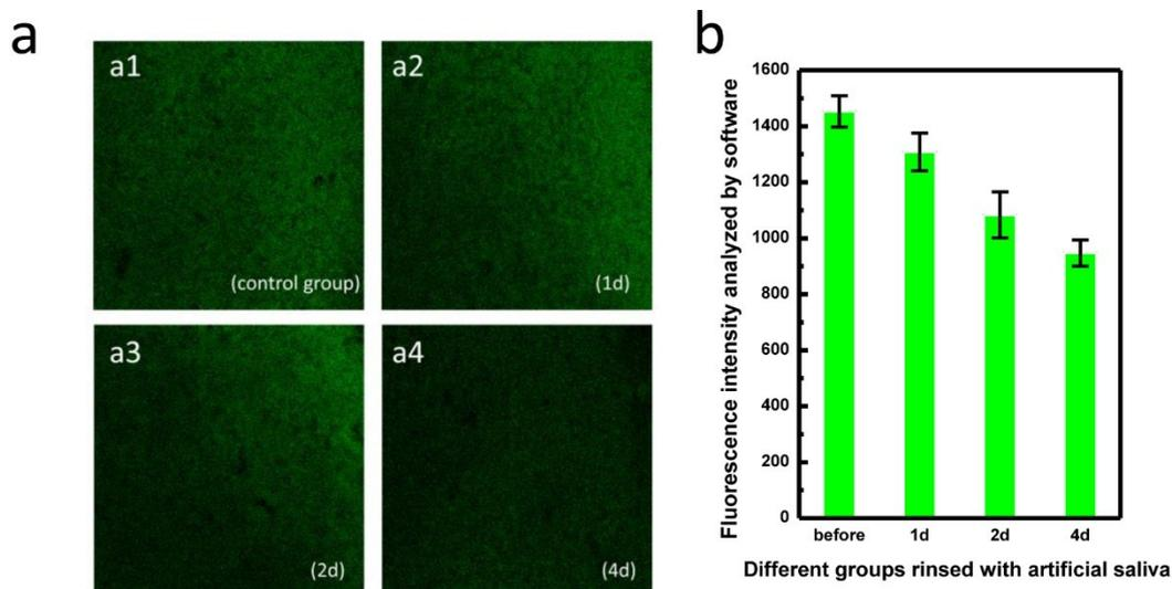
**Figure S3.** (a) CLSM fluorescence images of HA disk surfaces. (a) a1, before washout; a2, after one-day washout; a3, after two-day washout; a4, after four-day washout. (b) The fluorescence intensity was calculated by the software to estimate the amount of Peptide-7-FITC retained on HA surfaces after being washed for different number of days. The histogram shows the fluorescence intensity descending process.
