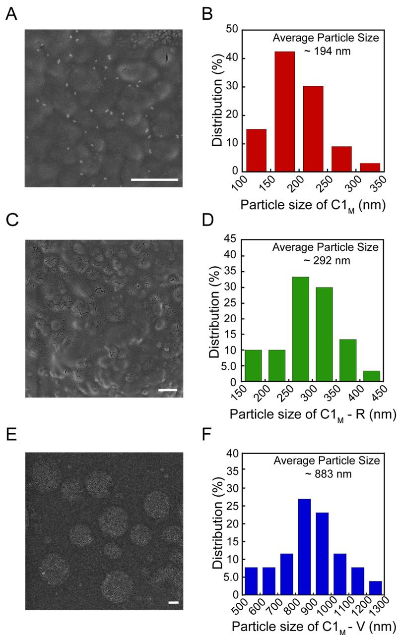
**Figure S9.** (A, C and E) FESEM image  $C1_M$ ,  $C1_M-R$  and  $C1_M-V$ . Scale bar for the image is 500 nm. (B, D and F) Particle size distribution of  $C1_M$ ,  $C1_M-R$  and  $C1_M-V$  determined by ImageJ software.
