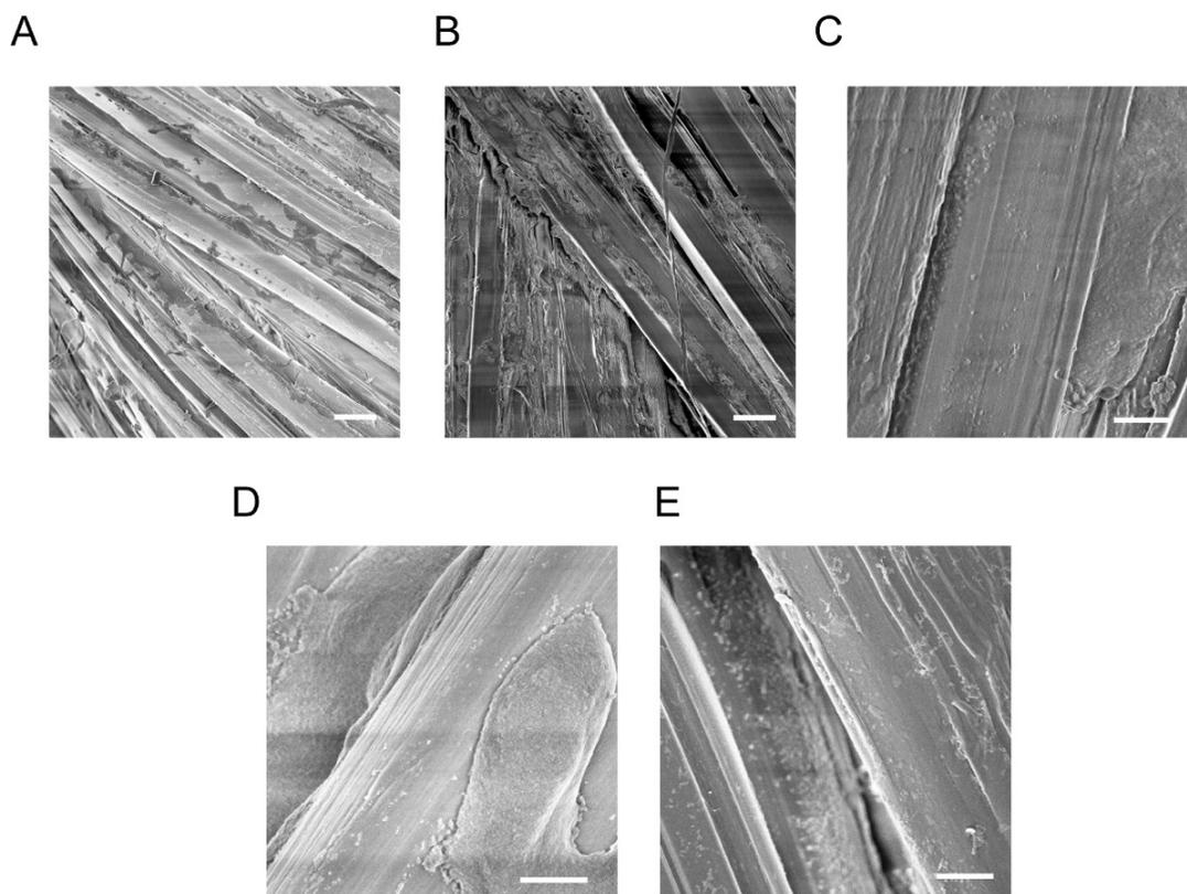
**Figure S13.** FESEM images of (A) Non-coated silk suture and silk sutures coated with (B) C1, (C) C1<sub>M</sub>, (D) C1<sub>M</sub>-R and (E) C1<sub>M</sub>-V. Scale bar for the images is 2.0  $\mu\text{m}$ .
