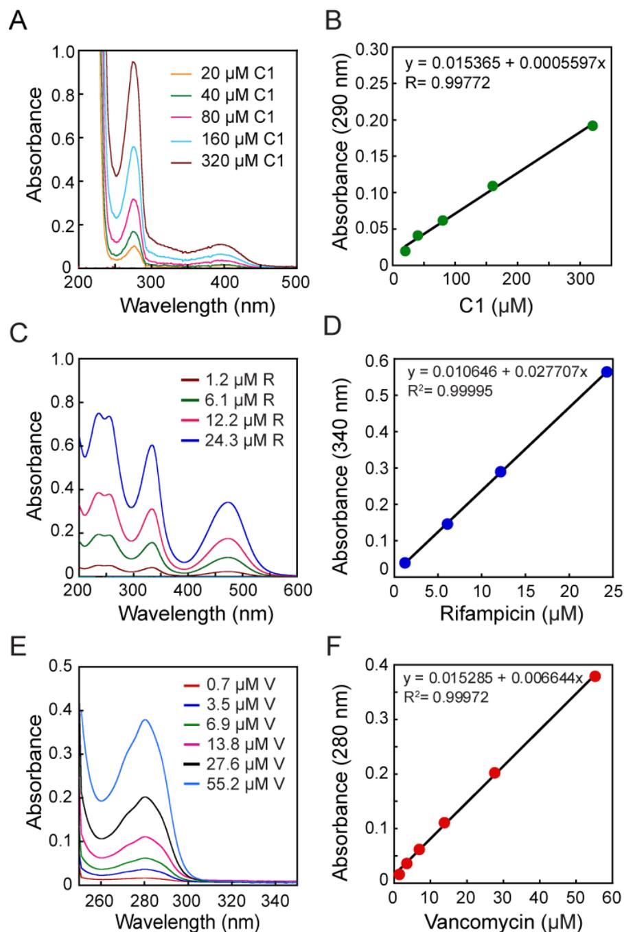
**Figure S10.** UV-visible absorption spectra of varying concentrations of (A) C1, (C) rifampicin (R) and (E) vancomycin (V). Calibration plots for (B) C1, (D) rifampicin and (F) vancomycin generated by plotting the respective absorbance maxima against concentration.
