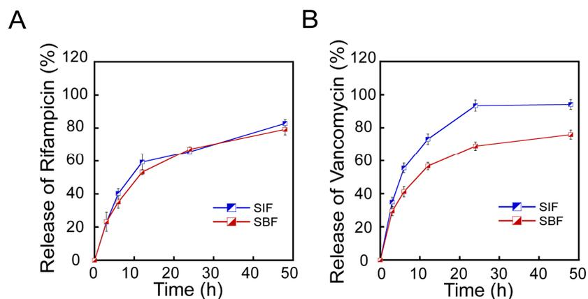
**Figure S11.** *In vitro* release kinetics of (A) rifampicin and (B) vancomycin from loaded C1<sub>M</sub> incubated in simulated body fluid (SBF) (pH 7.4) and simulated intestinal fluid (SIF) (pH 8.0).
