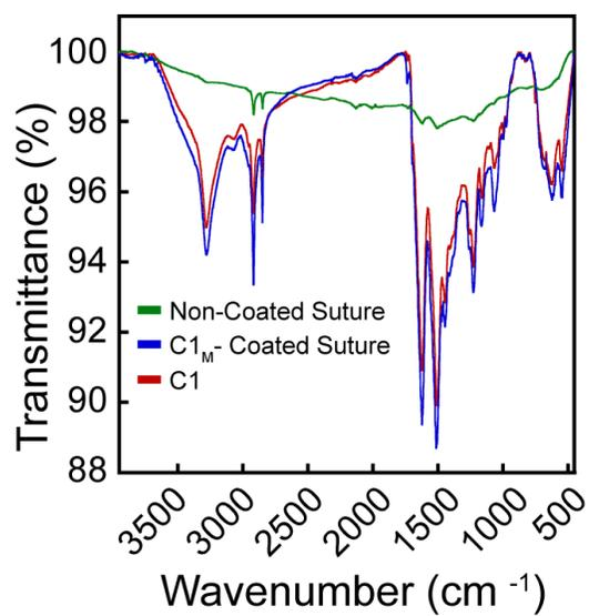
**Figure S14.** ATR-FTIR of non-coated silk suture, C1<sub>M</sub> coated silk suture and C1 alone.
